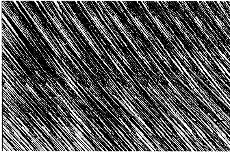
Figure 4.5: Final workpiece surface: normal grits move along the straight line
