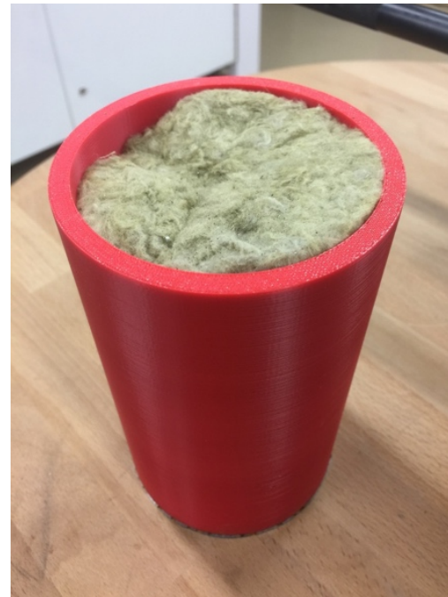
Figure 23: Test sample of perforated wall
