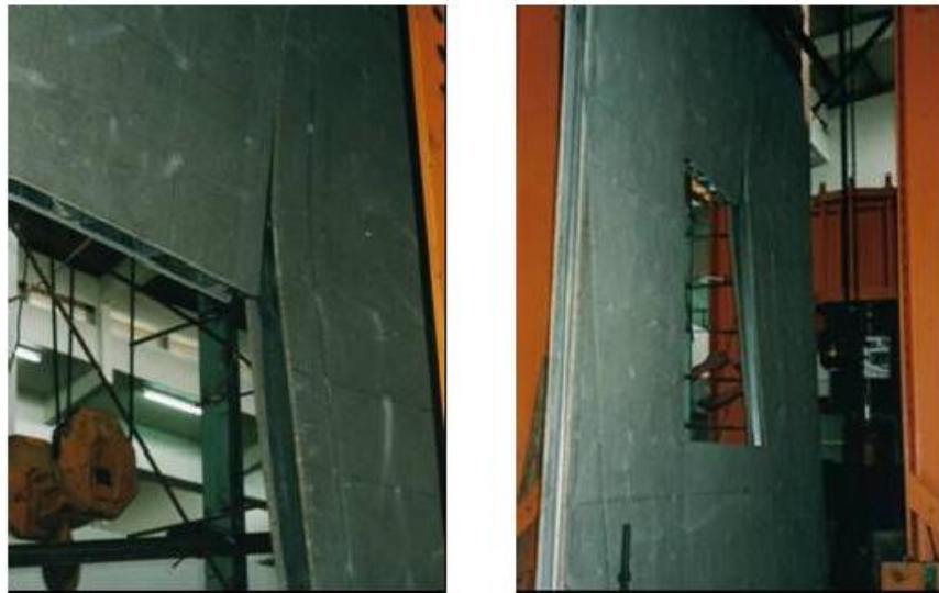
Figure 2.17 Failure at the corner of opening during experiment (Hamzah & Badaruzzaman, 2009)
