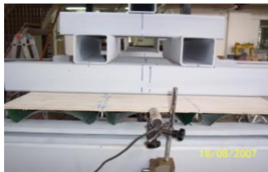
Figure 2.13 Buckling of lower flange of the profiled steel sheet (Awang and Badaruzzaman, 2009)
