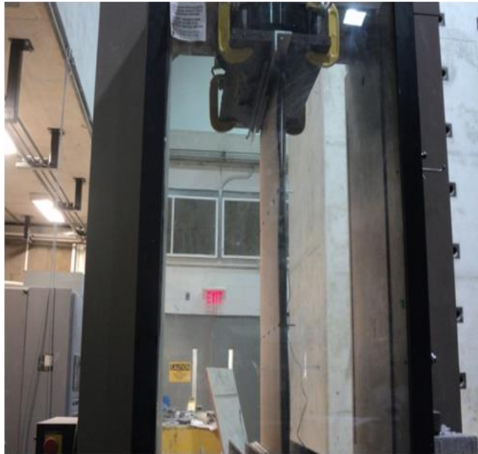
Figure 3.3 MTS test set-up for PSSDB wall panel subjected to axial loading
