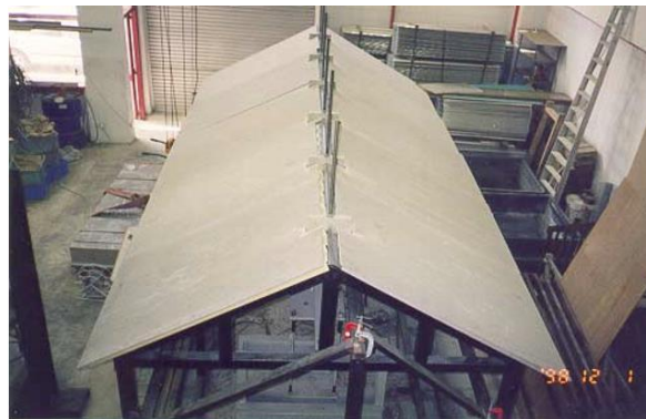
Figure 2.10 Complete model of PSSDB folded roof plate tested in the laboratory by Ahmed et al. (2000)
