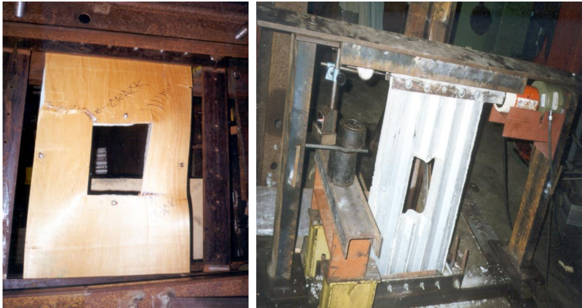
Figure 4.4 (b) Experimental set-up for A1-B1 series wall panels subjected to horizontal shear loading
