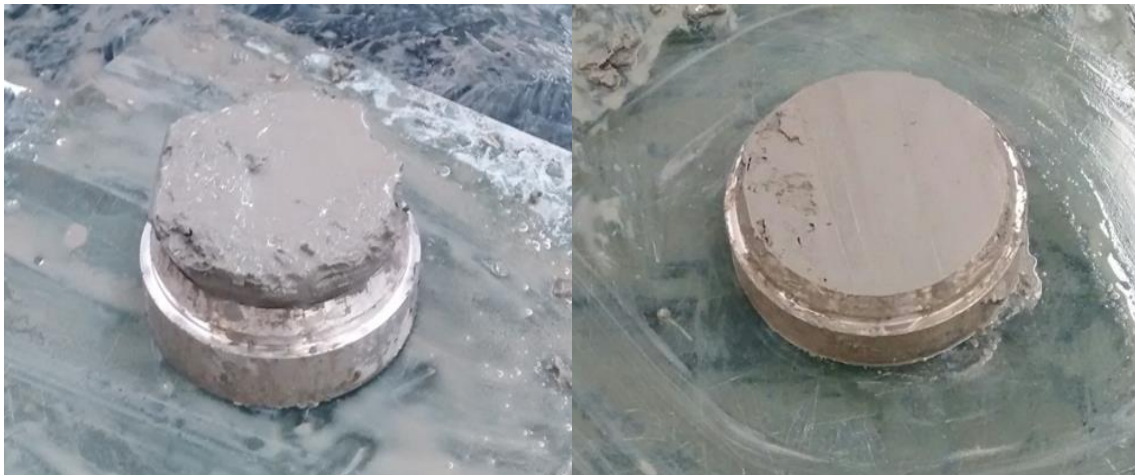
Figure 4.9 Trimming of Champlain Sea clay samples for CRS tests
