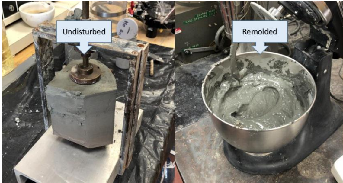
Figure 4.5 The loss of shear strength in Champlain Sea clay due to remolding
