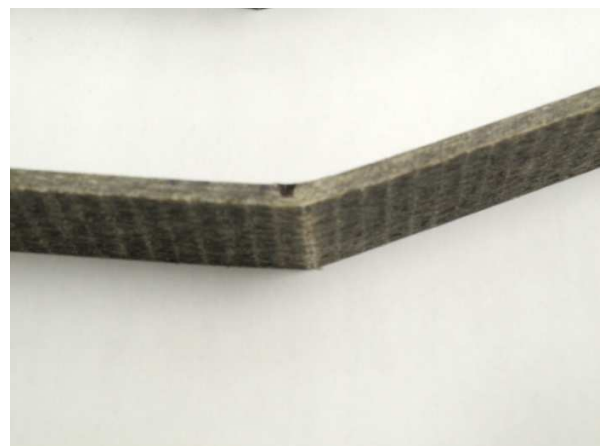
Figure 60: Simple outer-surface failure under flexural load - close view
