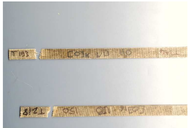
Figure 58: Failure of samples under tensile load - horizontal view
