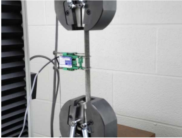
Figure 10: Tensile test with extensometer - close view
