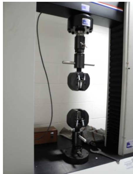
Figure 9: A view of the grips used for tensile testing
