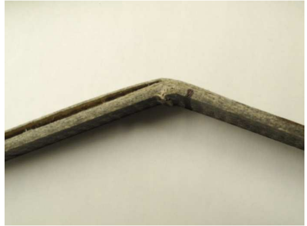
Figure 62: Complex outer-surface tensional failure, inner-surface compressive failure, and delamination under flexural load
