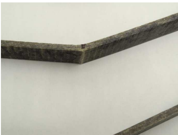
Figure 59: Simple outer-surface failure under flexural load
