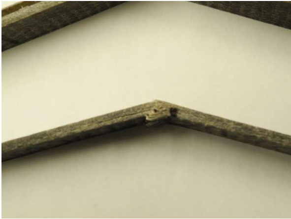
Figure 61: Combined outer-surface tensional failure and inner-surface compressive failure under flexural load
