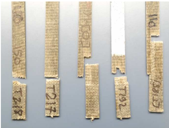
Figure 57: Failure of samples under tensile load - vertical view
