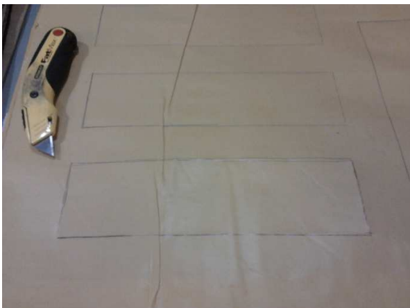
Figure 1: Mapping and cutting of prepreg composite layers
