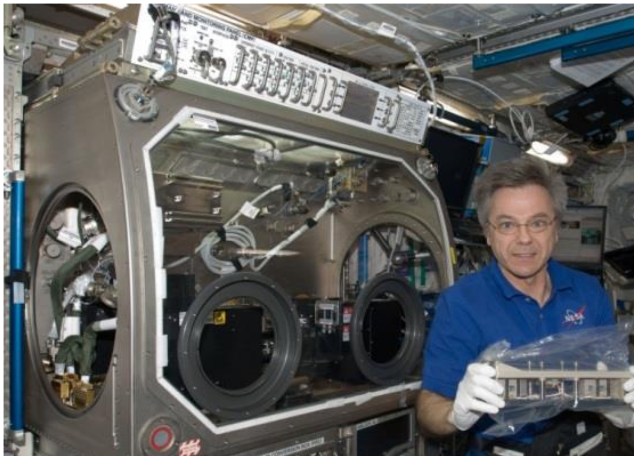
Figure 8-2: Glovebox and CSA astronaut Thirsk, onboard ISS before installing SODI array inside that box
