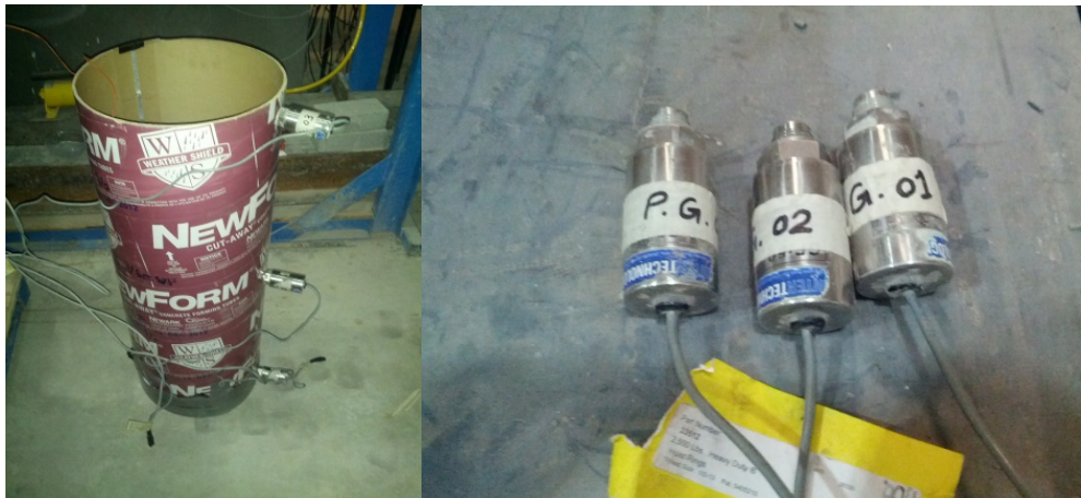
Figure 3.13: Pressure transducers installed in the Weather Shield tube
