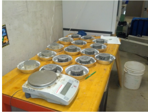
Figure 3.24: Experimental setup for sorptivity test
