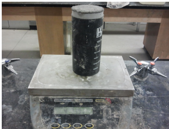
Figure 3.10: Fresh density monitoring setup
