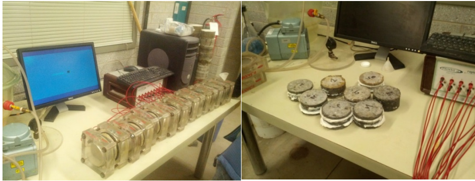
Figure 3.26: Experimental Setup of chloride penetration test
