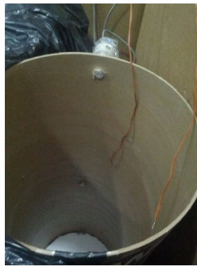
Figure 3.14: Temperature thermocouple introduced at core and at surface of Weather Shield tube for all concretes.
