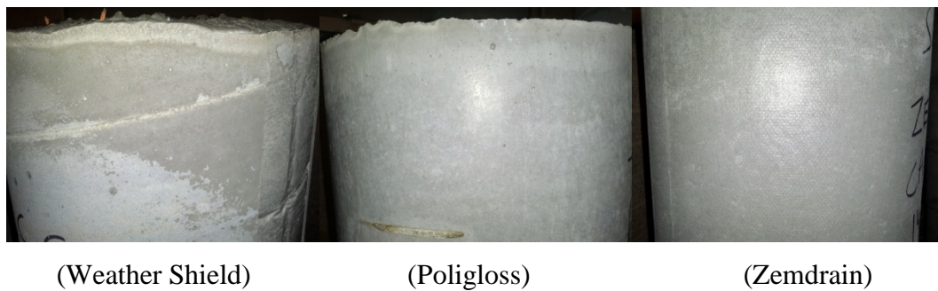
Figure 4.8: Concrete finish after removing formwork for MS-S10 SCC
