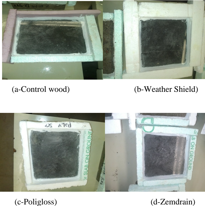
Figure 4.30: Condition of SCC concrete Surface After 50 Cycle
