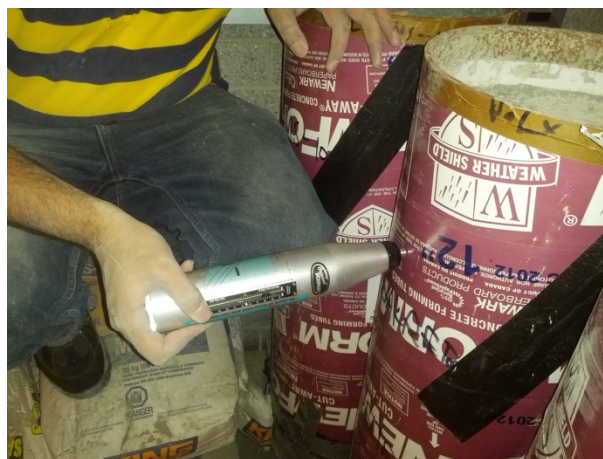
Figure 3.16: Schmidt hammer test on a typical tube
