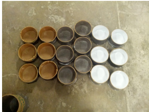
Figure 3.25: Chloride penetration molds for Weather Shield, Poligloss and Zemdren
