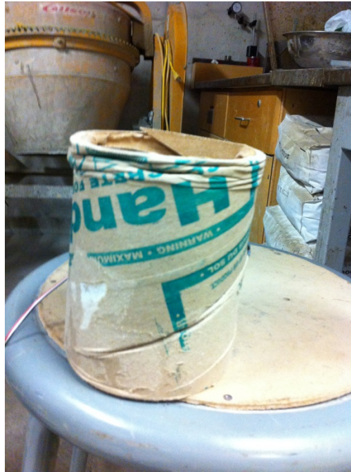
Figure 3.34: Weather Shield forming tube after compressive test
