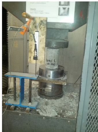
Figure 3.19: Typical experimental setup of Compressive testing machine.
