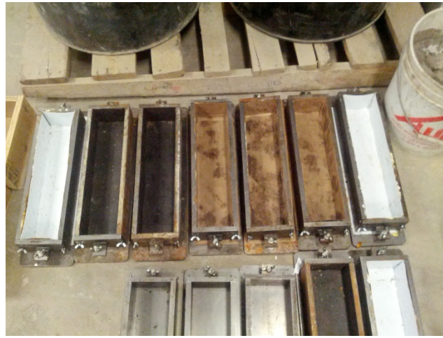
Figure 3.27: Freeze Thaw molds for Weather Shield, Poligloss and Zemdrain
