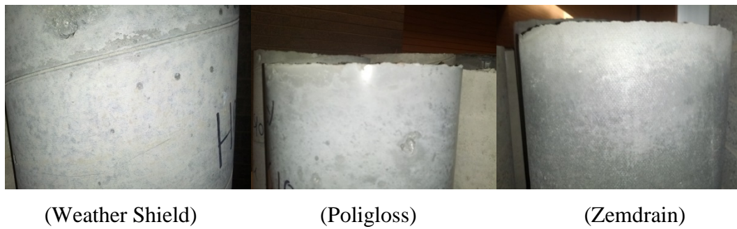
Figure 4.7: Concrete finish after removing formwork for HP-S10
