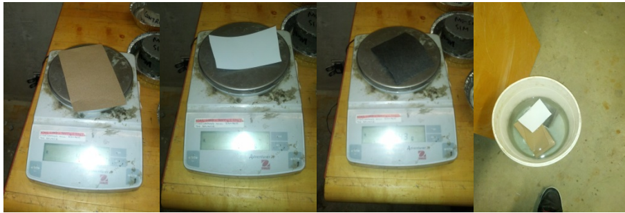
Figure 3.17: Setup for water absorption of formwork liners.
