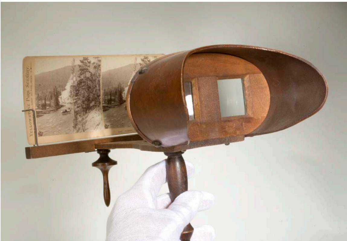
fig. 2: Holmes Stereoscope with a folding handle. George Eastman House: International
