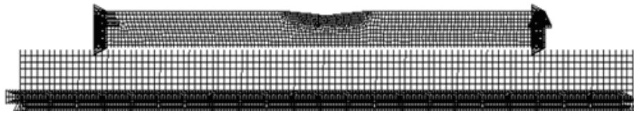
Figure 5.14 Mesh of a PDMS sample 5 cm long x 4 mm thick constrained at the ends.
