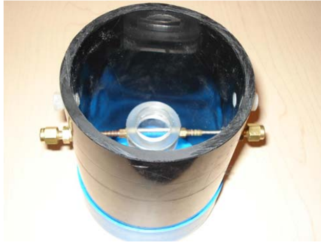
Figure 3-2 In this custom-made container for the attenuation measurements, ultrasound beam was reflected off a quartz plate, located at the focus of the transducer.
