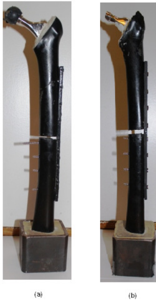
Figure 3.8 Two conditions of testing (a) Injured femur with titanium bone plate; (b) Injured femur with carbon/epoxy bone plate
