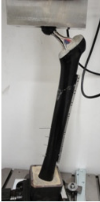
Figure 3.9 Experimental set-up for axial compression test of femur with 7° inclination
