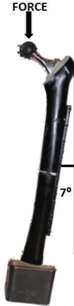
Figure 3.1 Axial loading of femur at 7 degrees of adduction
