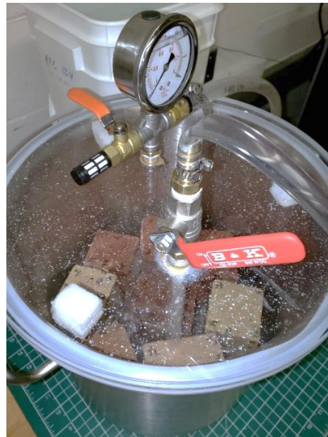
FIGURE 4-9: ONCE THE RIGHT LEVEL OF VACUUM PRESSURE WAS REACHED (I.E. 0ATM OR -30INHG), THE VALVE CONNECTING THE RESERVOIR TO THE DESICCATOR VESSEL WAS OPEN ALLOWING IT BE FILLED WITH DISTILLED WATER
