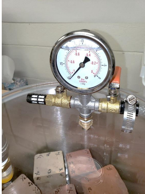
FIGURE 4-8: THE BRICK SAMPLES WERE SUBJECTED TO A VACUUM INSIDE THE VESSEL, WHEREBY THE GAUGE HERE INDICATED THE PRESSURE INSIDE TO BE -1ATM (~30 INHG).
