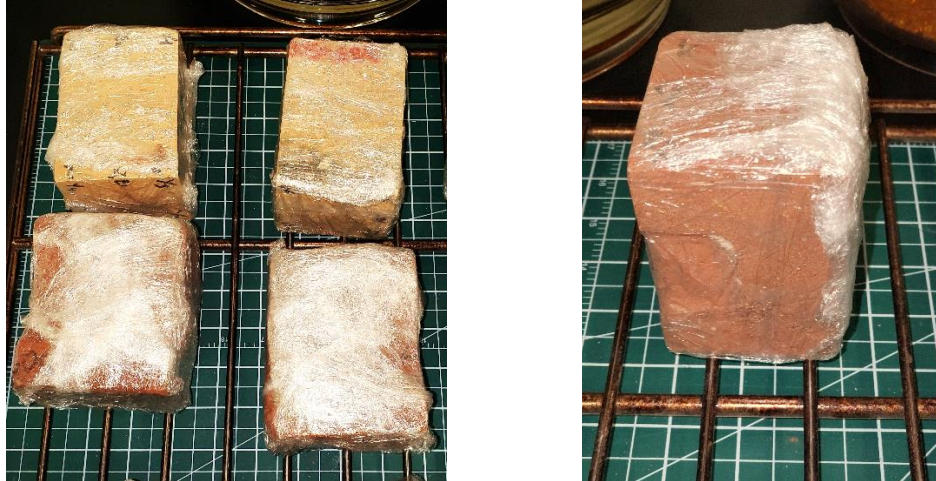
FIGURE 4-12: THE BRICK SAMPLES HAVE BEEN TIGHTLY WRAPPED IN TWO LAYERS OF CLING FILM
