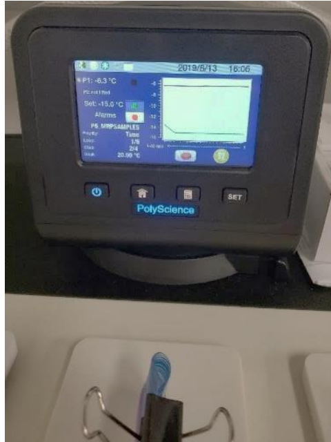
FIGURE 4-15: THE PROGRAM FOR THE FREEZE-THAW CYCLES IS BEING RUN AS SEEN ON THE CONTROLLER'S SCREEN.
