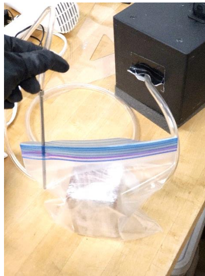
FIGURE 4-13: AIR WAS REMOVED FROM INSIDE THE ZIPLOCK BAG USING A MODIFIED ‘VACUUM CLEANER’.
