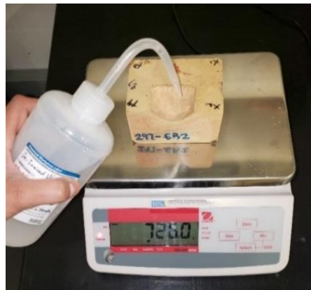
FIGURE 4-10: A DROPPER WAS USED TO APPLY DISTILLED WATER ON THE BRICK SAMPLE, ALL THE WHILE METICULOUSLY MONITORING THE CHANGE IN MASS
