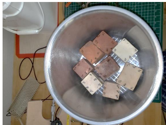
FIGURE 4-7: THE TEST SAMPLES WERE PLACED ON A LEVELLING RACK INSIDE THE DESICCATOR VESSEL. THEY WERE ARRANGED IN AN ORDER TO ENSURE THAT ALL OF THEM COULD BE VACUUM SATURATED AT THE SAME TIME.
