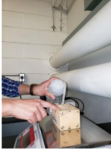
FIGURE 4-11: THE TECHNIQUE OF REAPPLYING MOISTURE SUCH THAT IT IS EVENLY DISTRIBUTED IN THE BRICK SPECIMEN
