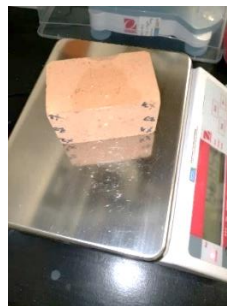
FIGURE 7-3: THE SURFACE OF THIS BRICK SAMPLE IS READILY ABSORBING MOISTURE
