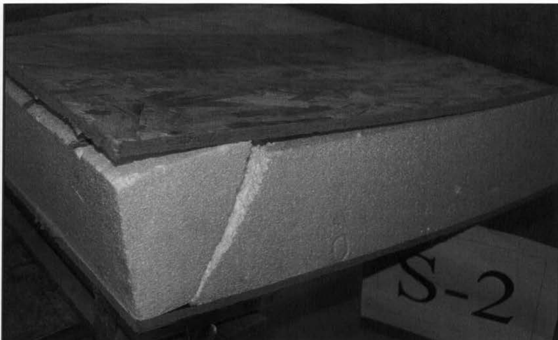
Figure 4.17 Close-up view of the diagonal shear crack in the foam at support at the other free edge of specimen S-2
