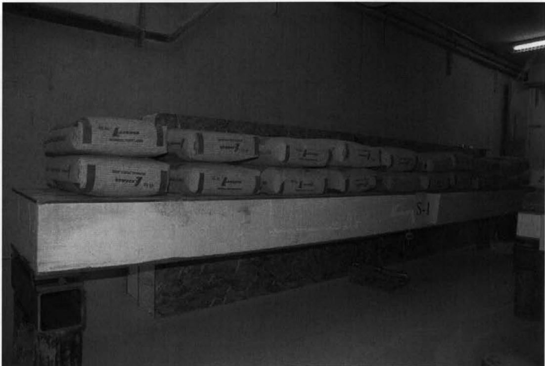
Fig. 3.20 View of dead and live load over panel S-4
