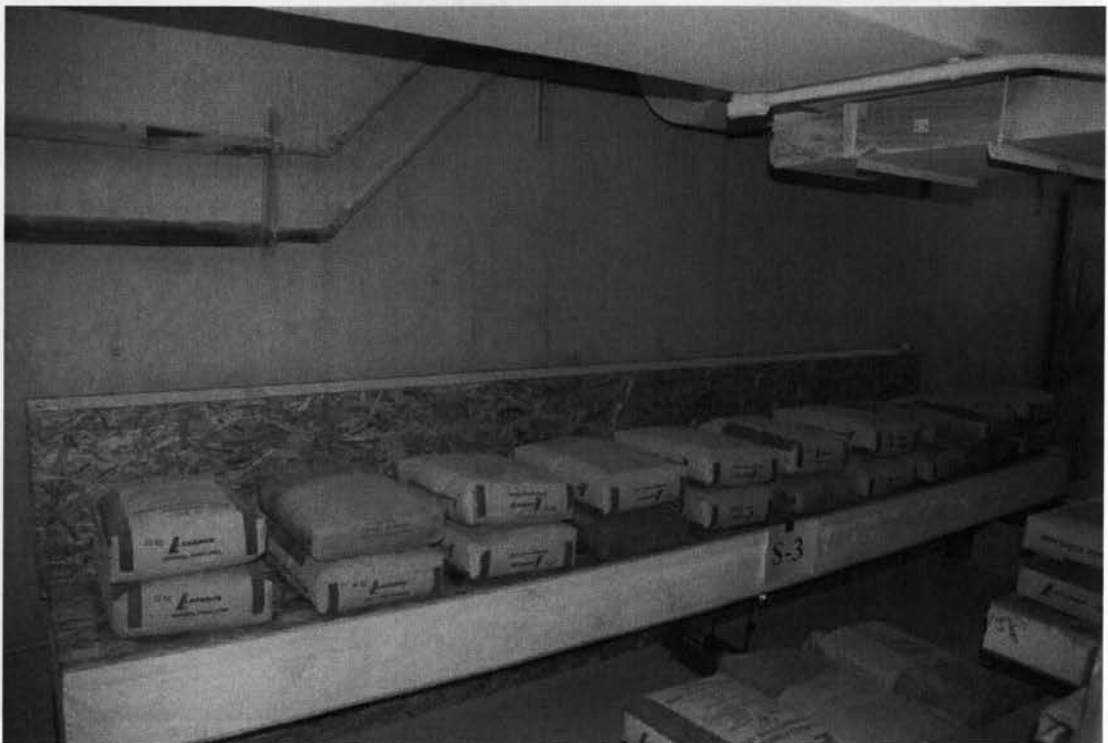
Fig. 3.26 View of dead and live load over panel S-6
