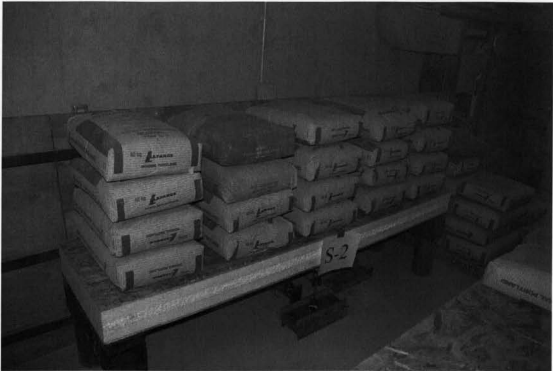
Fig. 3.15 View of double dead and live load over panel S-2
