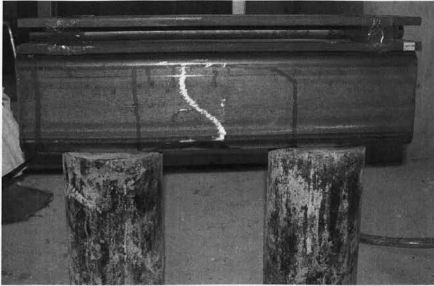
Figure 3.8 Typical support system for creep test
