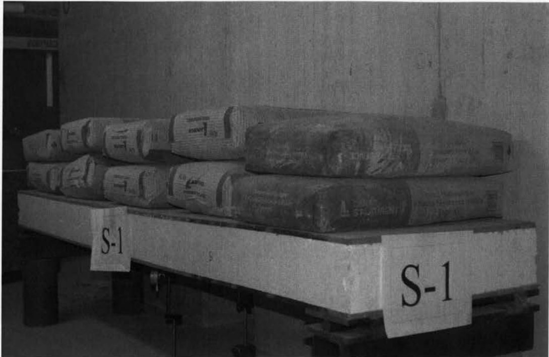
Figure 3.29 View of panels S-1 during long-term creep test
