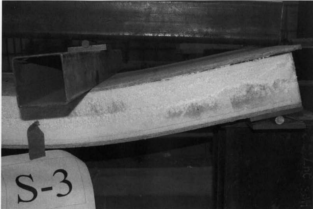
Figure 4.21 Close-up view of the horizontal shear failure between OSB top facing and foam core between support and quarter point of specimen S-3
