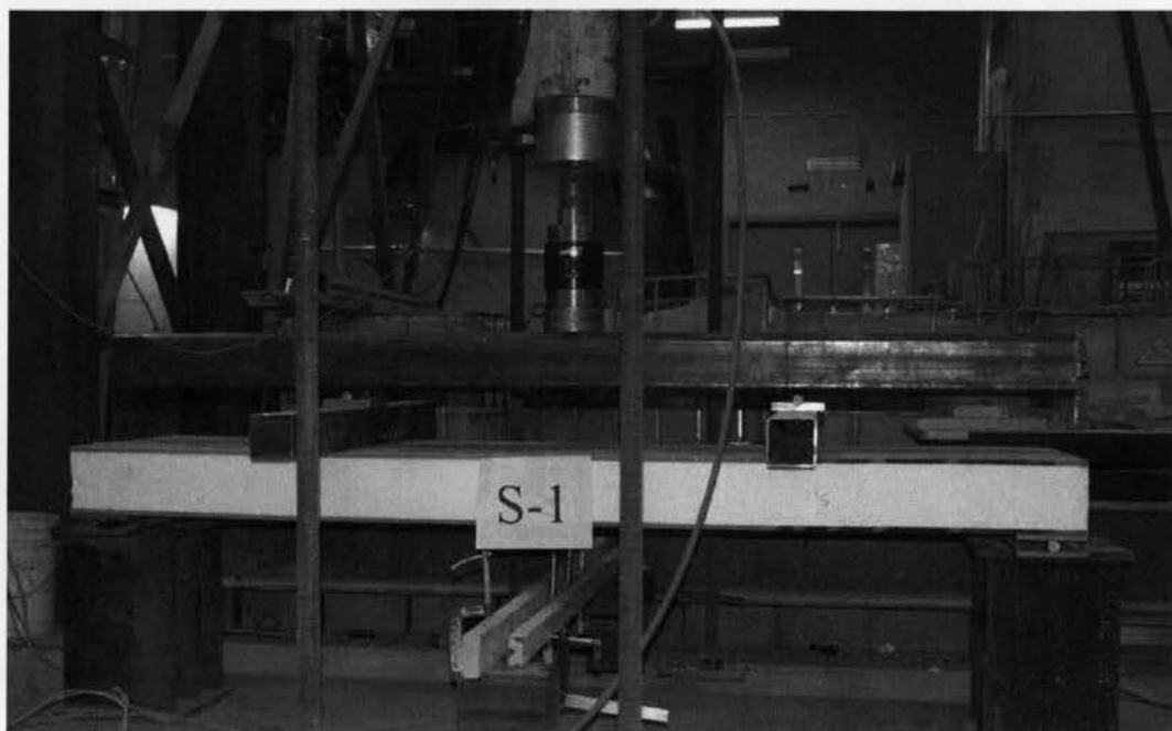
Figure 3.34 View of specimen S-1 before flexural load testing
