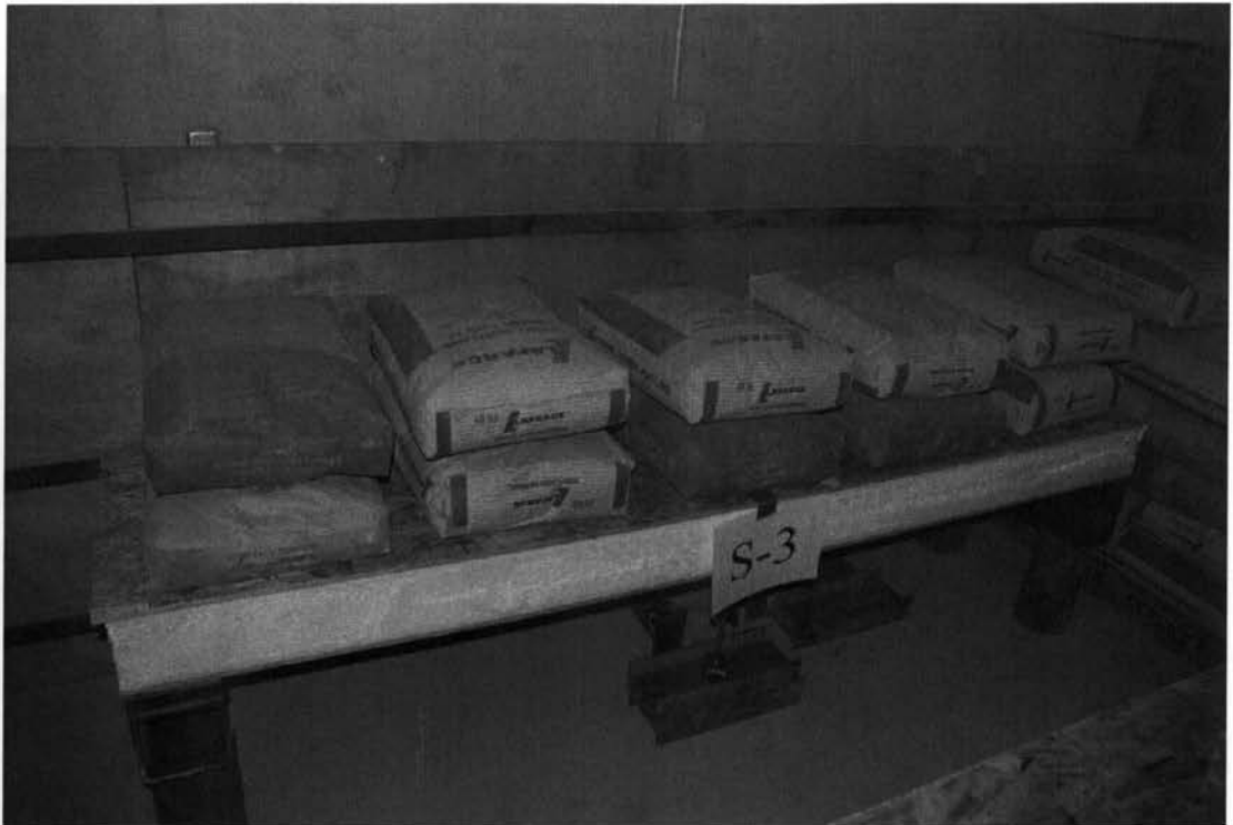
Fig. 3.17 View of dead and live load over panel S-3
