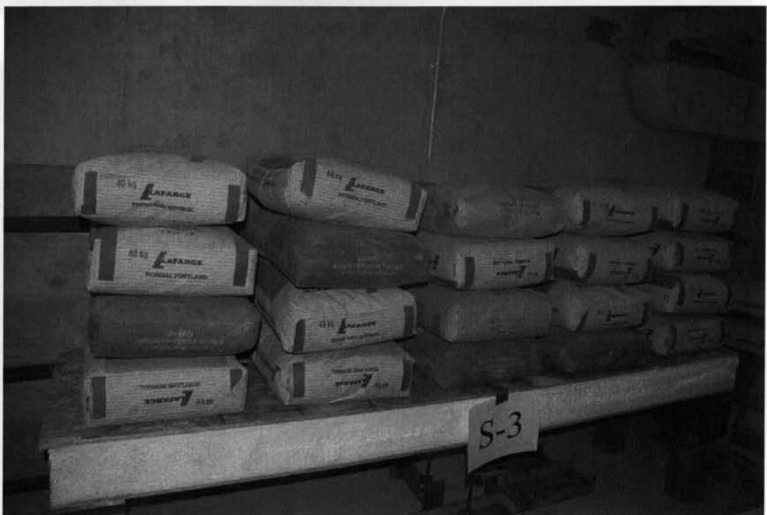
Fig. 3.18 View of double dead and live load over panel S-3
