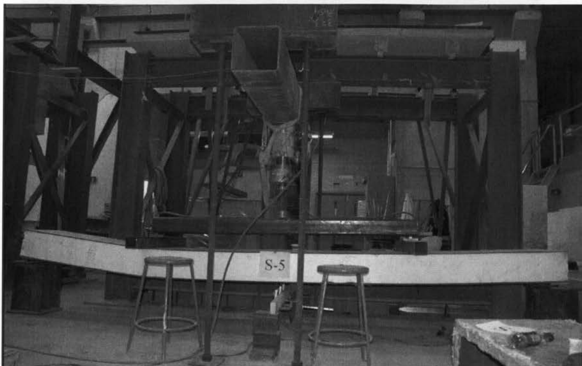
Figure 4.29 View of panel S-5 after failure
