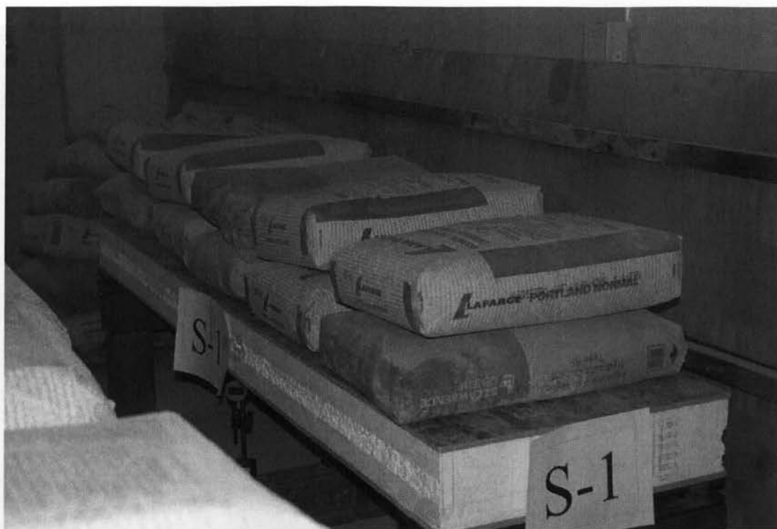
Fig. 3.11 View of dead and live load over panel S-1
