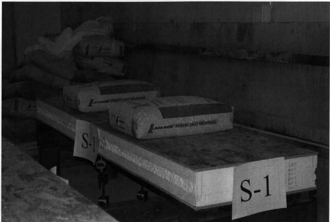
Fig. 3.10 View of dead load over panel S-1
