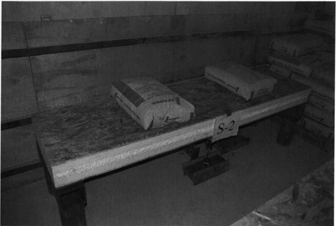
Fig. 3.13 View of dead load over panel S-2
