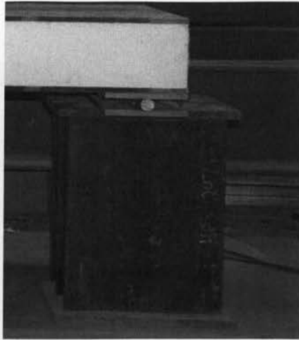
Figure 3.35 Enlarged view of the roller support of the tested panels
