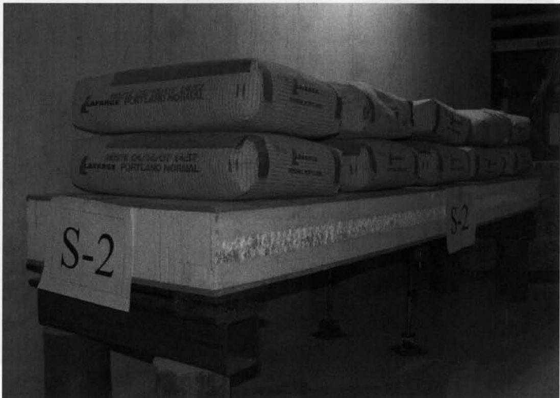
Figure 3.30 View of panels S-2 during long-term creep test
