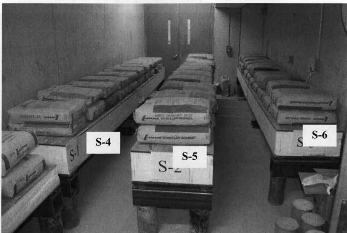
3.32 Views of panels S-4, S-5 and S-6 during long-term creep test
