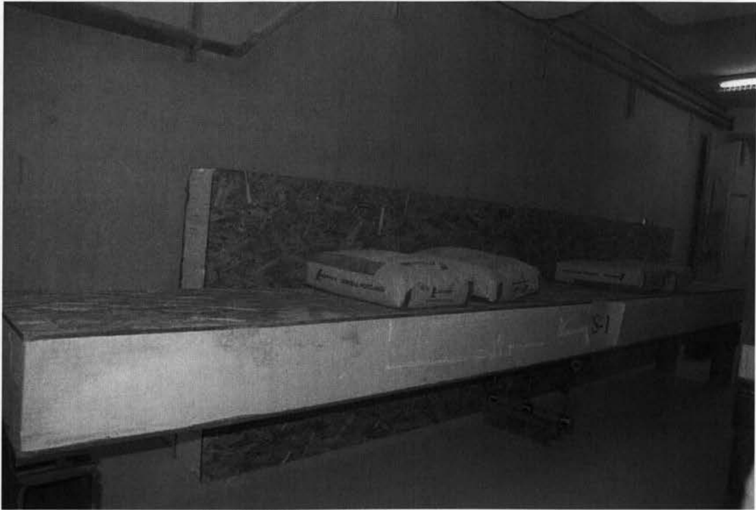
Fig. 3.19 View of dead load over panel S-4
