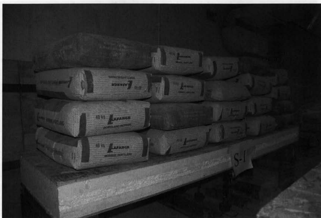
Fig. 3.12 View of double dead and live load over panel S-1
