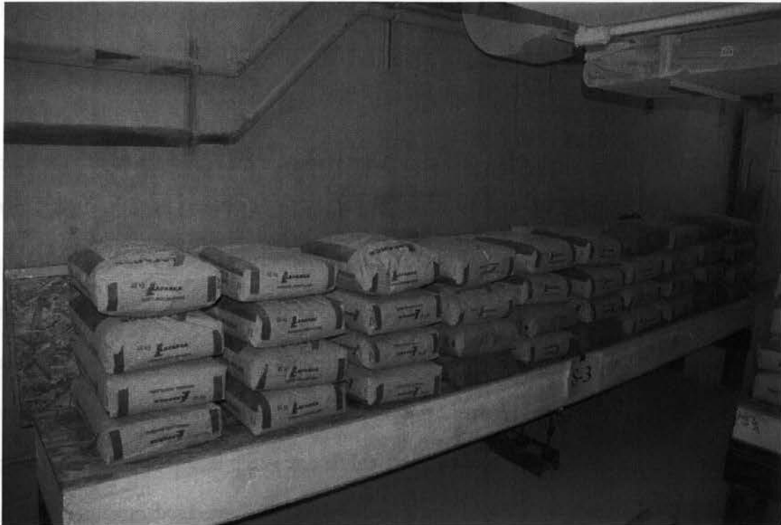
Fig. 3.27 View of double dead and live load over panel S-6
