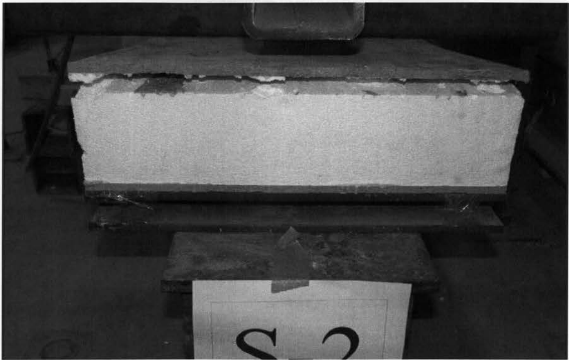
Figure 4.16 Close-up view of foam-OSB splitting over the support of specimen S-2 at failure
