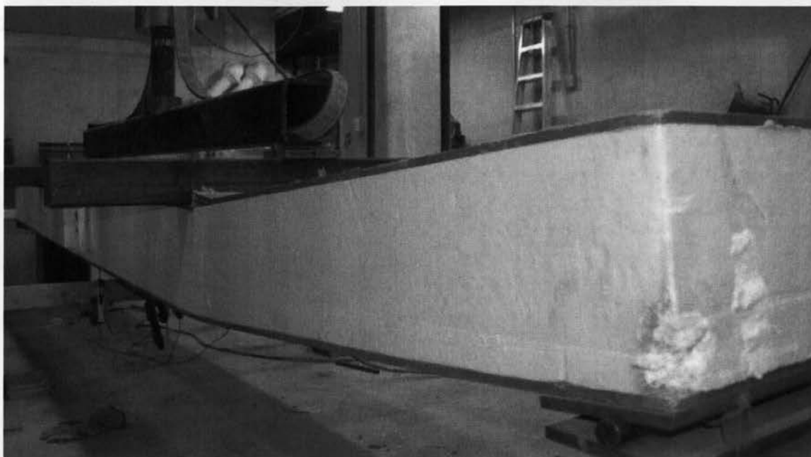
Figure 4.26 View of panel S-4 after failure showing deflected shape and OSB top facing crushing at the quarter point load location
