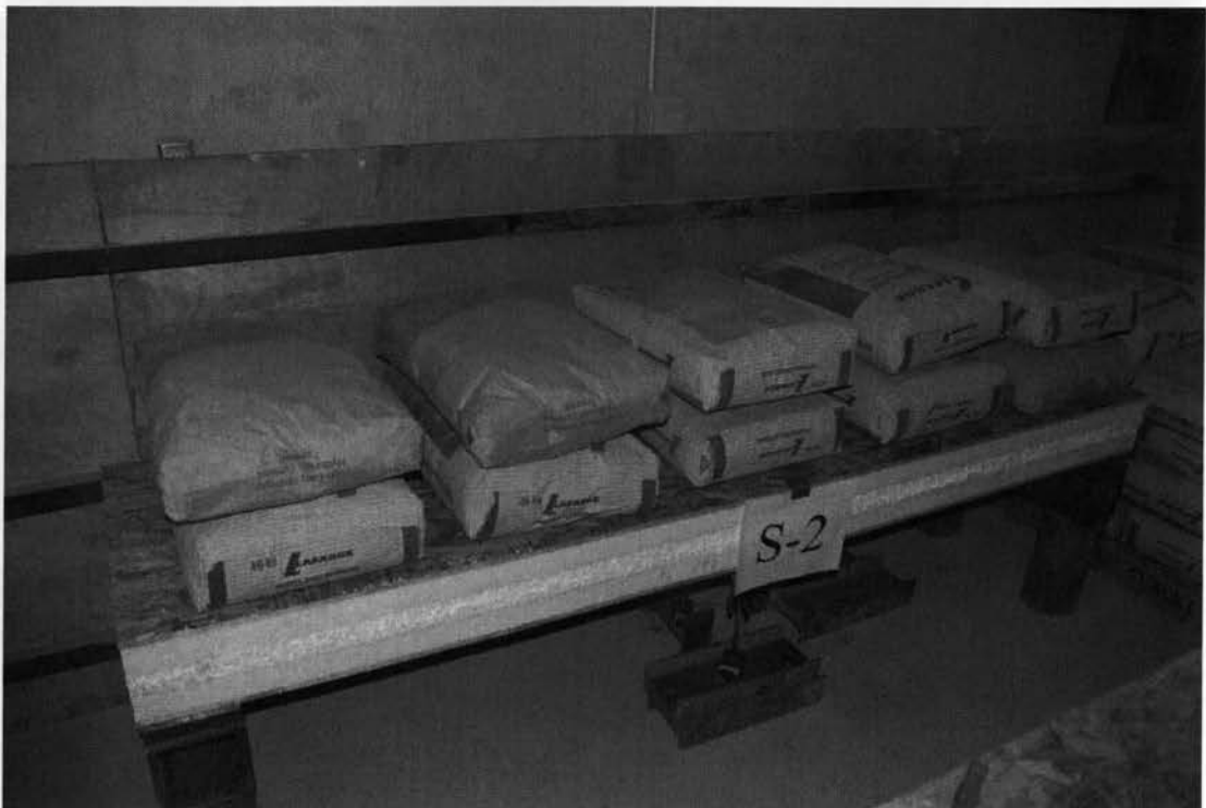
Fig. 3.14 View of dead and live load over panel S-2
