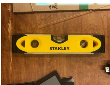
Figure 44: A level to ensure the camera and the album are even
