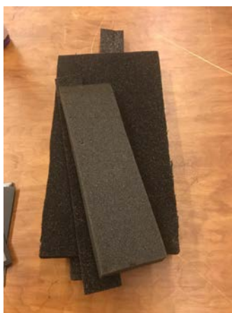
Figure 42: A selection of foam in different sizes and thickness to adjust the surface of the album while digitizing and flipping pages
