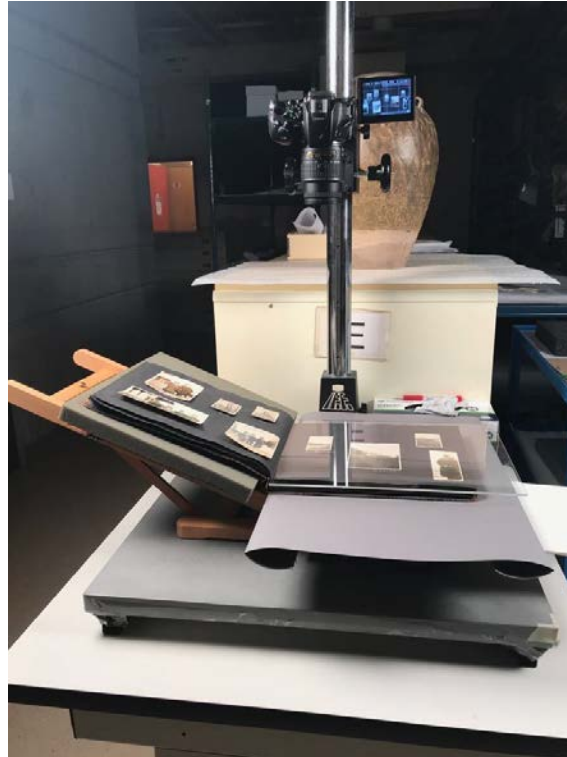
Figure 26: Author's recommended set-up for digitization of the family albums, using a book easel to support the album and a grey background to reduce the noise behind the album.
