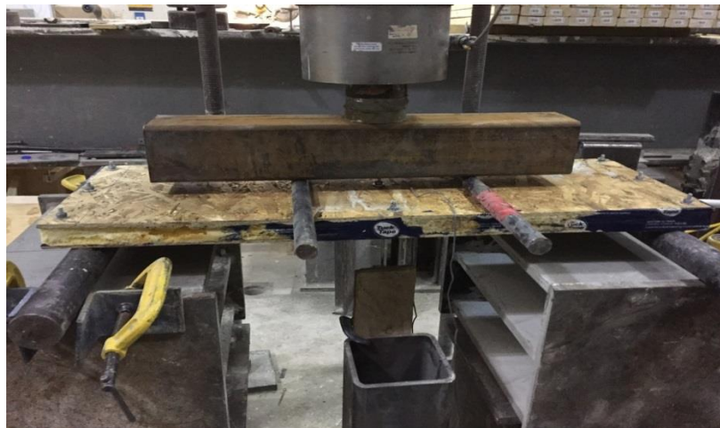
Figure 4.22- Four point flexural load test set-up for OSBSW wall
