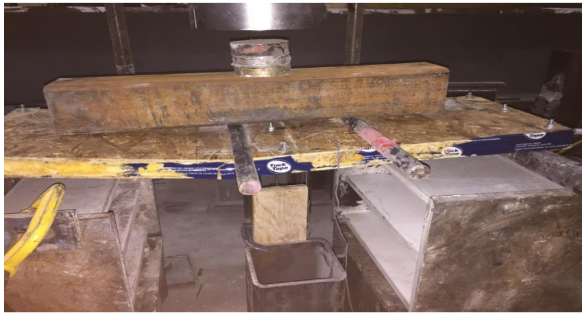
Figure 4.23- Failure of the wall during testing
