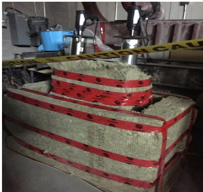
Figure 4.15- Test set up for thermal conductivity test of wall
