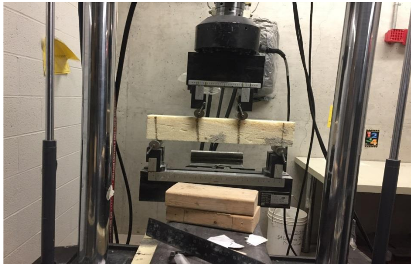
Figure 3.8- Four point loading test of commercial form material beam
