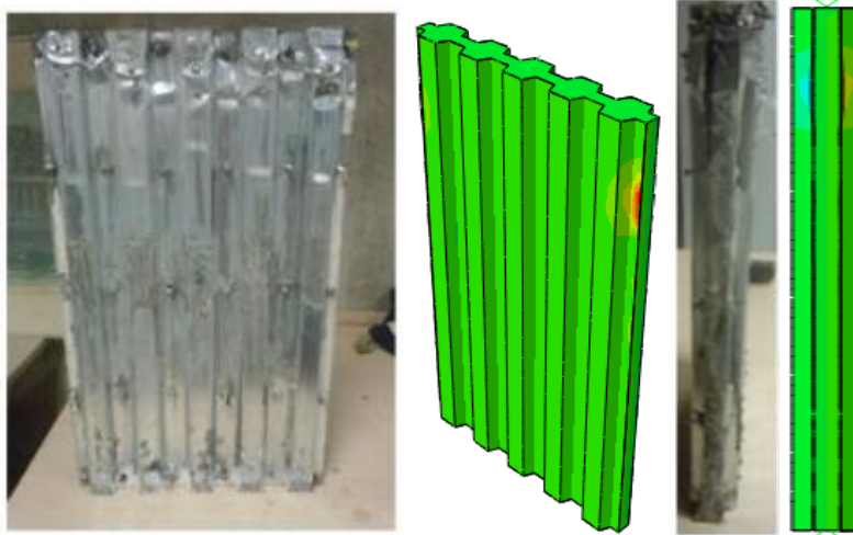
Figure 3.38: Experimental and FE failure shape for UHPC wall
