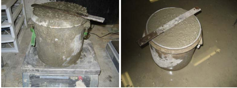
Figure 3.18 - Fresh density test and Fresh density test
