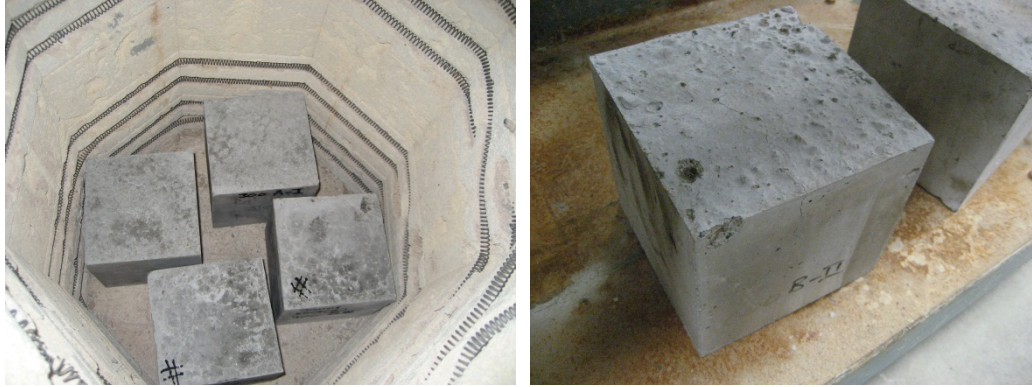
Figure 8.10 - LWS-C specimens during elevated temperatures test
