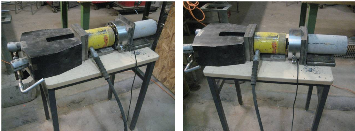
Figure 7.35 - Pull-out test of LWSCC cylinders
