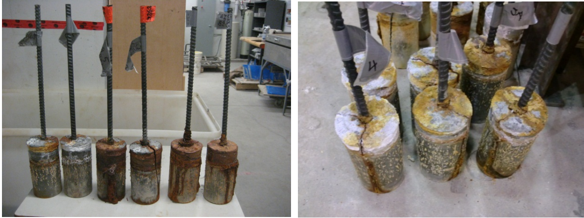
Figure 8.3 - LWSCC specimens after accelerated corrosion test
