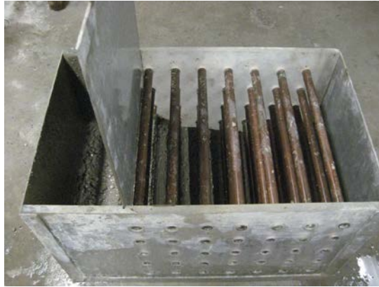
Figure 3.15 - V- Funnel test and filling capacity test
