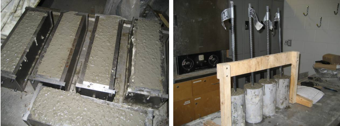
Figure 7.7 - Preparation of LWSCC freeze – thaw prisms and cylinders for bond test
