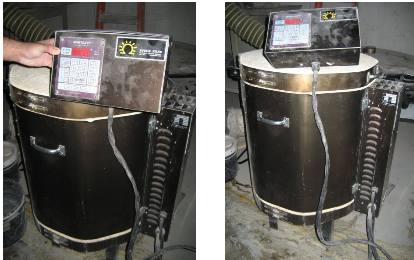
Figure 8.11 - Controlled furnace used during elevated temperatures test
