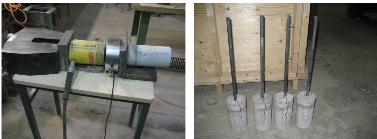
Figure 7.36 - Pull-out test set up and LWSCC specimens after testing
