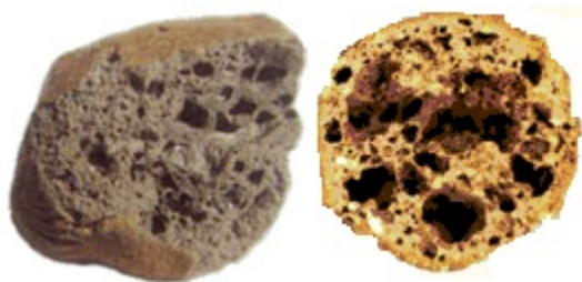
Figure 2.3 - Internal pore structure of lightweight aggregate
