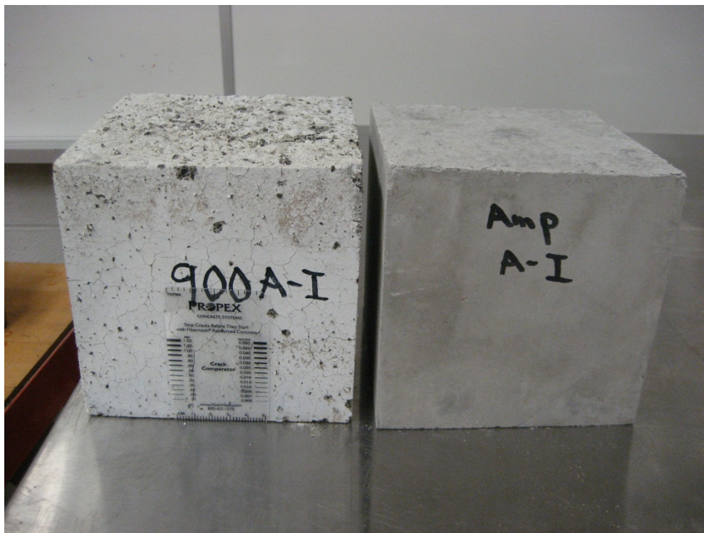
Figure 8.13 - EC-LWSCC specimens after undergoing elevated temperatures tests
