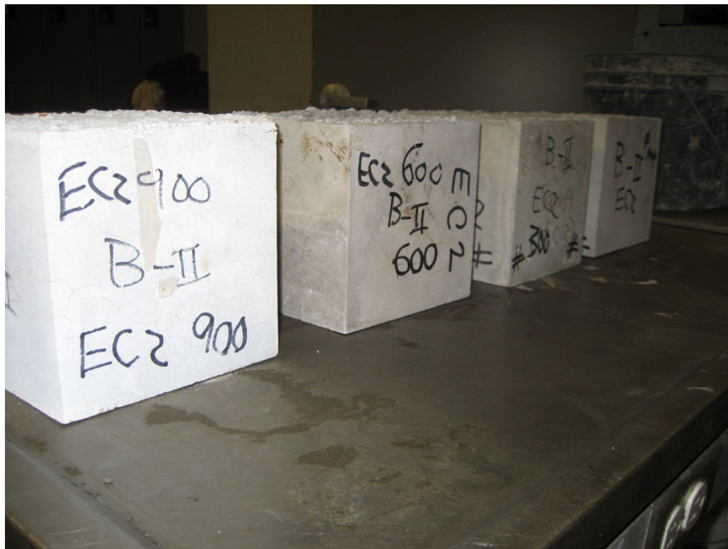
Figure 8.16 - Discoloration of LWSCC specimens after specimens after the 900°C exposure tests
