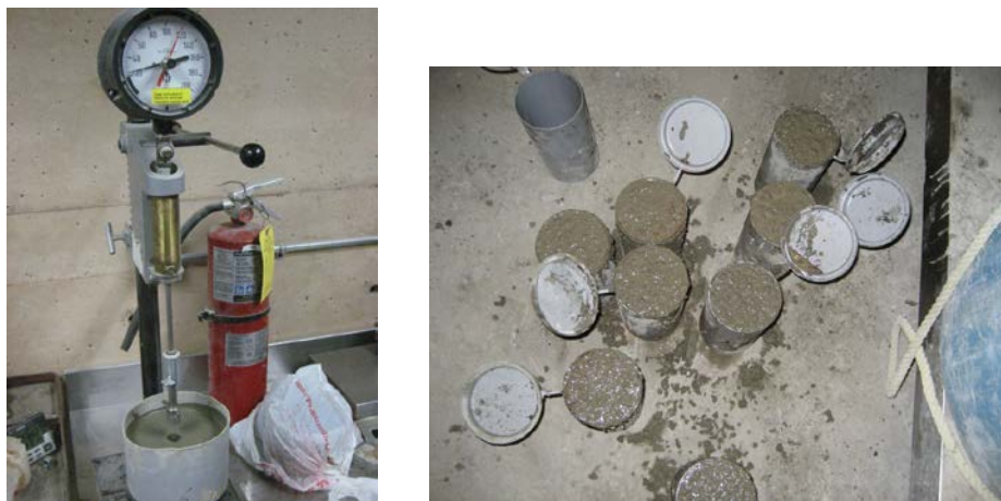
Figure 3.20 - Penetration resistance test (set time test) and moulds casting
