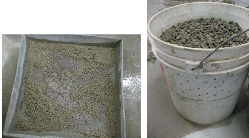
Figure 3.11 - Draining excess water form pre- soaked fines and coarse aggregates
