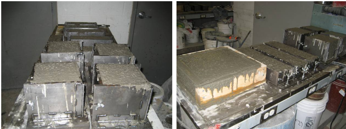
Figure 7.8 - Casting and preparing LWSCC specimens
