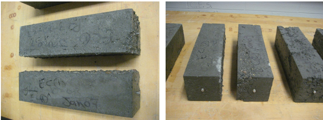
Figure 8.38 - Evaluating LWSCC specimens during freeze-thaw test
