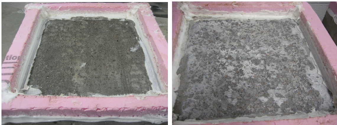
Figure 8.26 - FS/EC LWSCC specimens after undergoing salt scaling test
