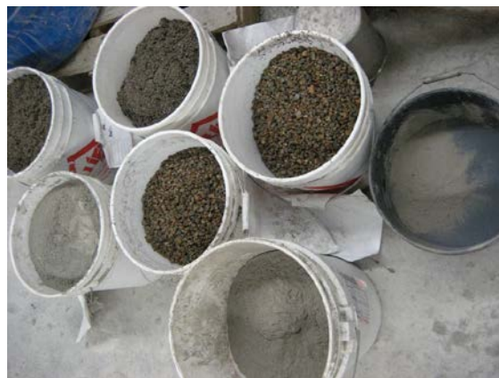
Figure 3.12 - Pre-weight mixture proportions
