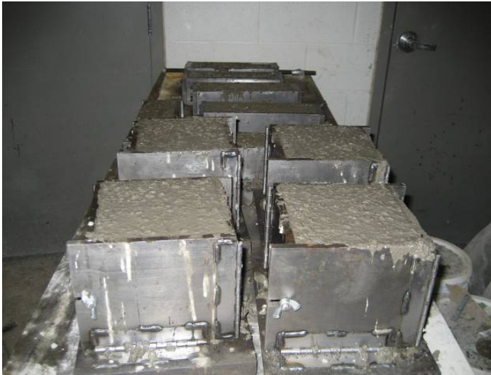
Figure 7.2 - Preparation of LWSCC elevate temperature and salt scaling specimens
