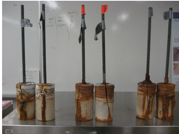
Figure 8.3 - LWSCC specimens after accelerated corrosion test
