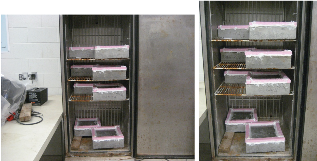
Figure 8.24 - Controlled freezer used salt scaling test
