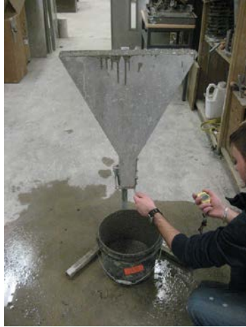
Figure 3.15 - V- Funnel test and filling capacity test
