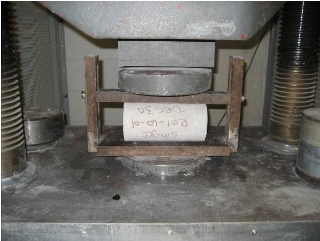
Figure 7.29 - Split tensile strength test of LWSCC cylinder
