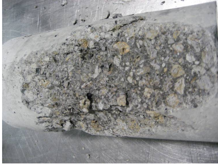
Figure 7.15 – Coarse FS aggregate fracture in the broken specimens
