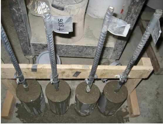
Figure 7.4 - Preparation of LWSCC specimens
