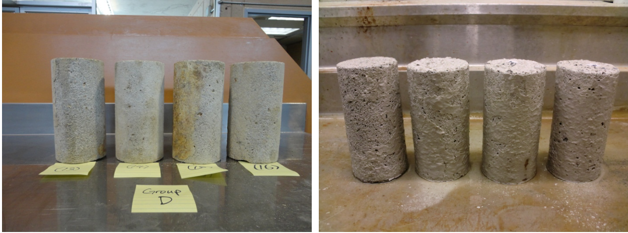
Figure 8.33 - LWSCC specimens under evaluation after exposure to sulfuric acid
