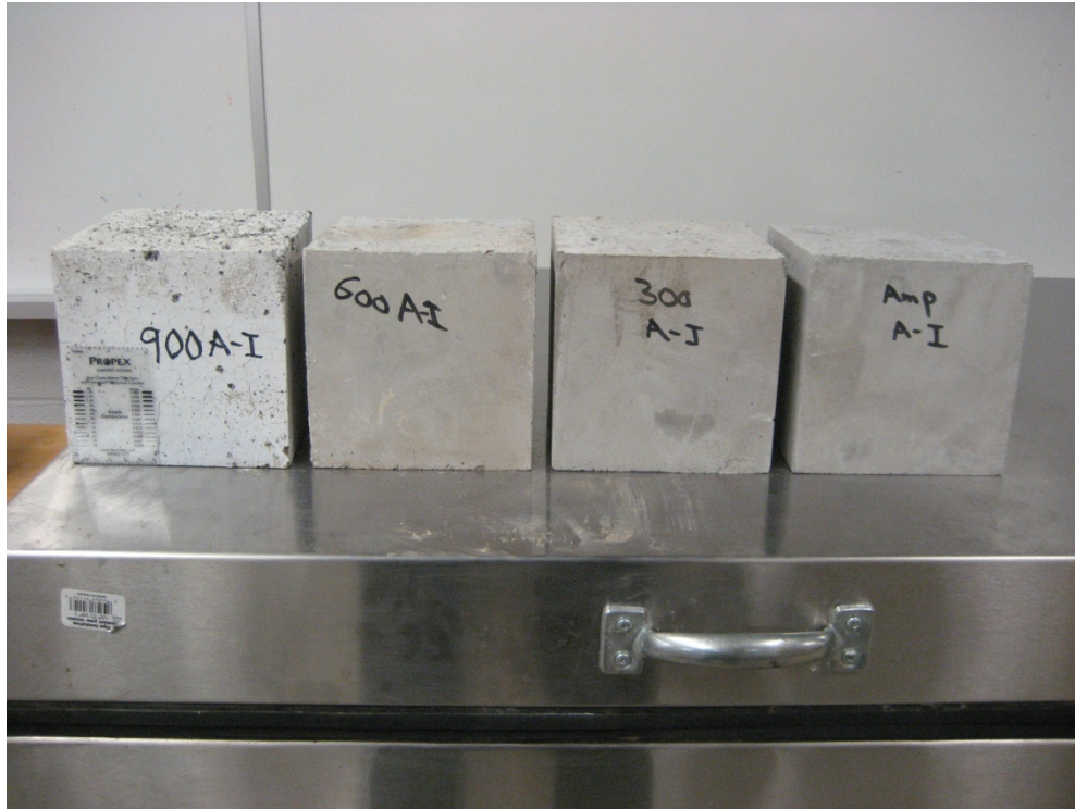
Figure 8.13 - EC-LWSCC specimens after undergoing elevated temperatures tests
