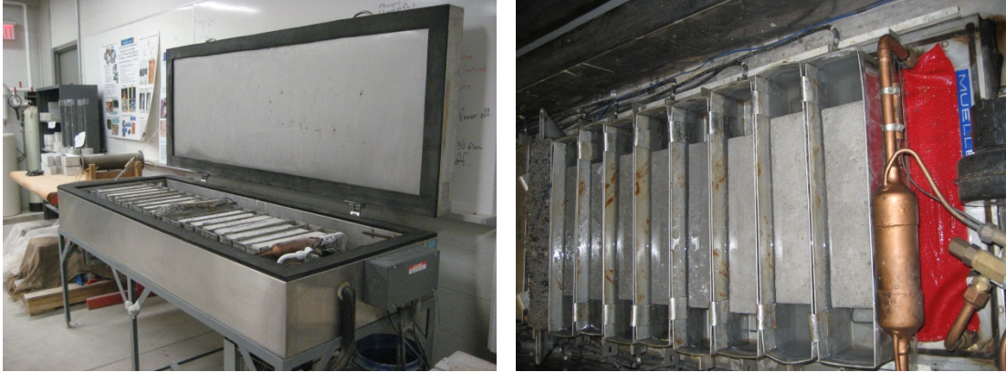
Figure 8.37 - LWSCC specimens undergoing freeze-thaw cycles
