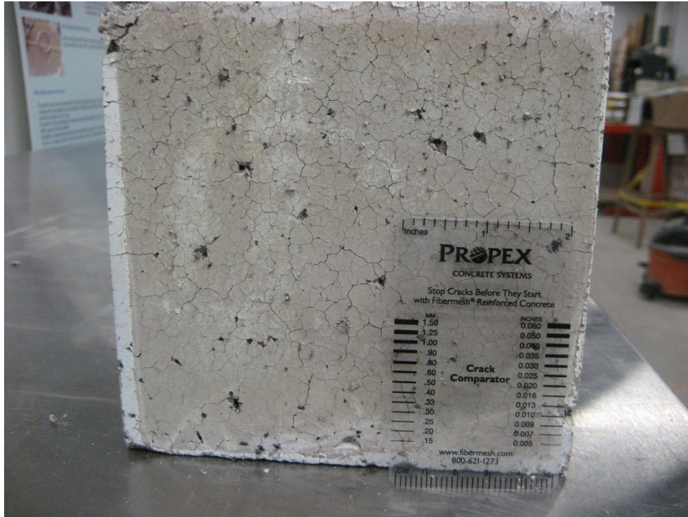
Figure 8.15 - Surface map cracks on FS-LWSCC specimens after the 900°C exposure test
