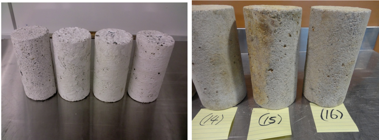
Figure 8.31 - LWSCC specimens undergoing exposure to sulfuric acid
