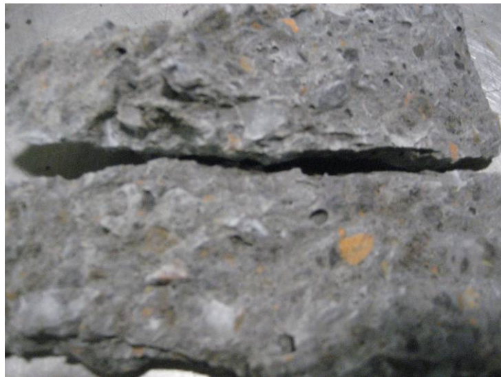
Figure 7.16 – Coarse ESH aggregate fracture in the broken specimens
