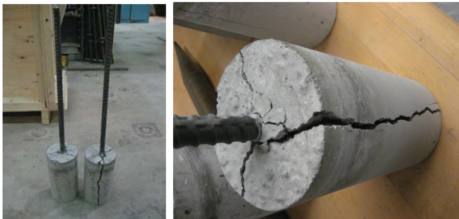
Figure 7.40 - Bond failure due to splitting with cracks forming at approximately 120^\circ
