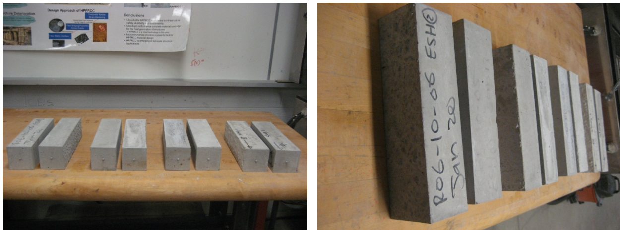
Figure 8.36 - LWSCC specimens before freeze-thaw test
