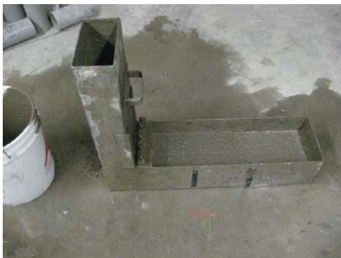
Figure 3.17 - L- Box test and bleed test
