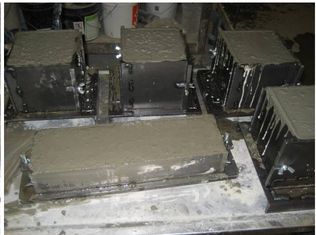
Figure 7.3 - Preparation of LWSCC shrinkage prisms and elevate temperature specimens
