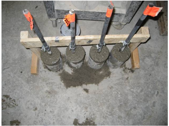
Figure 7.5 - Preparation of LWSCC specimens
