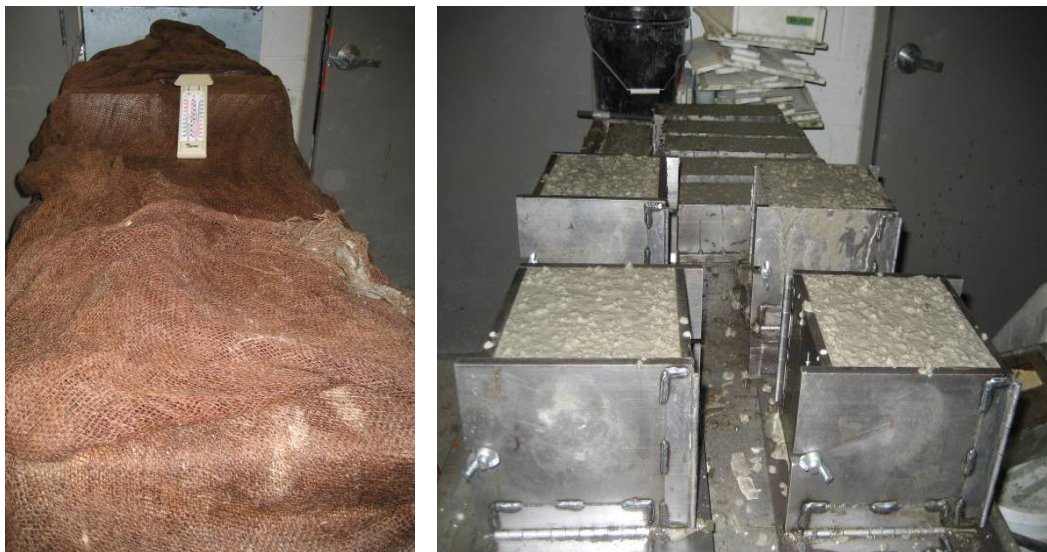
Figure 7.9 - Casting initial curing of LWSCC specimens
