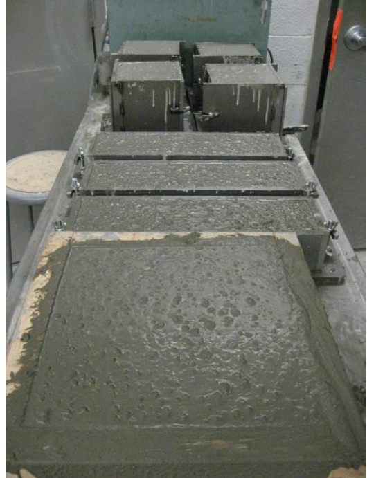
Figure 7.2 - Preparation of LWSCC elevate temperature and salt scaling specimens
