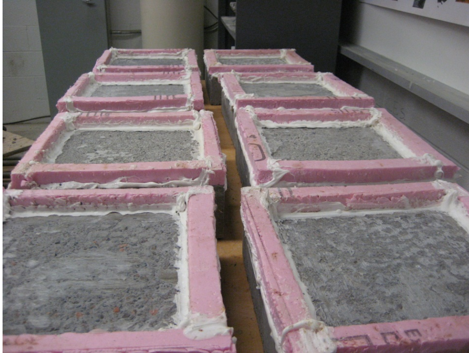
Figure 8.27 - LWSCC specimens specimen after undergoing salt scaling test
