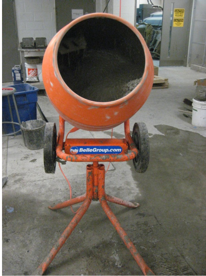
Figure 3.9 - Drum rotating mixer
