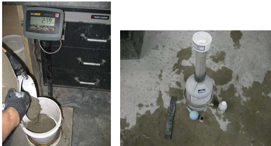
Figure 3.19 - Sieve segregation resistance test and air content test (volumetric method)
