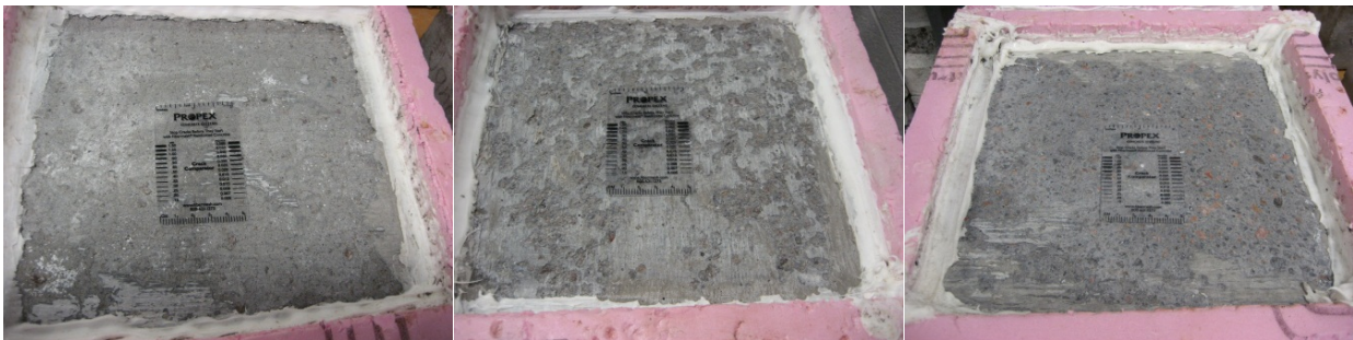
Figure 8.28 - FS/EC/ESH LWSCC specimens after undergoing salt scaling test
