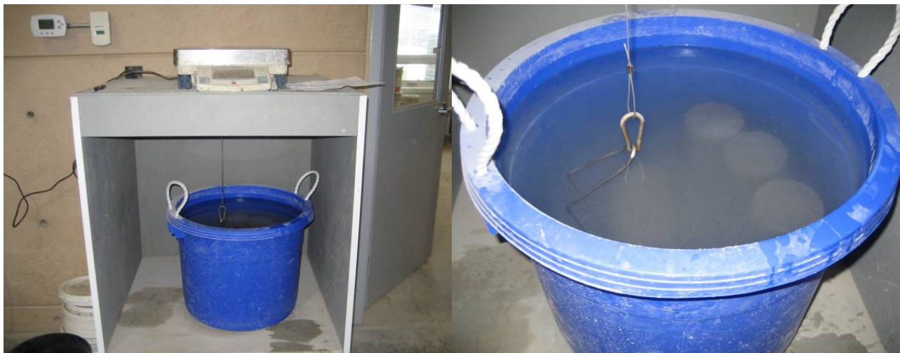
Figure 7.44 - Absorption and porosity test of LWSCC specimens
