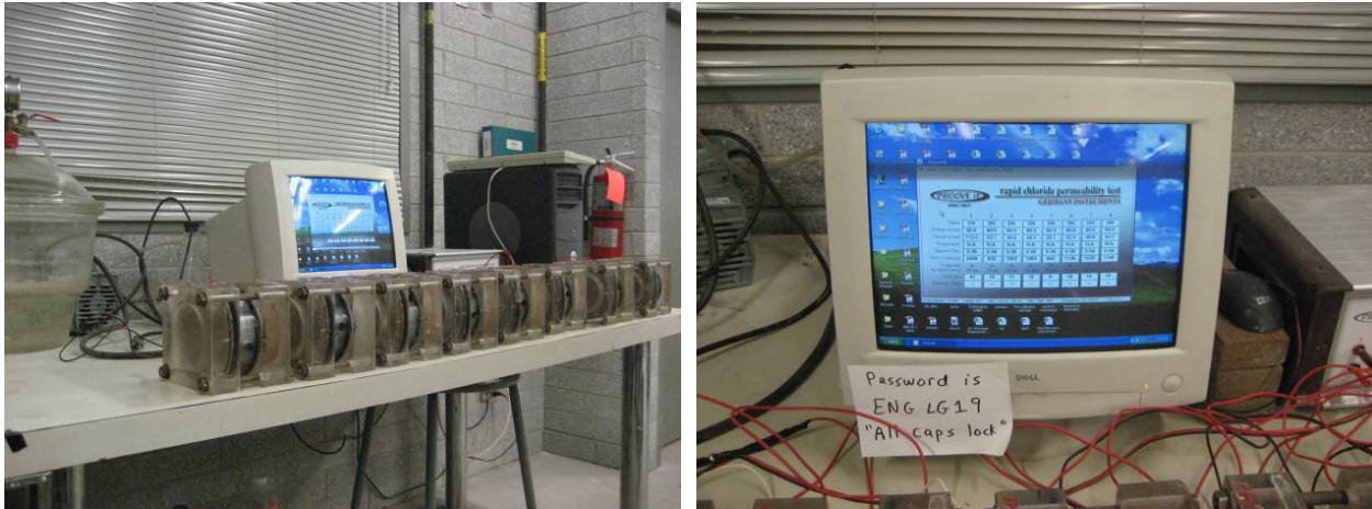
Figure 7.53 - LWSCC samples undergo RCPT and “Germann Prove-it” software screen
