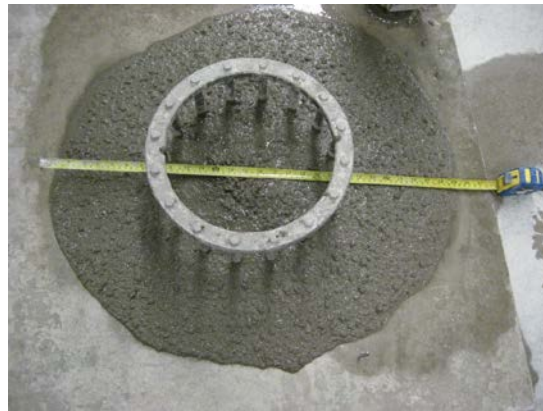
Figure 3.16 - J-ring and J- ring height test
