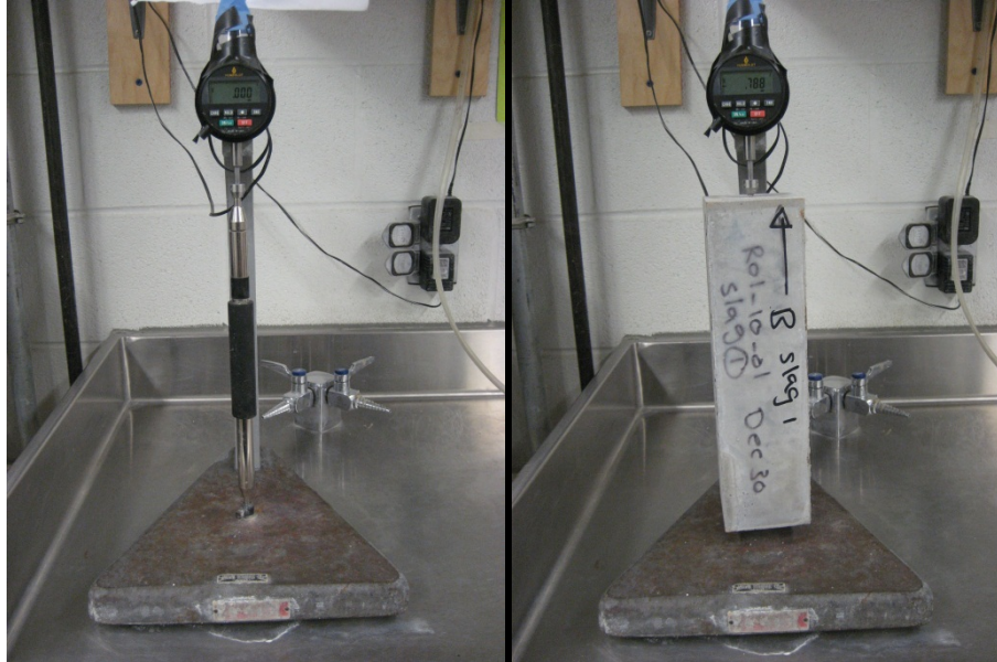
Figure 7.56 - Drying shrinkage test of LWSCC prisms
