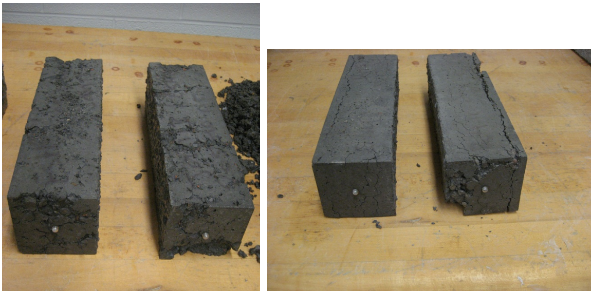
Figure 8.40 - Evaluating LWSCC specimens during freeze-thaw test
