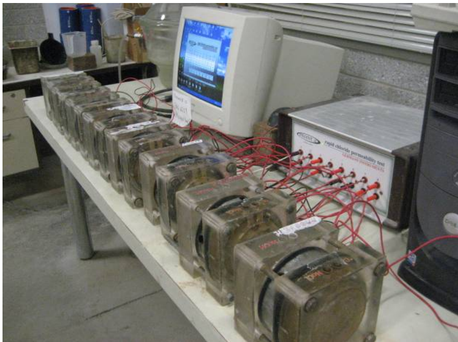
Figure 7.54 - LWSCC samples after RCPT test
