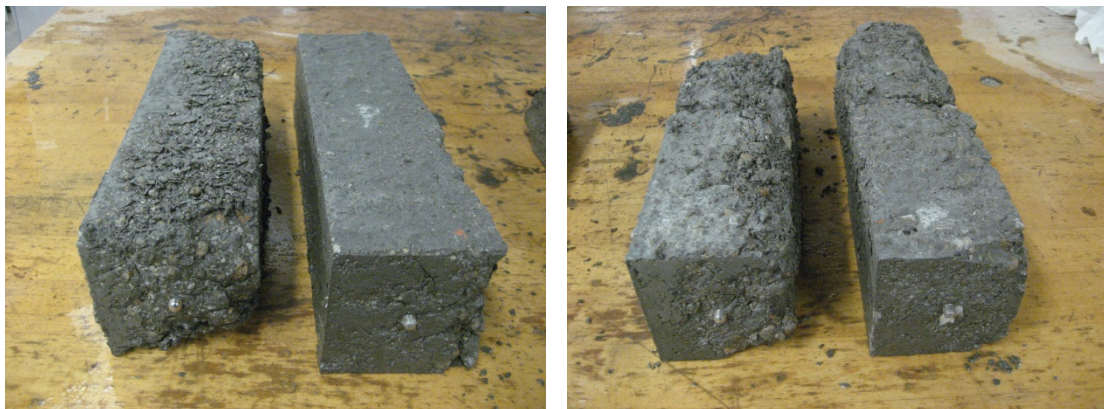
Figure 8.41 - Evaluating ESH-LWSCC specimens after freeze-thaw test
