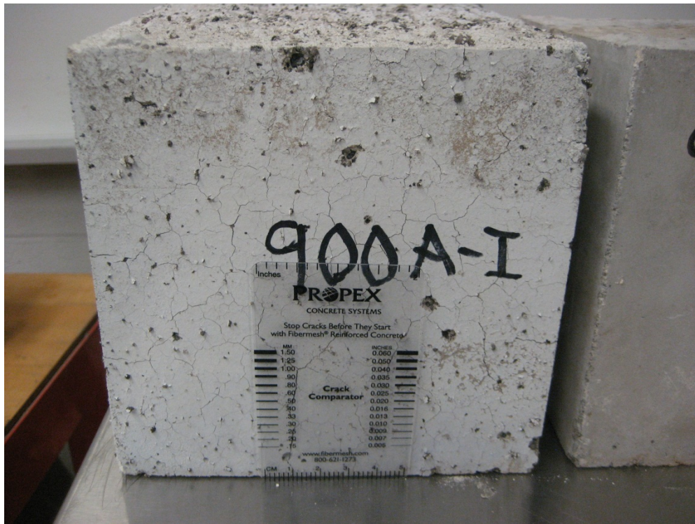
Figure 8.17 - ESH-LWSCC specimens after the 300 and 600 0 C exposure tests
