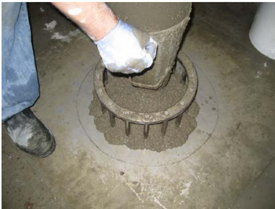
Figure 3.16 - J-ring and J- ring height test
