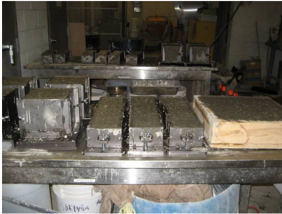
Figure 7.5 - Preparation of LWSCC specimens
