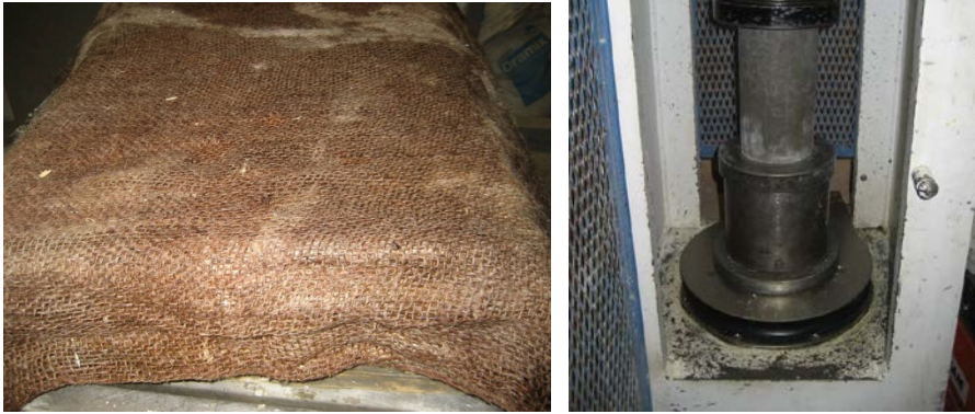
Figure 3.21 - Wet burlap curing in the first 24 hrs and compressive strength test
