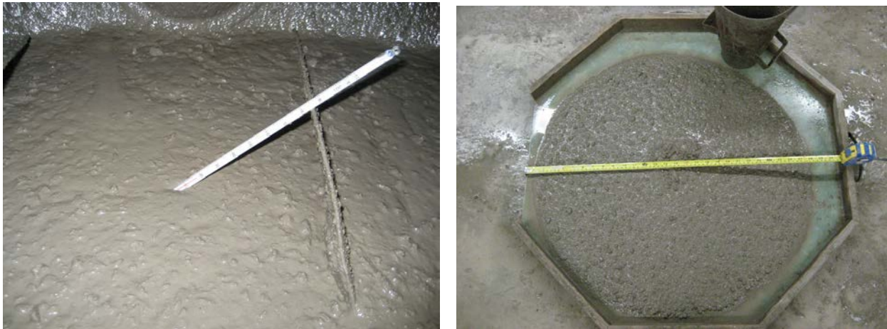
Figure 3.14 - Mixture temperature and slump flow test - measure of flowability
