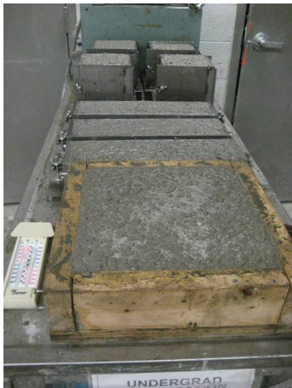
Figure 7.6 - Preparation of LWSCC specimens
