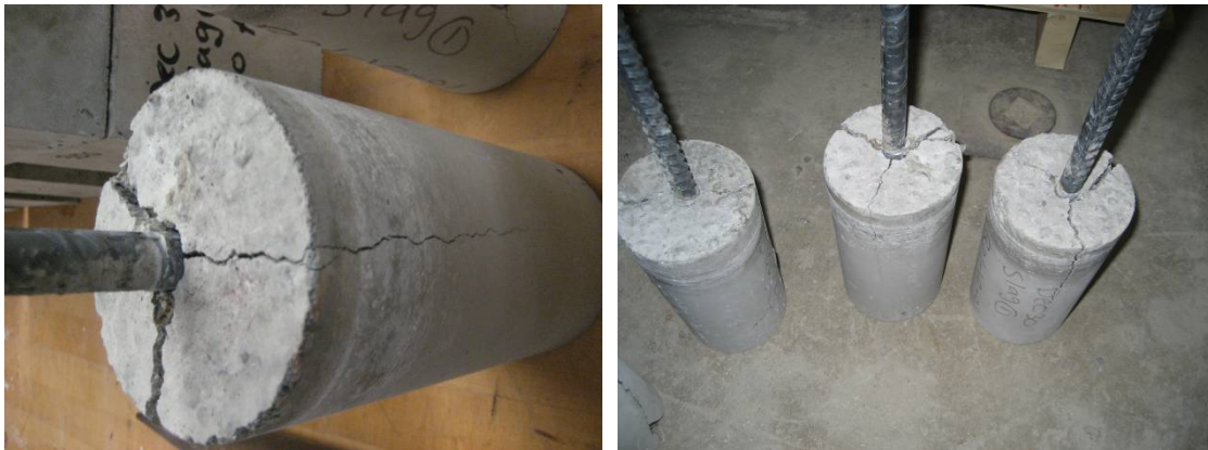
Figure 7.39 - Bond failure due to splitting with cracks forming at approximately 120^\circ
