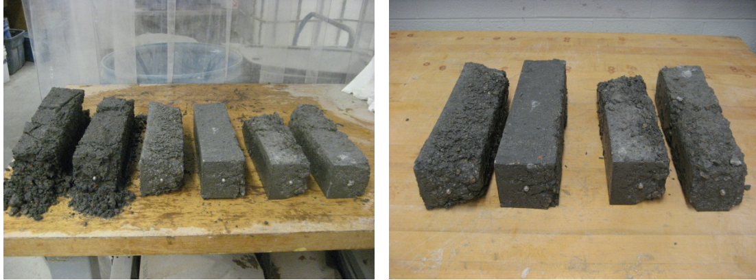
Figure 8.43 - Failed LWSCC specimens during freeze-thaw test
