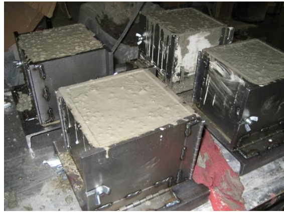
Figure 7.4 - Preparation of LWSCC specimens
