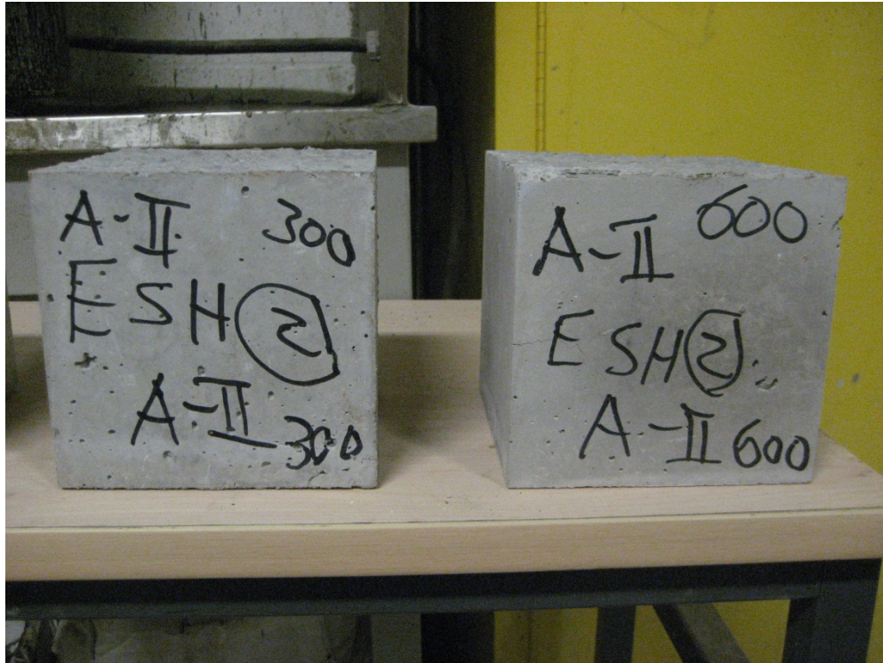
Figure 8.17 - ESH-LWSCC specimens after the 300 and 600 0 C exposure tests
