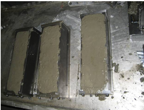
Figure 7.3 - Preparation of LWSCC shrinkage prisms and elevate temperature specimens
