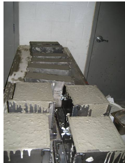
Figure 7.6 - Preparation of LWSCC specimens
