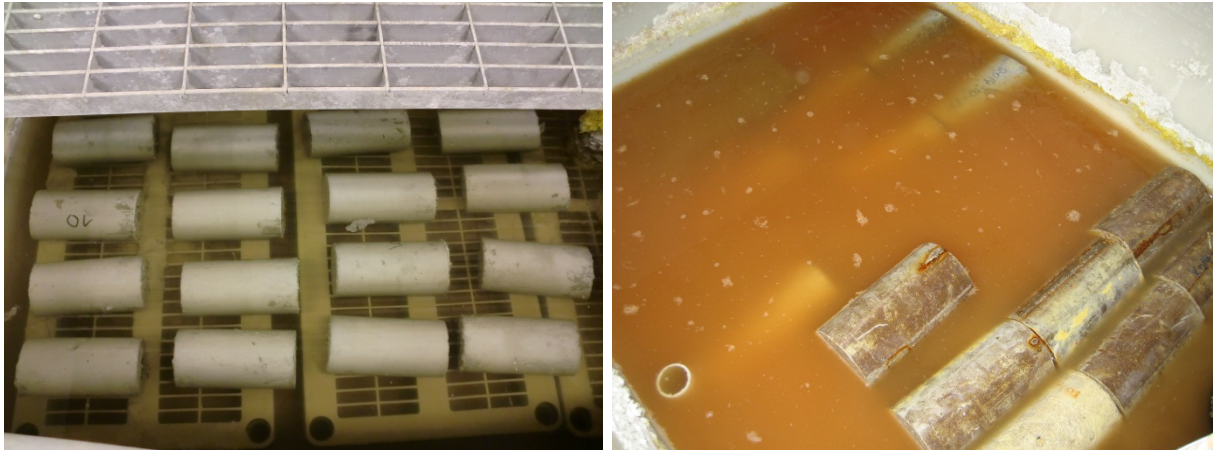
Figure 8.31 - LWSCC specimens undergoing exposure to sulfuric acid
