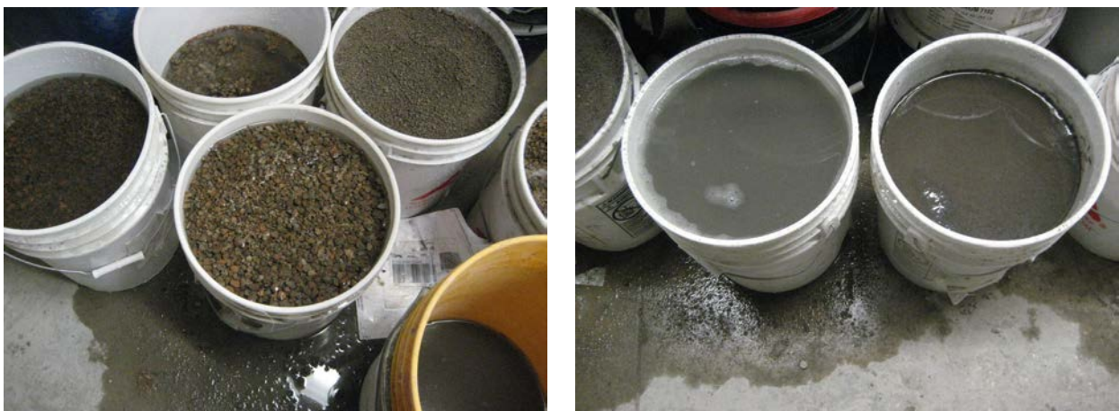
Figure 3.10 - Aggregates 72 hrs pre-soaking
