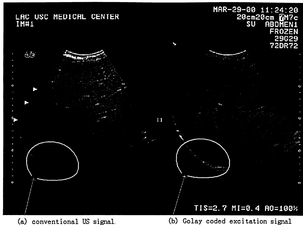
Figure 1.22 Golay Coded Excitation Signal and Conventional Signal The Benefits of Coded Excitation are Clearly Demonstrated in this Side-by-side Liver Comparison. Note the 20-cm Penetration while Maintaining 7-MHz Resolution
