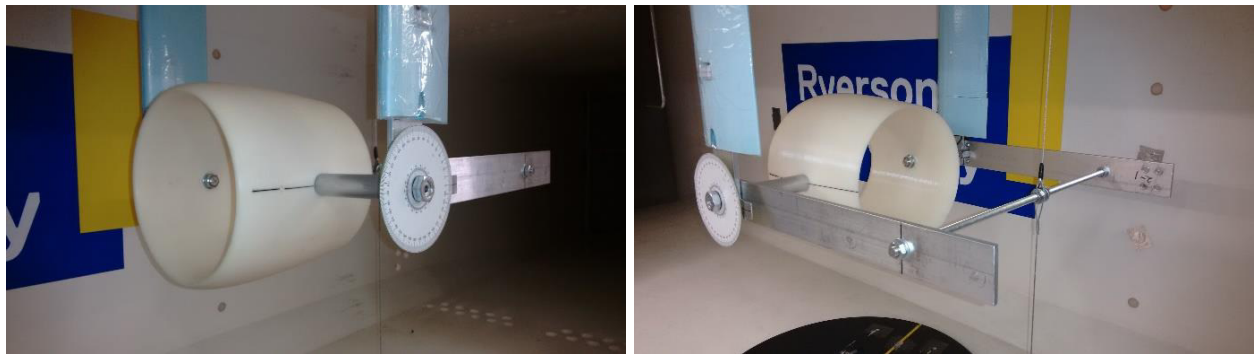
Figure 4-6: The mechanism used for measuring experimental pitching moment in the wind tunnel
