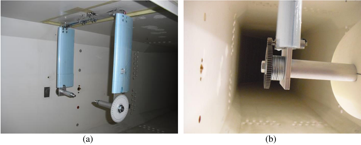
Figure C. 4: (a) Supporting frame, and (b) Gear system for tilting ducts
