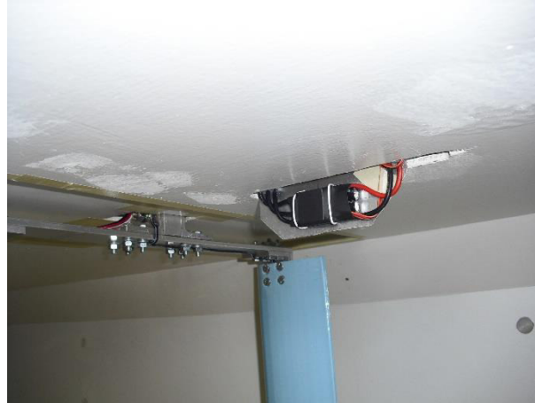
Figure C. 6: Installation of speed controller in the test section at the back of supporting frame
