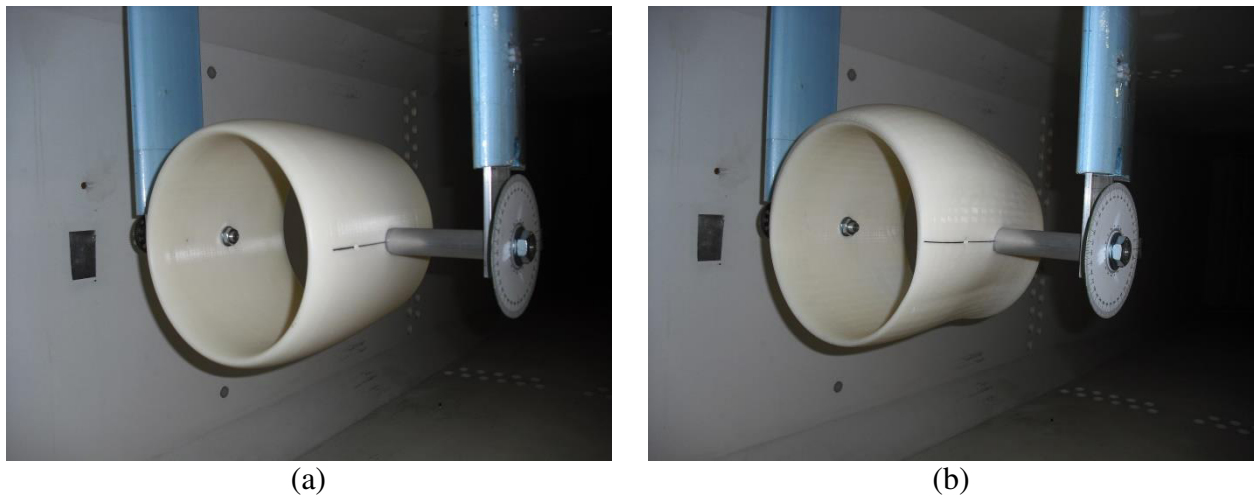
Figure 4-5: The symmetrical and asymmetrical ducts installed in the wind tunnel
