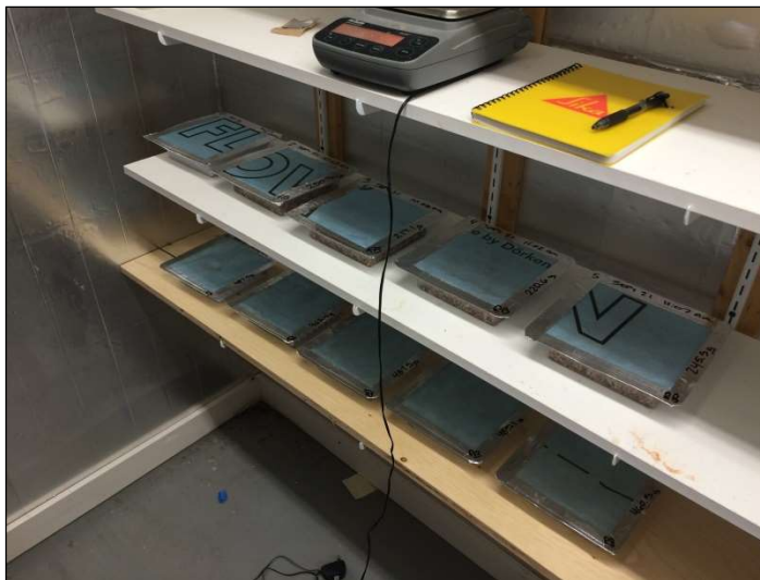
Figure 10 – Dry cup and wet cup samples placed in a climate chamber at 25°C and 50% RH.
