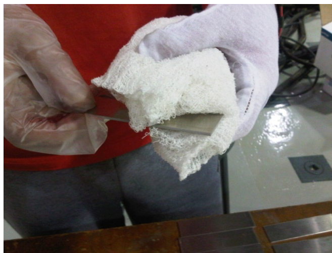
Figure 4.6 - Wiping Down with Degreaser
