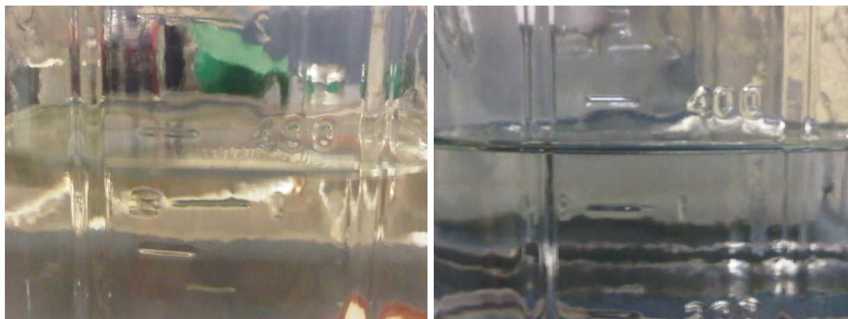
Figure 3.3 - Fuel Levels Before and After Soaking at 163 C Respectively
