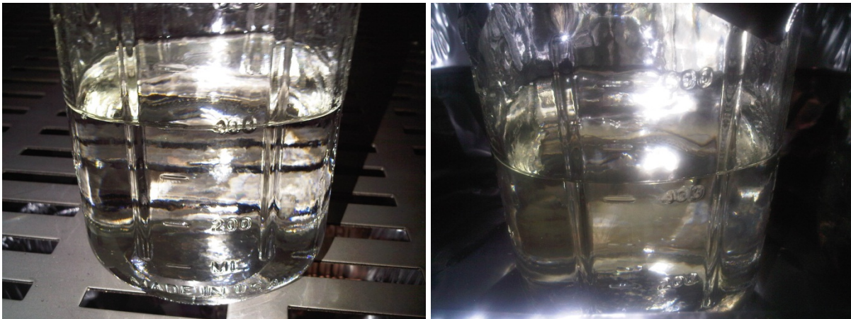
Figure 3.2 - 400 mL of Jet A1 Fuel @ 163C Expansion to ~430 mL (Before and After Respectively)
