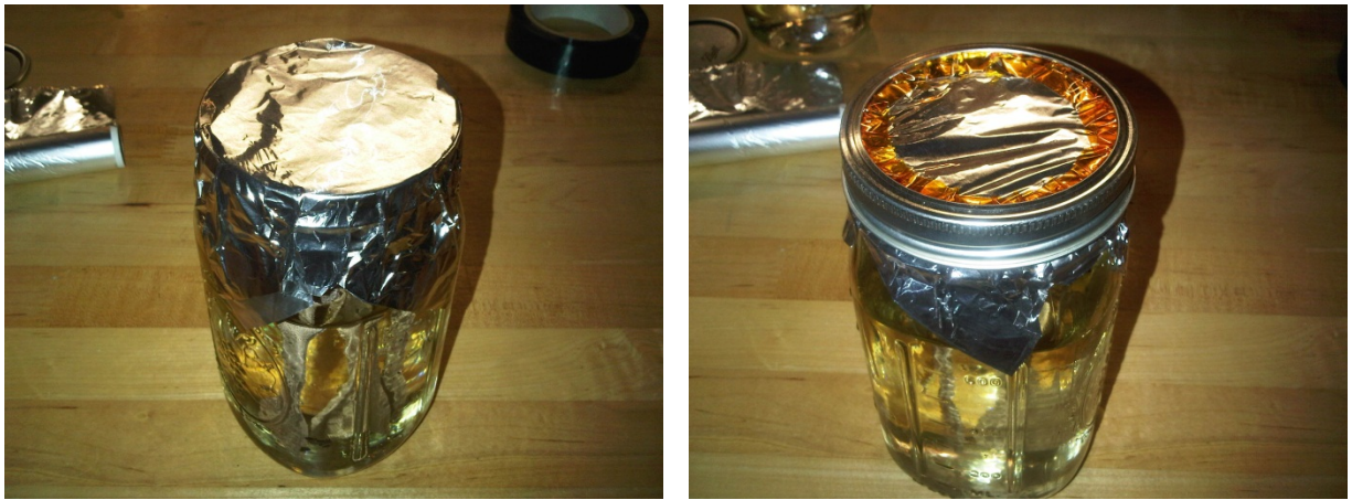
Figure 3.4 - Revised Jar Sealing Method
