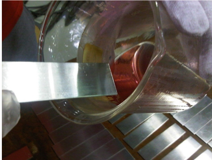
Figure 4.7 - Soaking Specimens in Acetone Bath
