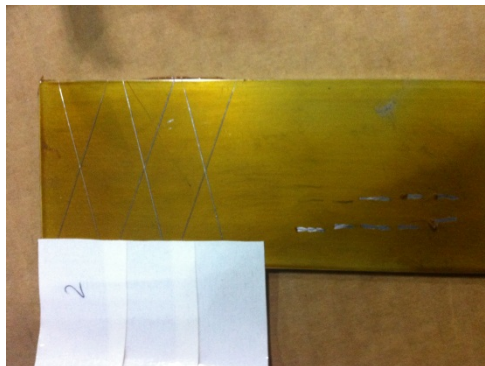
Tape Adhesion and Scratch Hardness 825X309 & EC776 Respectively JetA1
