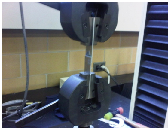
Figure 3.6 - Lap Shear Gripped in Tensile Machine
