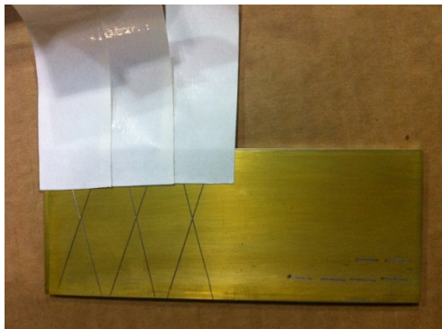
Tape Adhesion and Scratch Hardness 825X309 & EC776 Respectively Bio50
