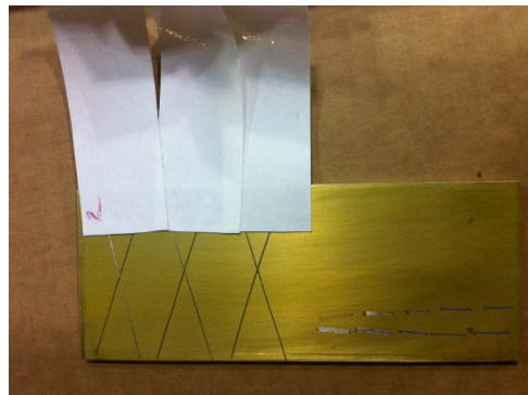
Tape Adhesion and Scratch Hardness 825X309 & EC776 Respectively Bio50
