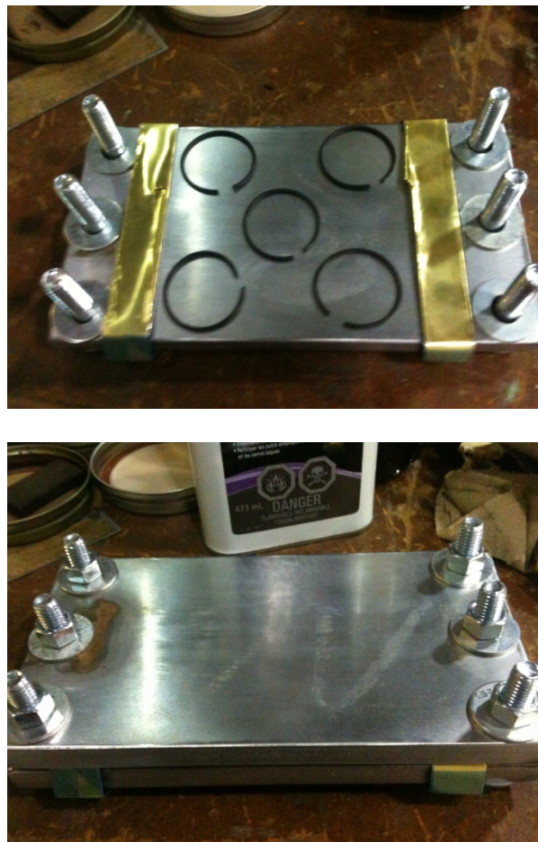
Figure 3.15 - Compression Plate and O-Ring Setup
