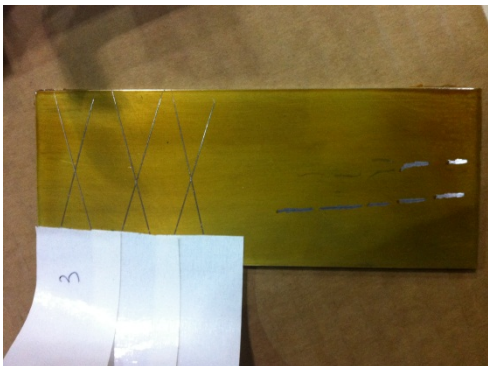
Tape Adhesion and Scratch Hardness 825X309 & EC776 Respectively JetA1
