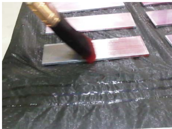
Figure 4.18 - Brush Application of EC 776
