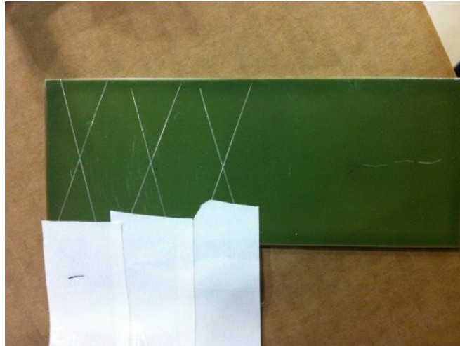
Figure 5.4 - Tape Adhesion Results of 825X309 in Jet A1
