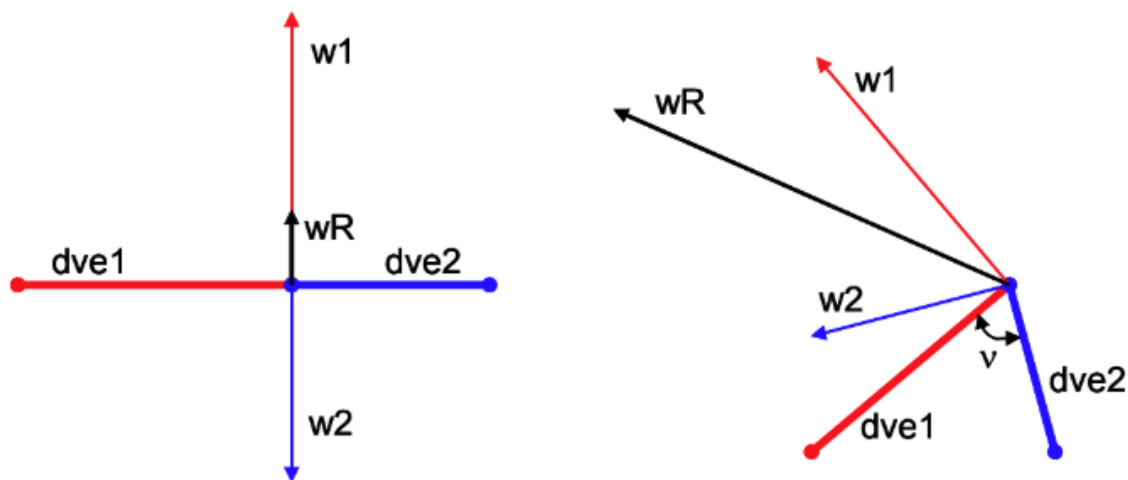
Figure 1-4. False Velocity Spike when DVE's are not coplanar [5]
