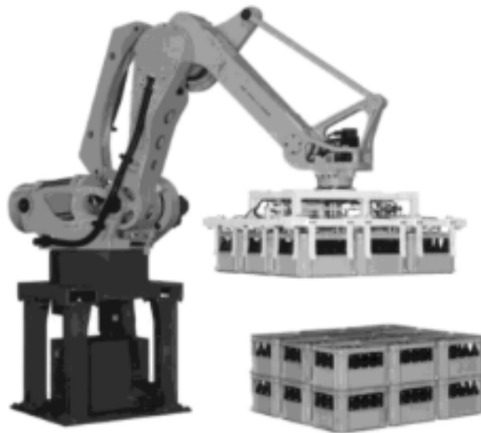
Figure 7: A Fanuc M-410iWW palletizing robotic manipulator with its end effector (Niku, 2010: 7)
