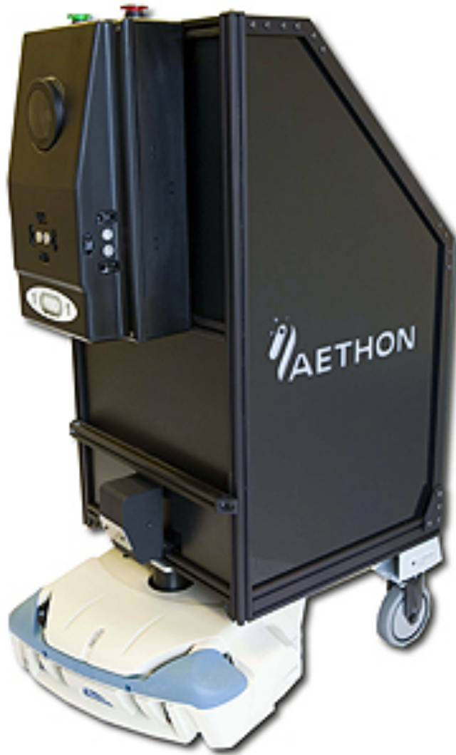
Figure 10: Homer, an RFID-enabled version of Aethon's Tug robot (O'Connor)
