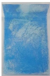
Figure 3.1 PS substrate coated by electrospray deposition of diblock copolymer 15 and stained with BPB
