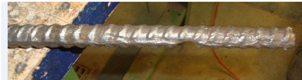
Figure 4.55: Rib profile of rebar after brushing corrosion dust (Mix ID 16L2)
