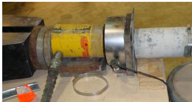
Figure 3.15: Pullout test setup [Mix ID: 20L2]
