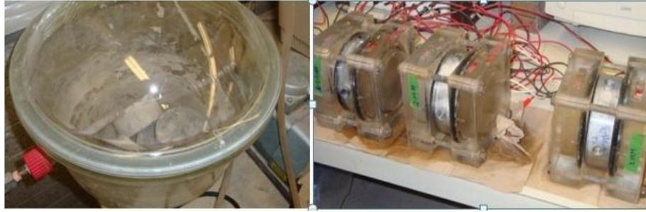
Figure 3.16: RCPT test setup showing specimen in dessicator and during testing
