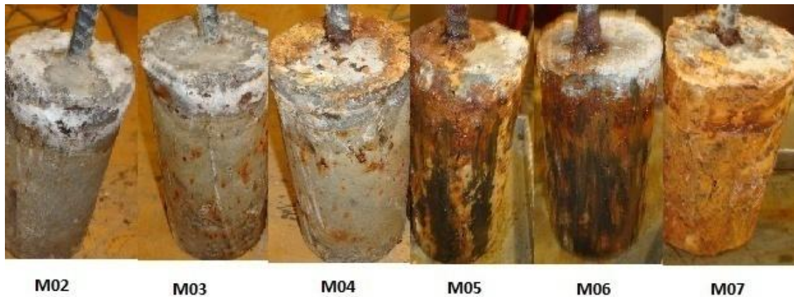
Figure 4.56: Effect of corrosion on concrete mixtures with shorter steel fibers (start from left: 4L1, 8L1, 12L1, 16L1, 20L1 and 24L1)
