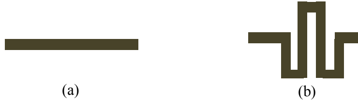
Figure 4-10 Anchoring springs (a) rectangular (b) serpentine
