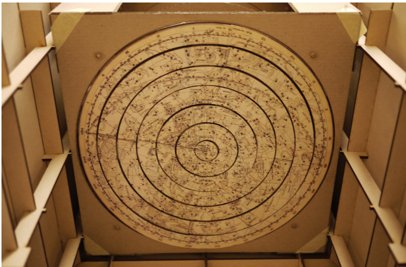
Figure 2.27 (above): View of the puzzle at one end of the machine, it is attached to a series of concentric rings that are able to freely rotate. These rings are moved by the rods.
