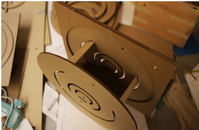
Figure 2.25 (right top): Model showing a revised puzzle mechanism, the previous version is much simplified from multiple layers into one. The puzzle is no longer attached directly to the rods, but are driven by a series of rings that are operated by the movement and rotations of the rods.
