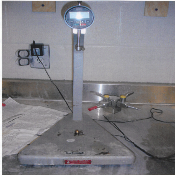
Figure 3.1: Comparator used for expansion measurement
