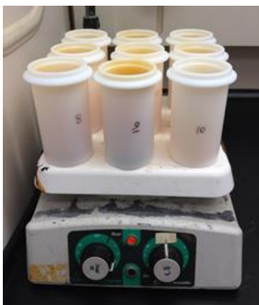
Fig. 3. Setup for acid evaporation using a hot plate
