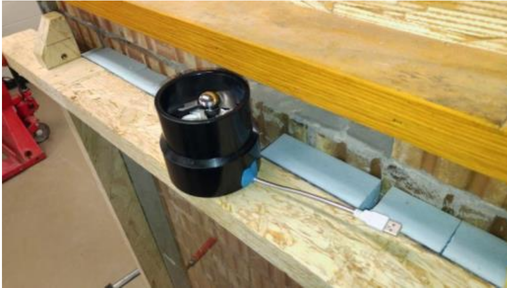
Figure 4 – Components of suction system used to simulate ventilation air
