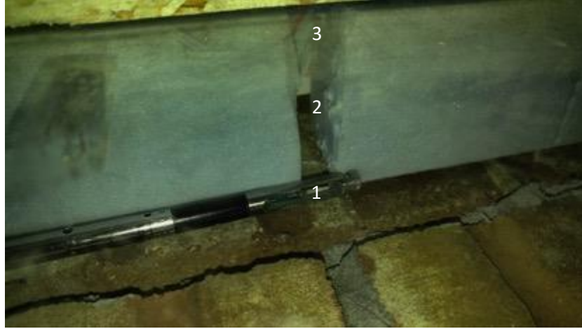
Figure 6 – Hot-wire anemometer probe at position closest to backside of wall specimen. Three measurements taken at vent opening and an average used for ACH calculations.
