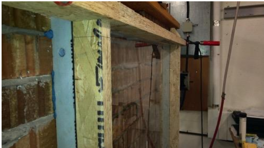
Figure 3 – Cavity frame with putty adhesive acting as an air seal. Note the eyehole punched through the insulation, this was used for air velocity measurements.
