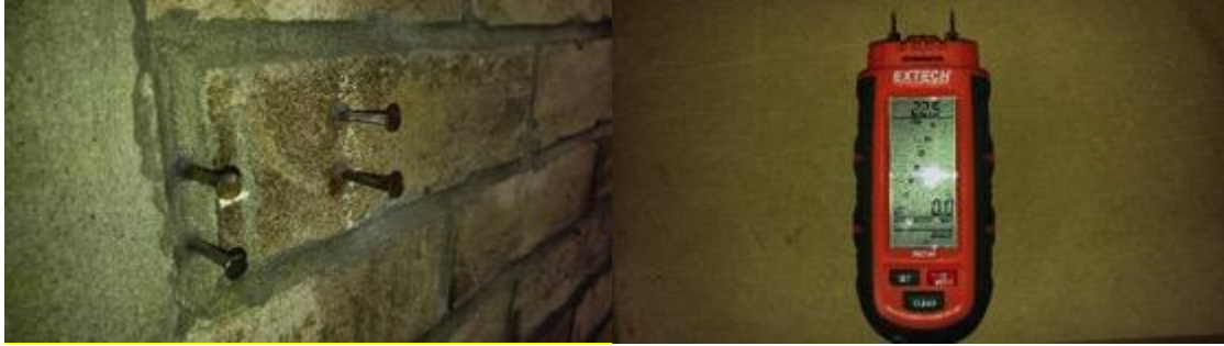
Figure 11 – Typical installation of moisture meter pins shown on left. Extech MO230 Moisture meter shown on right
