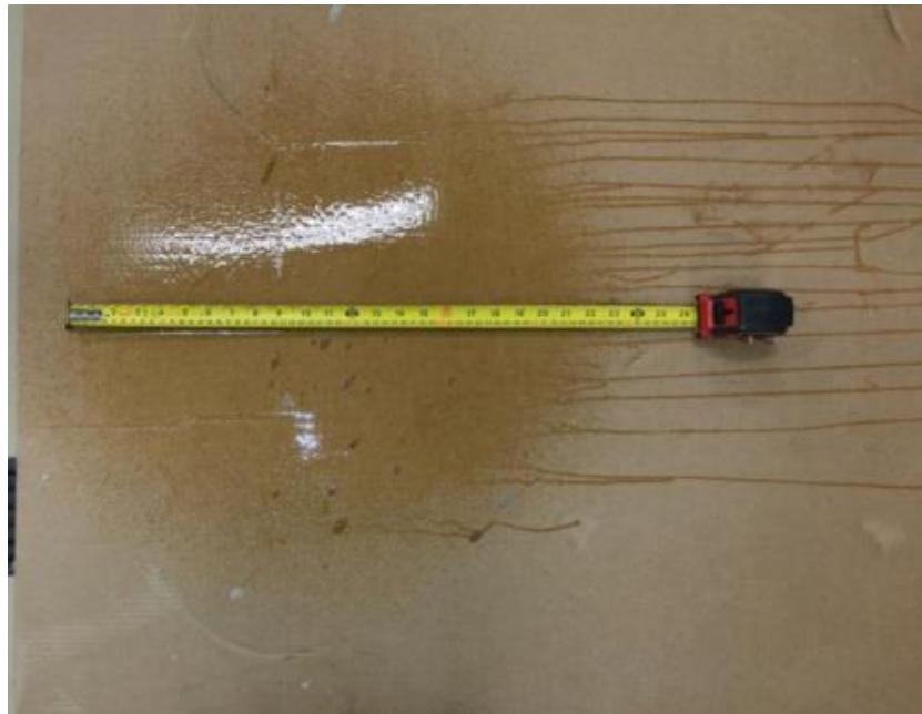
Figure 2 – spread pattern from Lee Valley misting head at 30 cm, 25 PSI
