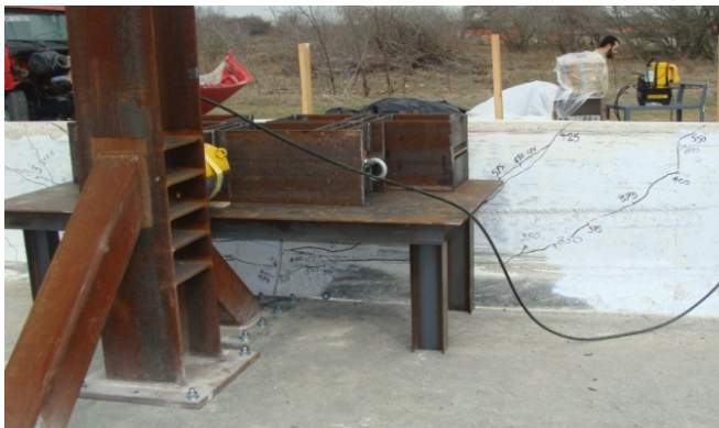
Figure 4.24 Cracks appeared at front face during testing at interior load location
