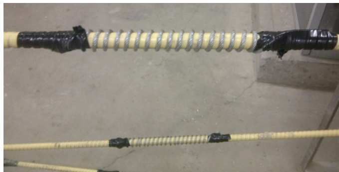
Fig. 3.6 Metal rope wrapped around a 12-mm diameter bar at the grip location
