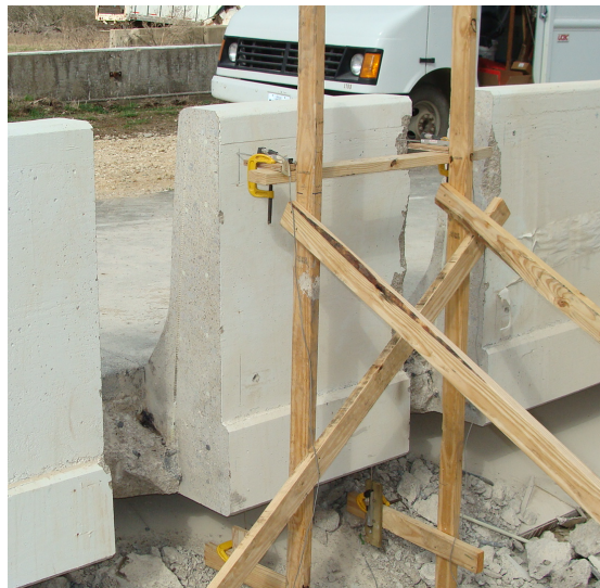
Fig. 4.8 View of LVDT location in Sample 1: two LVDTs at the top of the wall oriented horizontally and 2 LVDTs at the bottom of the deck edge oriented vertically
