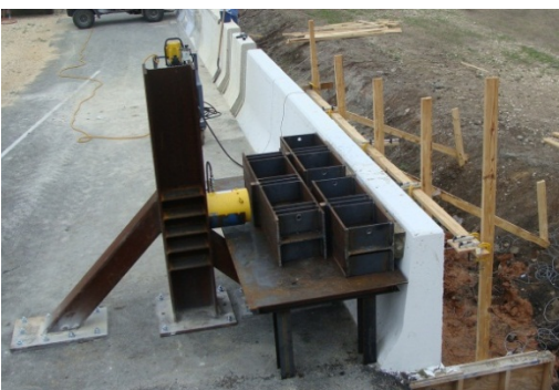
Fig. 4.16 Views of the test setup and sensor location at (a) front and (b) back of the barrier wall at end load location
