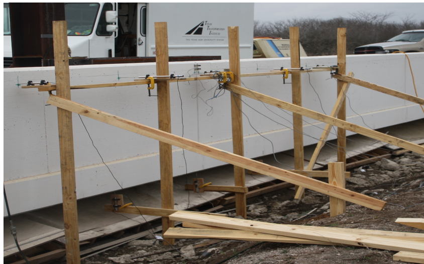
Fig. 4.12 View of back face of Sample 5 showing 5 LVDTs oriented horizontally at the top of the wall and 3LVDTs oriented vertically at the bottom of the deck edge.
