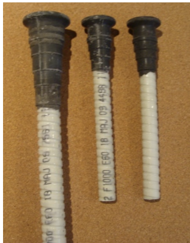
Fig. 1.2 View of GFRP bars with cast heads
