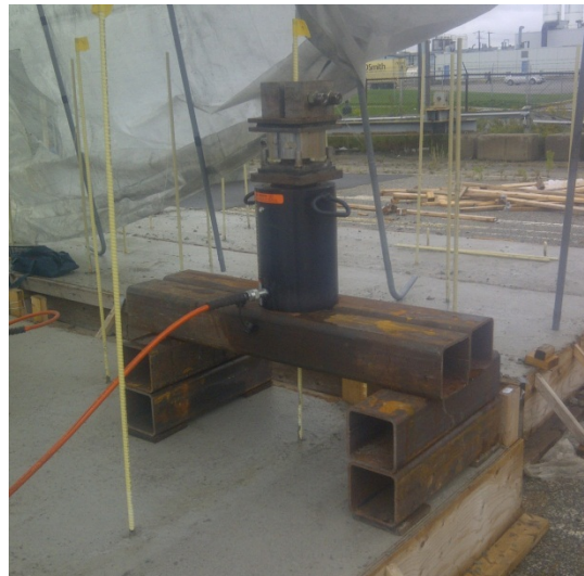
Fig. 3.3 Test setup for slab pullout testing
