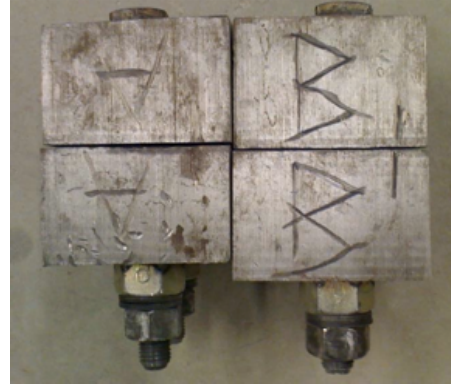
Fig. 3.4 Views of steel grips used in pullout tests, clamping the bar from two opposite sides
