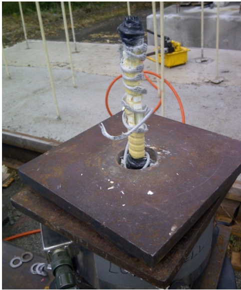
Fig. 3.8 Views of bar rupture at the location of the large grip
