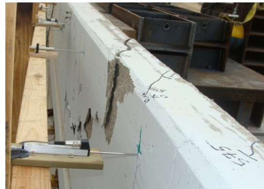
Figure 4.25 Punching shear crack appeared at end of the test at interior load location
