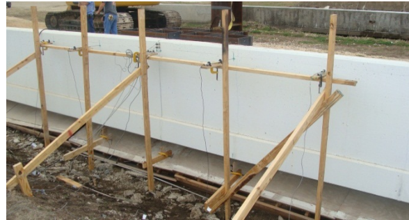
Fig. 4.15 Views of the test setup and sensor location at (a) front and (b) back of the barrier wall at interior load location
