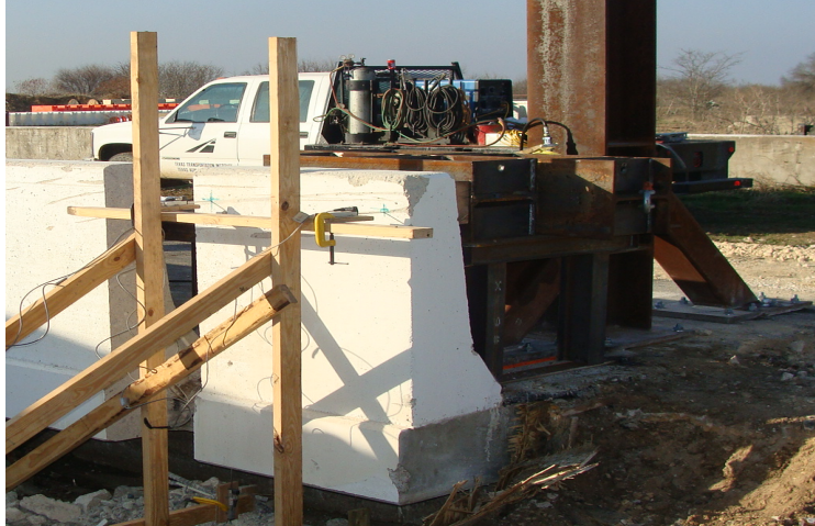
Fig. 4.9 Back view of Sample 2 showing 2 LVDTs at the top of the barrier oriented horizontally and 2 LVDTs at the bottom of the deck edge oriented vertically
