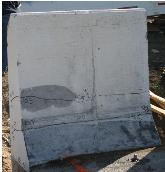
Fig. 4.20 Crack pattern in front of Sample 2
