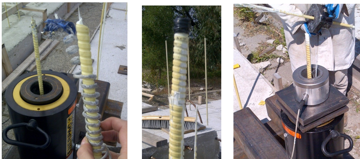
Fig. 3.10 Views of the bar rupture at grip location during pullout tests
