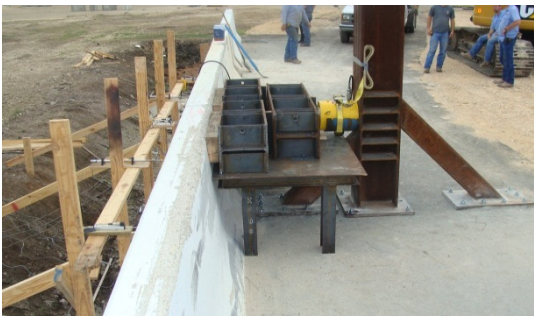
Fig. 4.15 Views of the test setup and sensor location at (a) front and (b) back of the barrier wall at interior load location
