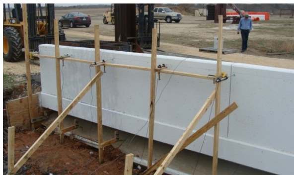
Fig. 4.16 Views of the test setup and sensor location at (a) front and (b) back of the barrier wall at end load location
