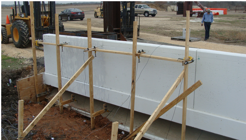
Fig. 4.10 View of back face of Sample 3 showing 5 LVDTs placed at the top of the wall and oriented horizontally and 3 LVDTs placed at the bottom of the deck edge and oriented vertically
