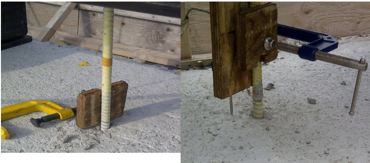
Fig. 3.12 Views of the bar pullout from the concrete slab after the test showing concrete shearing
