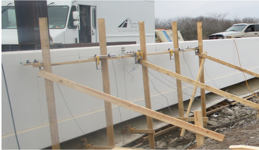
Fig. 4.11 View of back face of Sample 4 showing 5 LVDTs oriented horizontally at the top of the wall and 3 LVDTs oriented vertically at the bottom of the deck edge
