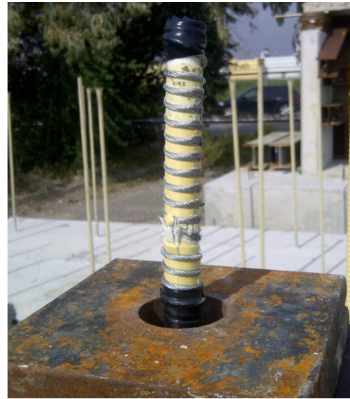
Fig. 3.8 Views of bar rupture at the location of the large grip
