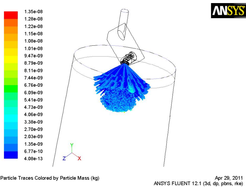
Figure 5.48: Particle Traces Colored by Particle Mass (kg) - The Rosin-Rammler Number of Classes Parameter
