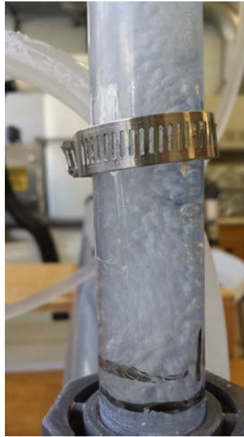
Figure 5-3. Air Entrainment in the Drop Shaft Due to a Free-falling Inflow
