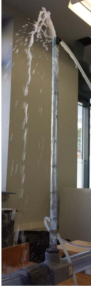
Figure 5-5. Geyser at the Drop Shaft
