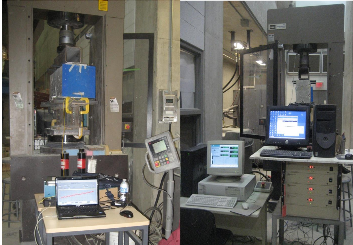
Figure 3-3 Typical beam under two point loading
