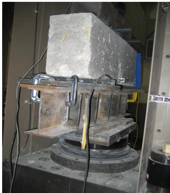
Figure 5-3 Typical beam under two point loading
