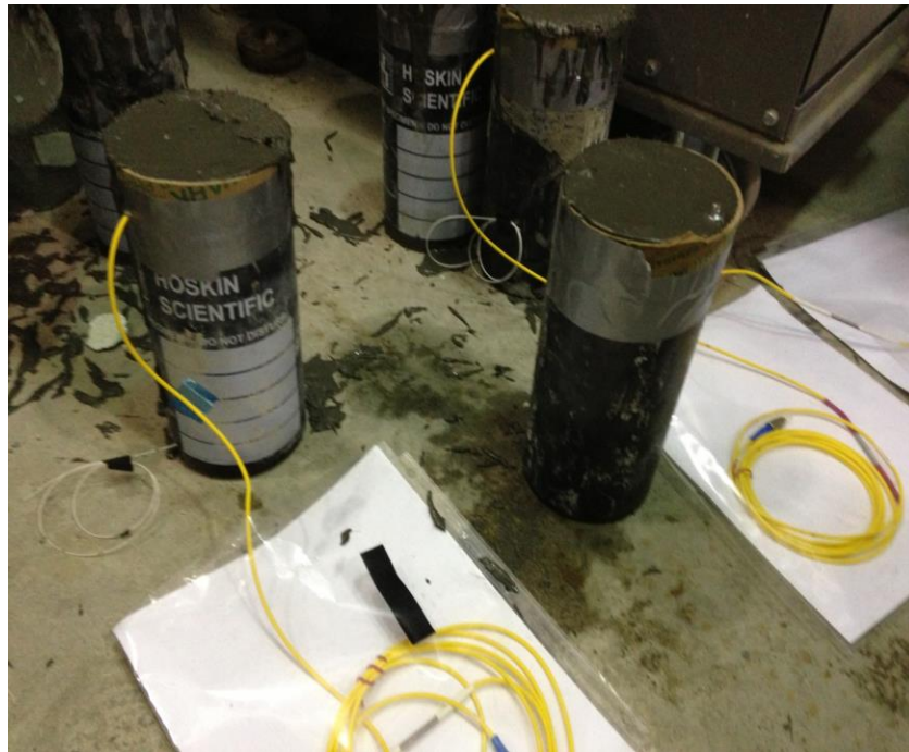
Figure 3-7 Cylinders after pouring concrete with embedded FBG sensor
