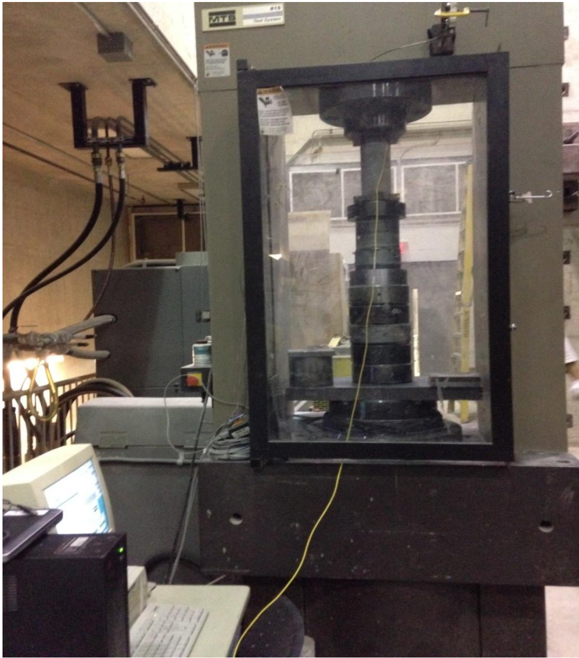
Figure 3-14 Modulus of elasticity test with embedded FBG sensor
