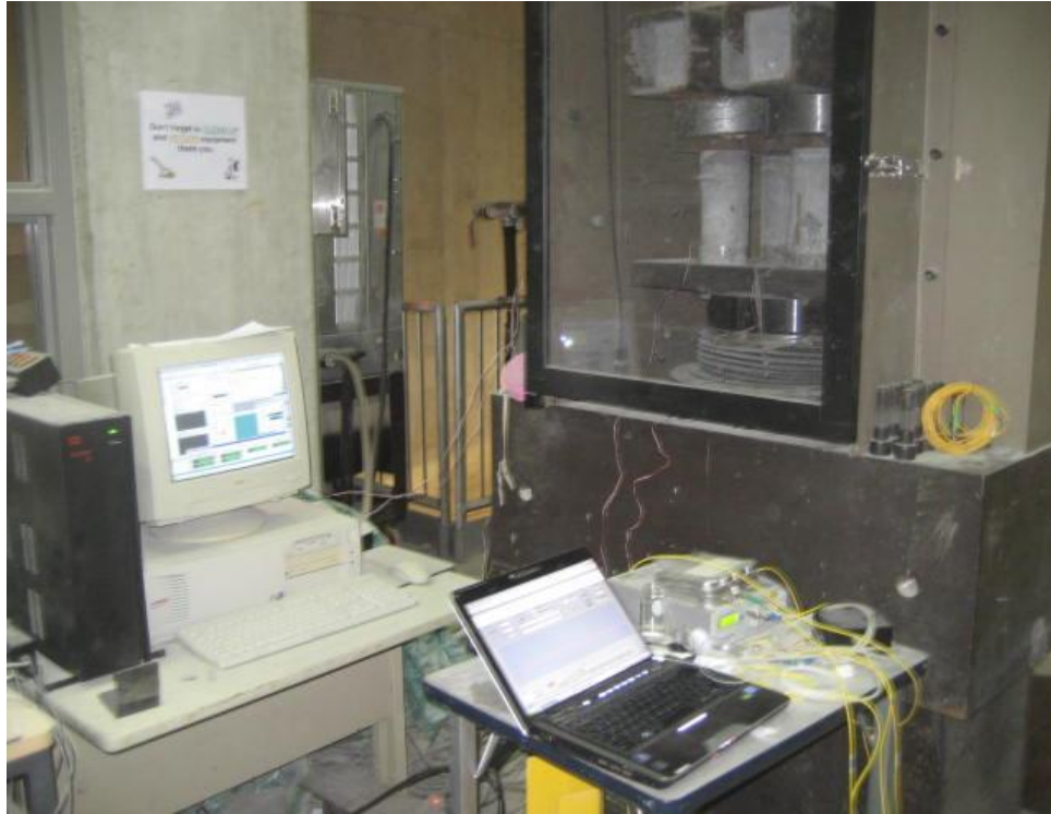
Figure 3-9 Experimental set up for creep test
