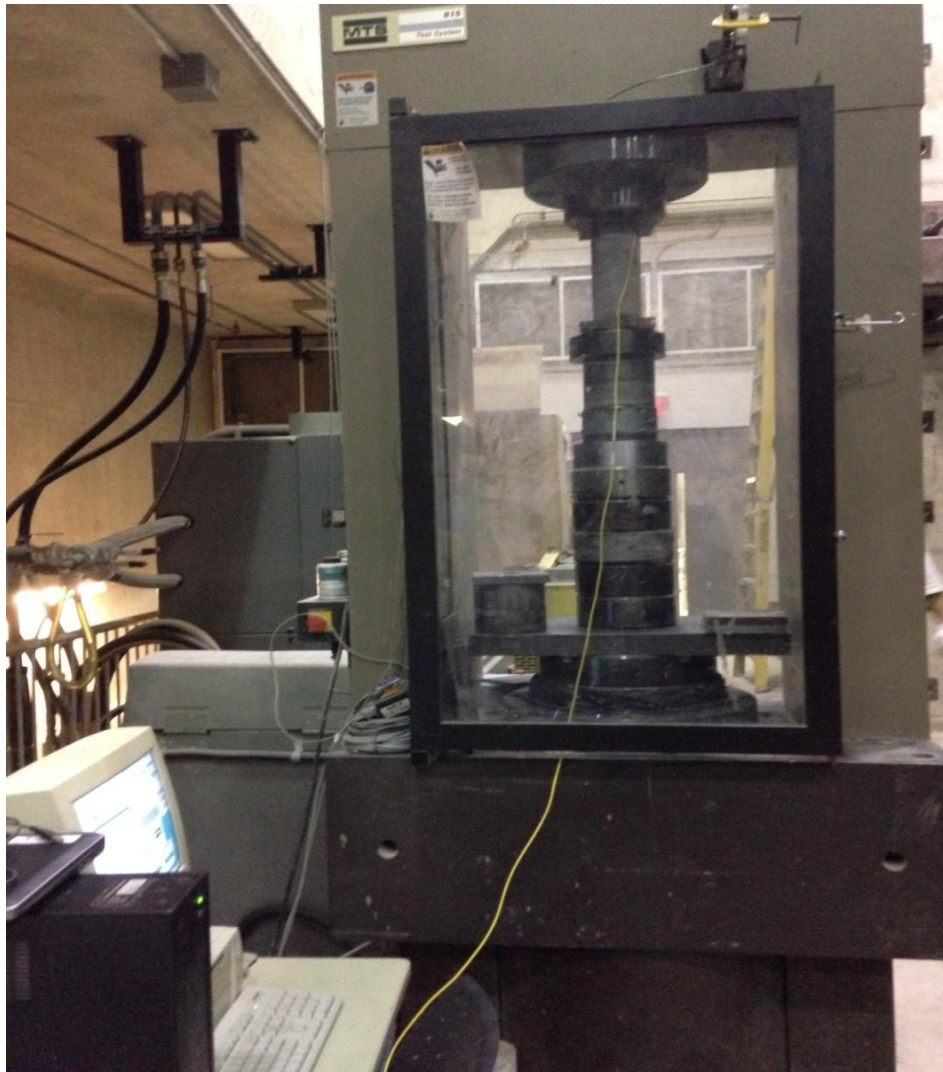
Figure 5-2 Modulus of Elasticity test with embedded FBG sensor
