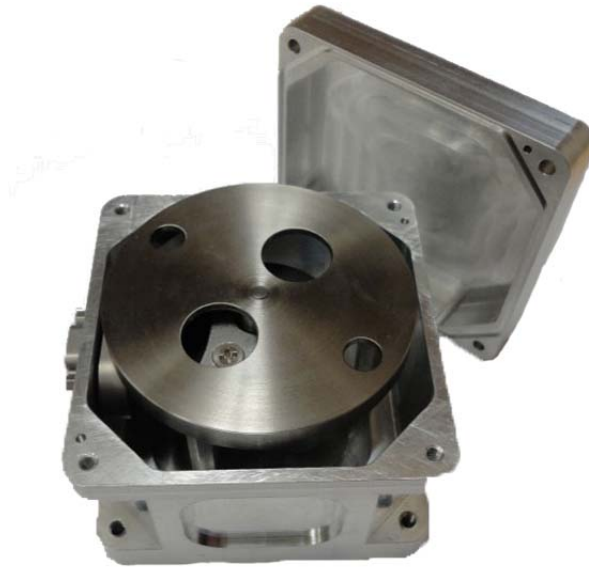
Figure 2.1 Reaction Wheel unit developed in the SSDC lab at Ryerson University
