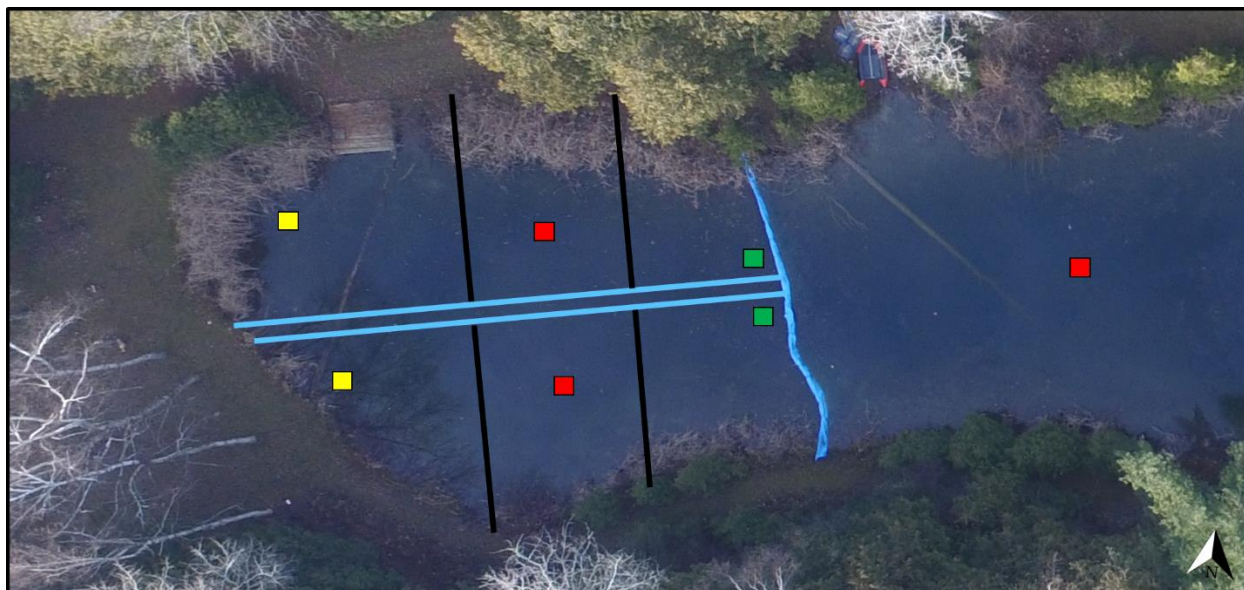
Figure 2.3: Location of temperature probes during experiment. Vertical thermistor chains were deployed in three locations: corner (green box), middle (red box), and shallow (yellow box) to represent different depths. Black lines represent the horizontal thermistor chains that were deployed along the sediment in east (right) and west (left) locations.
