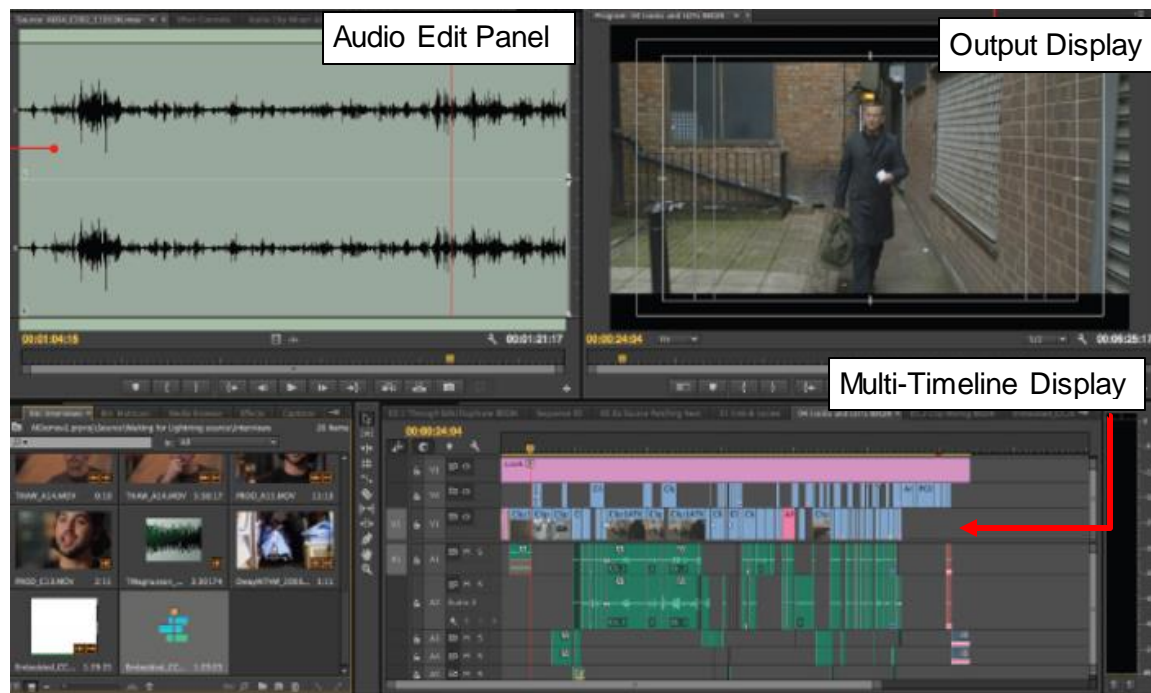
Figure 11: A screenshot of sample video editor, Adobe Premiere [56]. In the multi-timeline display panel, notice that the video clips are displayed with its thumbnails while audio samples are displayed with the frequency graph.
