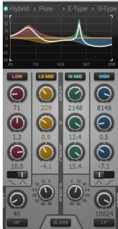
Figure 8: Screenshot from Cakewalk [52]: The user interface for EQ control with knob visual design. The knobs would increase/decrease the value when user turns clock-wise/counter clock-wise.
