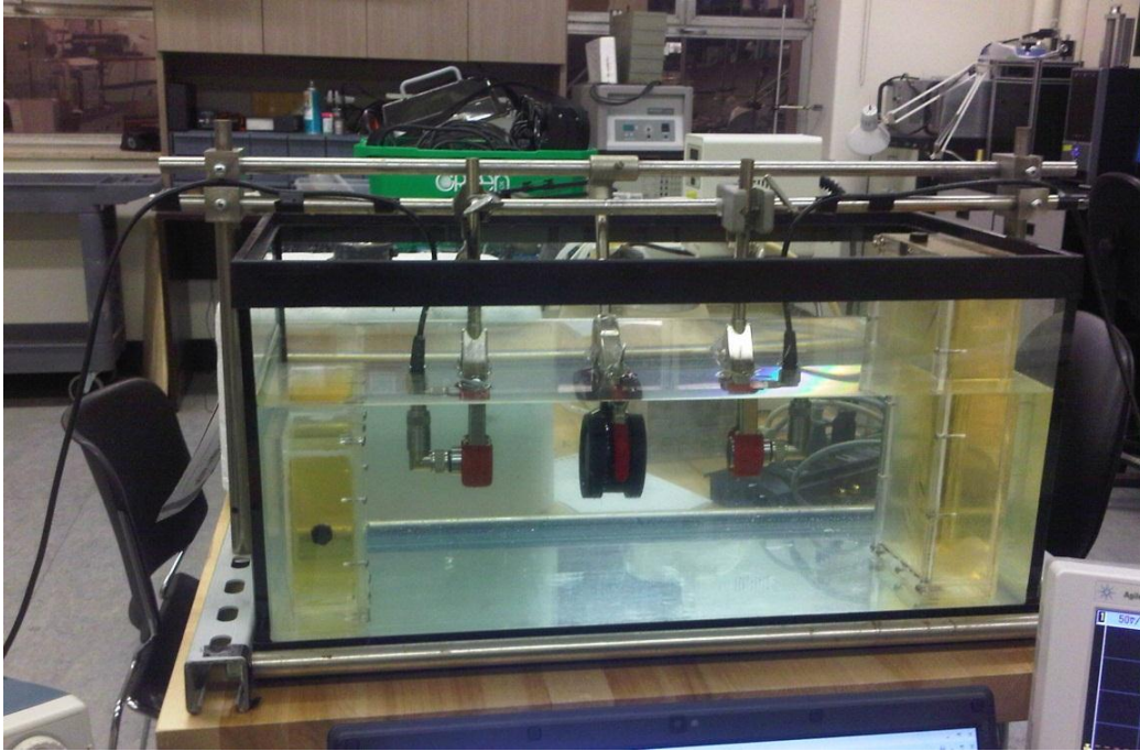
Figure 2-5 Insertion-loss acoustic attenuation measurement setup
