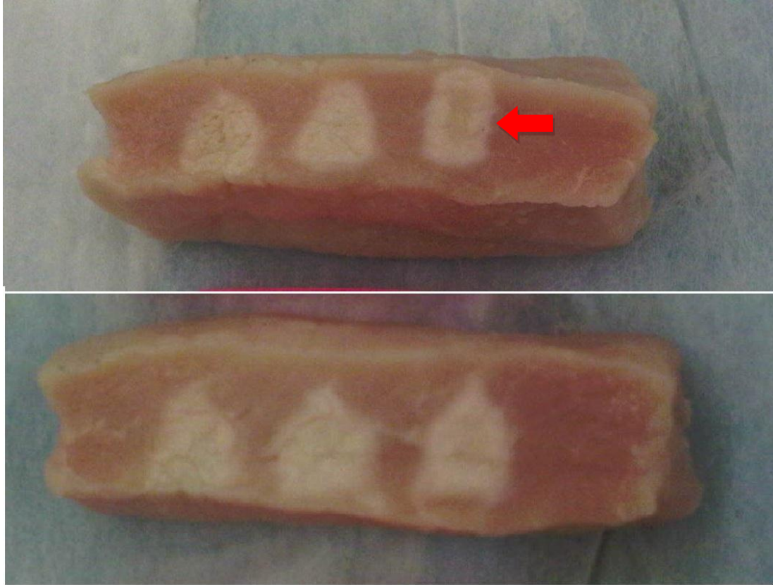
Figure 4-1 Lesions induced in degassed ex vivo porcine muscle tissues, where the input electric power of HIFU was 75 W, the duty cycle was 77%, and the average focal intensity at the HIFU treatment site was 801 W/cm 2 , for a total HIFU treatment time of 40 s
