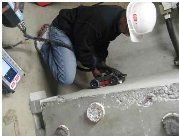
Fig. 4.12 Use of GPR to locate tendon duct centerline
