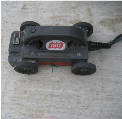
Fig. 4.65 GPR used to locate the tendon duct
