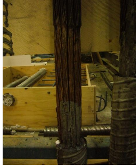
Fig. 3.34 View of the corroded 19/15 prestressing cable with the corroded portion and fully grouted duct at its bottom portion
