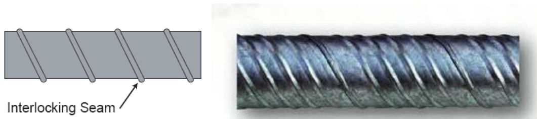
Fig. 3.62 Corrugated metal duct interlocking at seams
