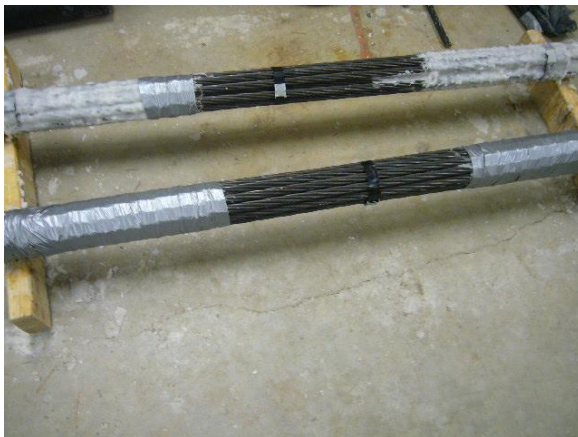
Fig. 3.54 Coating strands with candle wax (top); taping strands with electrical tape (bottom)
