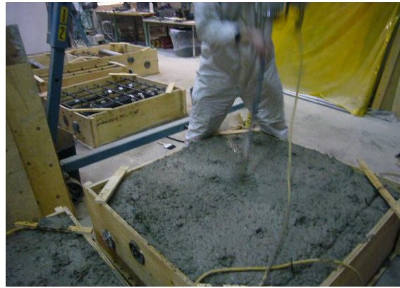
Fig. 3.67 vibrating concrete of specimen No.3
