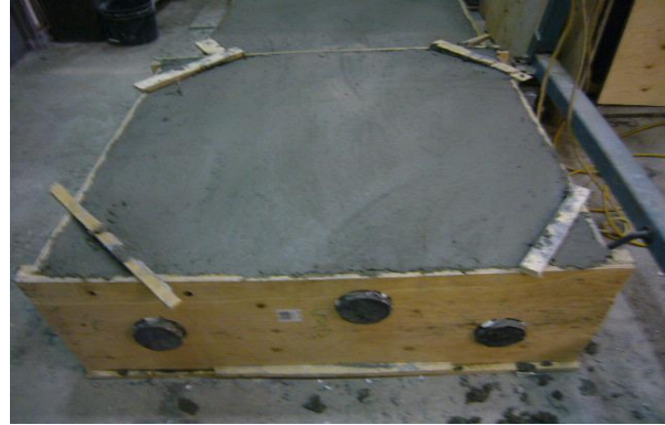
Fig. 3.25 View of specimen No. 3 after concrete casting
