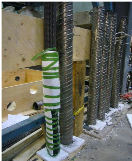
Fig. 3.27 View of the prestressing cable showing its middle portions with simulated void at its mid-length and partially grouted duct at its end
