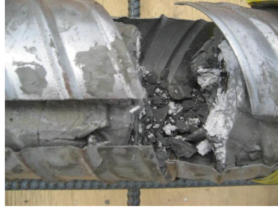
Fig. 3.50 View of complete wire break in the tendon at its mid-length
