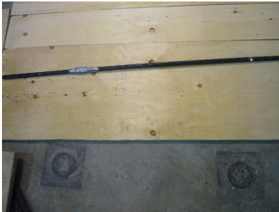
Fig. 3.39 View of the strand after introducing the artificial break and notch
