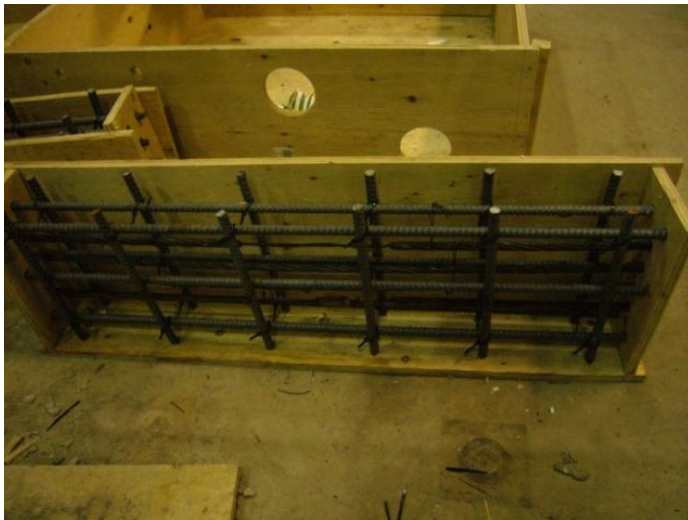
Fig. 3.42 View of specimens No. 7 before concrete casting
