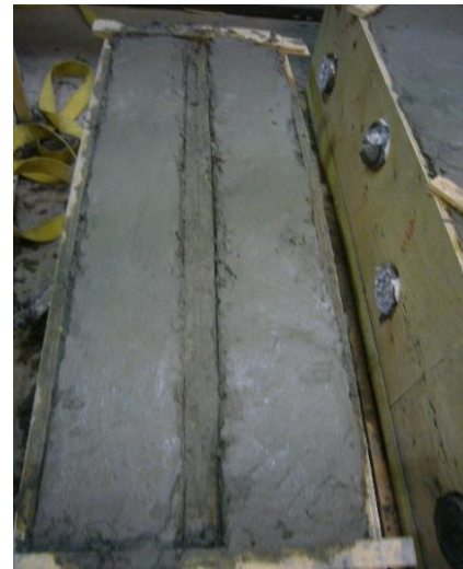
Fig. 3.43 View of Specimen No. 6&7 after casting concrete
