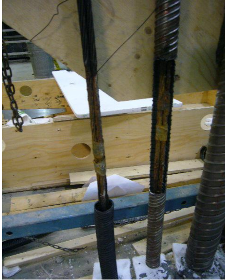
Fig. 3.33 View of the corroded 3/15 prestressing cable at its middle third portion along with partial grouting
