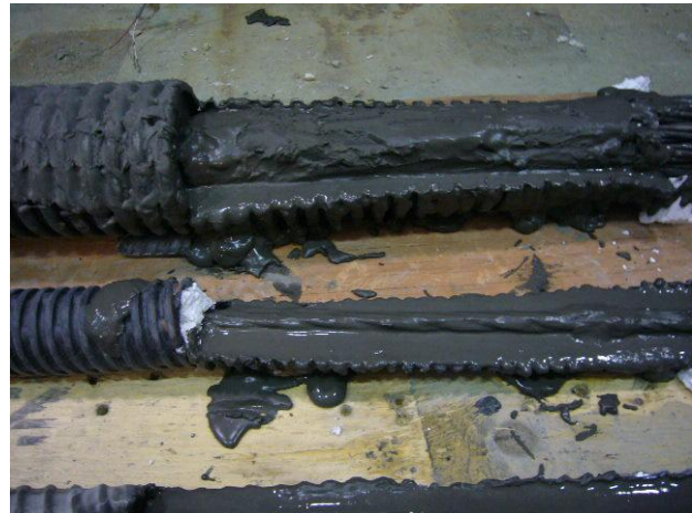
Fig. 3.29 Views of partial grouting of 100 mm and 50 mm plastic ducts
