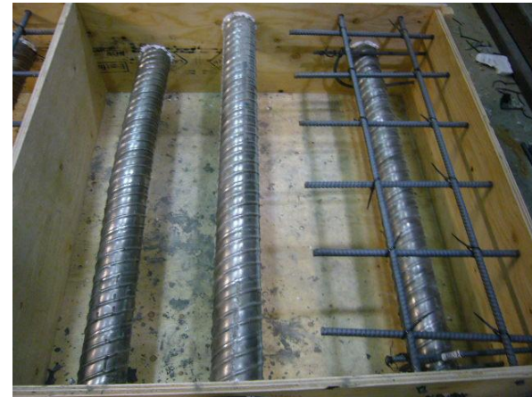
Fig. 3.8 View of the ducts and steel of specimen No.1 before concrete casting
