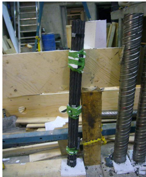
Fig. 3.14 View of simulated voids inside the duct by wrapping the prestressing cable with styrofoam
