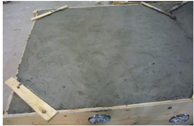
Fig. 3.16 View of specimen No. 2 after concrete casting
