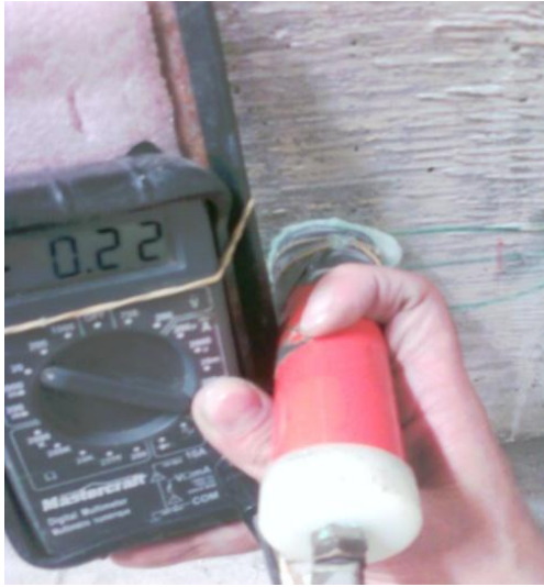
Fig. 4.61 half-cell potential reading obtained from specimen No. 3 (Fig. 3.18) in the region of active corrosion in strands
