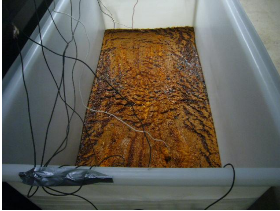
Fig. 3.56 Corrosion product of strands
