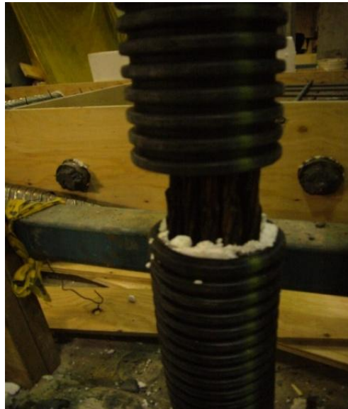
Fig. 3.35 View of how voids are introduced in plastic duct using Styrofoam infill
