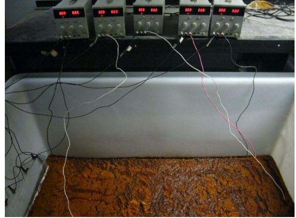
Fig. 3.57 Connecting anodic side of power suppliers to the strands and cathodic side to the steel mesh with a maximum current of 3 Ampere
