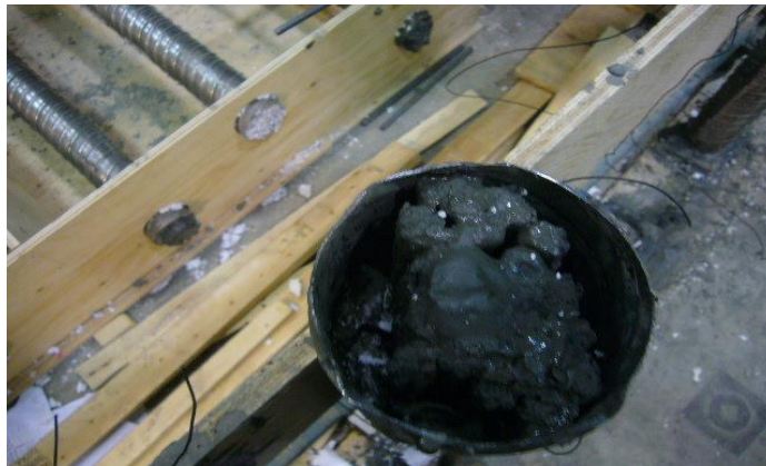
Fig. 3.23 Introducing simulated void of 60 mm length in the straight tendon near its end
