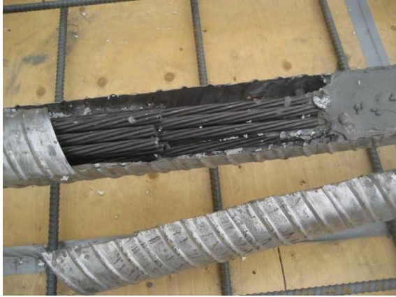
Fig. 3.49 View of the 100-m duct showing air void and wire breaks (section C-C)
