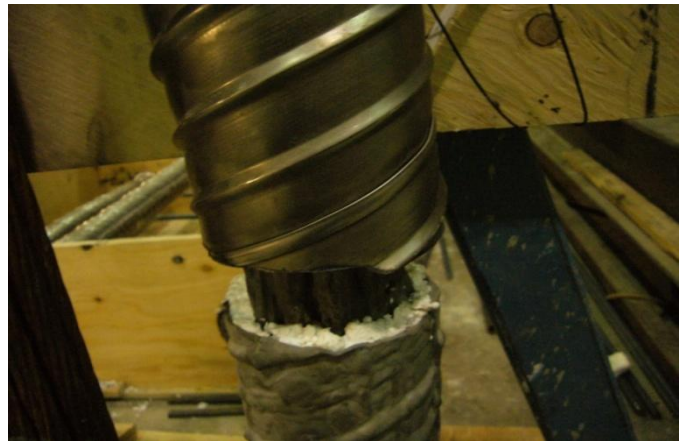
Fig. 3.22 Introducing simulated void of 60 mm length in the curved tendon using Styrofoam infill
