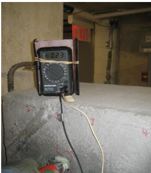
Fig. 4.63 Half-cell potential test on a wet concrete surface showing more negative voltage
