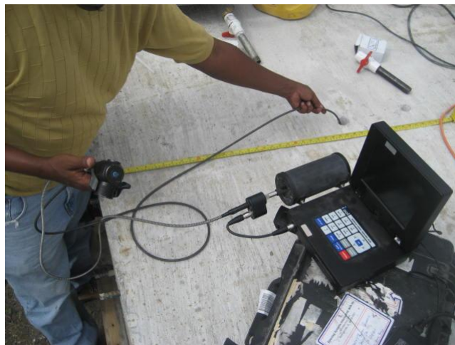
Fig. 4.72b Borescope recording the inside condition of the tendon duct
