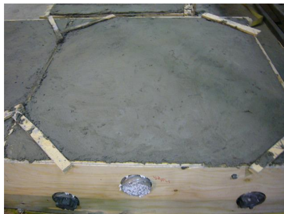
Fig. 3.9 View of specimen No.1 after concrete casting
