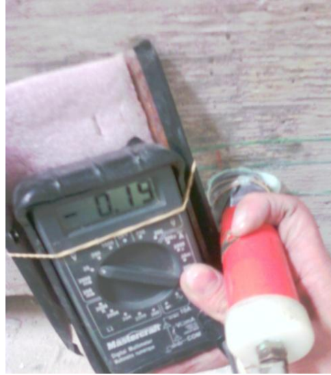
Fig. 4.62 Half-cell potential obtained from specimen No. 3 (Fig 3.18) at a point located below the region of active corrosion
