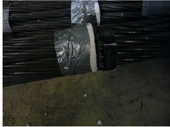
Fig. 3.6 View of the prestressing cable showing simulated break at its mid-length
