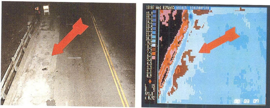
Fig. 2.16 Visual and thermal images of powdery concrete, Martin Luther King Bridge- St. Louis (Malhotra et al., 2004)
