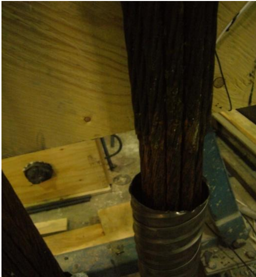
Fig. 3.21 View of the corroded cable over 300 mm length
