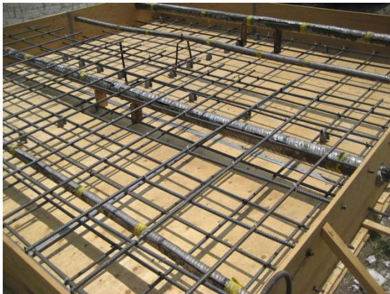
Fig. 3.51 View of specimen No. 8 before pouring concrete
