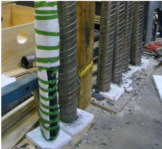
Fig. 3.64 Use of Styrofoam to form voids
