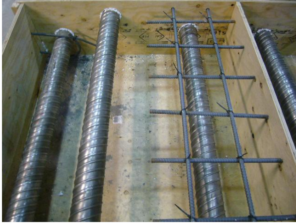
Fig. 3.66 view of tendon strands and rebar Placement in specimen No.2
