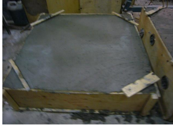
Fig. 3.37 view of specimen No. 5 after concrete casting
