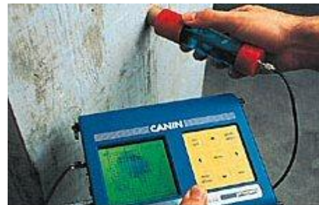
Fig. 2.6 Schematic diagram the Half- cell potential device (Adapted from Malhotra, 2004)
