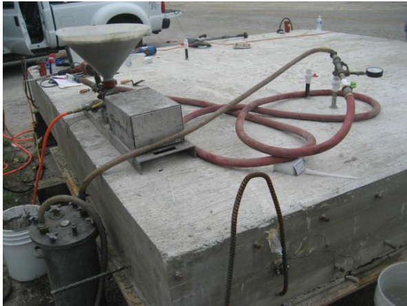
Fig. 4.75 Vacuum grouting of voided duct
