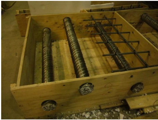
Fig. 3.15 View of specimen No. 2 before concrete casting
