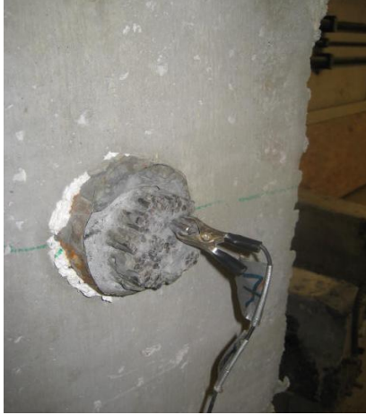
Fig.4.42 Electrical connection to an exposed wire strand
