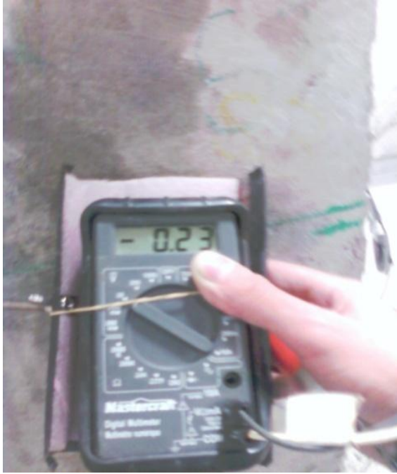
Fig. 4.57 Half-cell potential reading obtained from specimen No. 3 in corroded region where concrete cover to tendon is 50 mm
