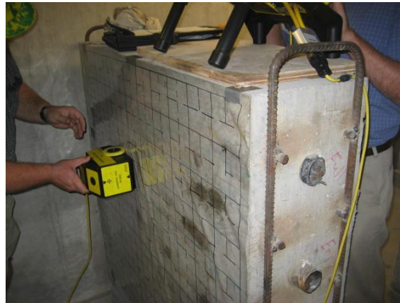
Fig. 4.7 performing GPR test in gird line of specimen No. 5 to obtain 3D-image
