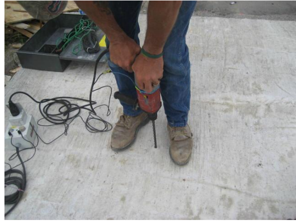
Fig. 4.69 Drilling a small diameter hole to verify presence of void
