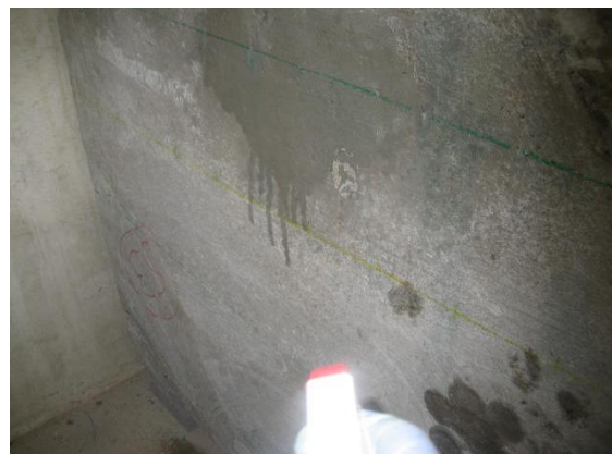
Fig.4.40 Cleaning strand using chisel Fig. 4.41 Watering the concrete surface prior to testing
