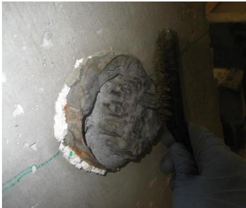
Fig.4.40 Cleaning strand using chisel Fig. 4.41 Watering the concrete surface prior to testing
