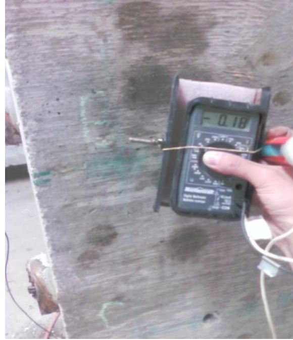
Fig. 4.58 Half-cell potential reading obtained from specimen No. 3 in corroded region where concrete cover to tendon is 250 mm (on the other side of the tendon)
