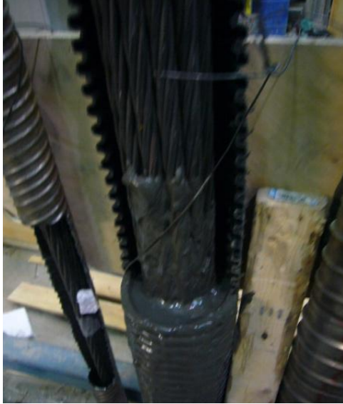
Fig. 3.28 View of the duct and the prestressing cable during grouting
