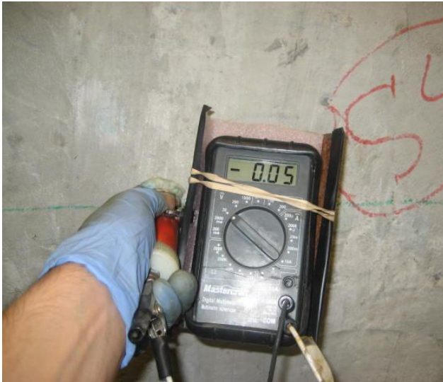
Fig. 4.59 Poor connection to steel strand in which the strand was not properly cleaned
