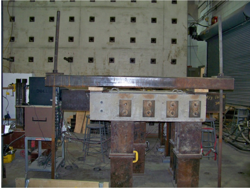
Figure 3.11: South view of the setup - RC beam on roller supports
