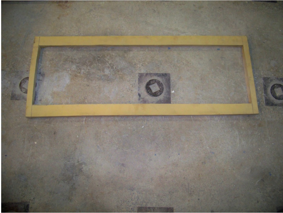
Figure 3.14: Gum Rubber used between the chamber and concrete surface
