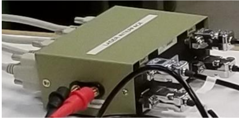
Figure 6: Laser Interface illustrating the power input terminals on the left side
