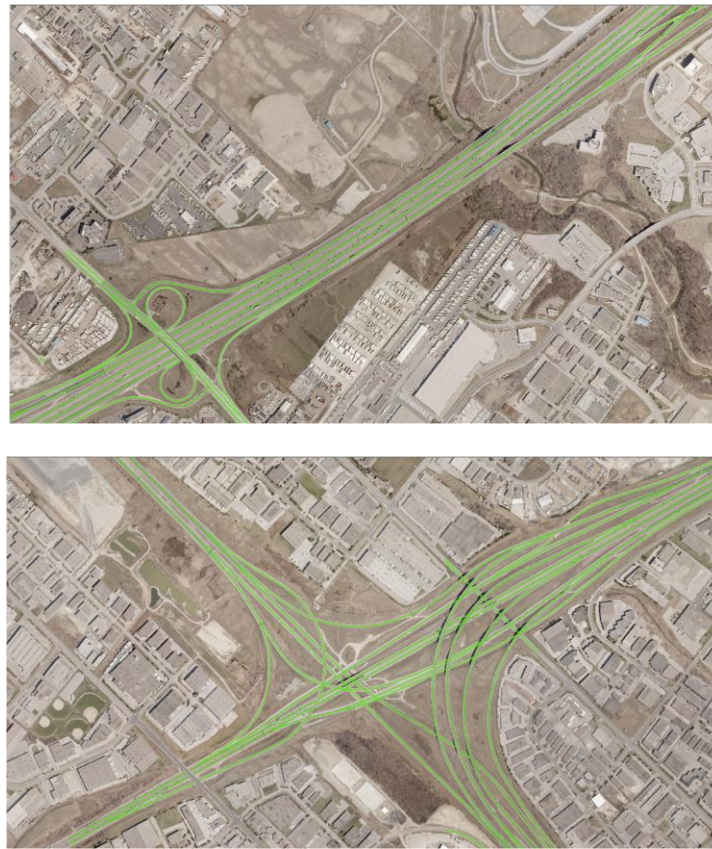
Figure 5.8: MTO highway horizontal alignment data (green) overlaid with 15-cm resolution aerial orthophoto.
