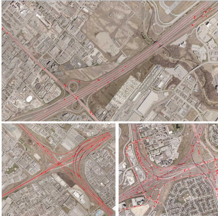
Figure 5.6: Visual inspection of extracted road network with high-resolution aerial orthophoto image.
