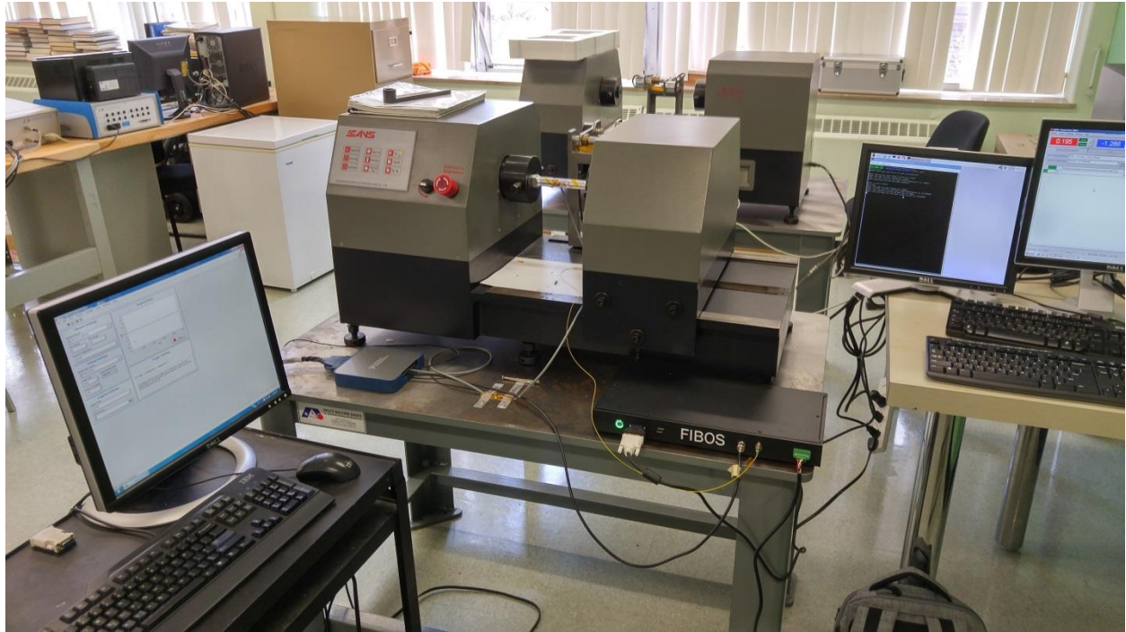
Figure 21 - Torque Experiment Setup. The aluminum torsion rod with both the fiber optic sensor and foil strain gauges is mounted in the SANS CTT202 Torsion Test machine.
