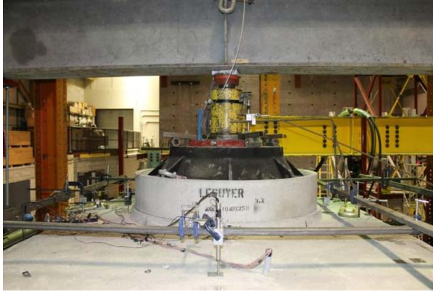
Figure 3.11: Details of load cell and load plate assembly (D'Amours, et al. , 2013)
