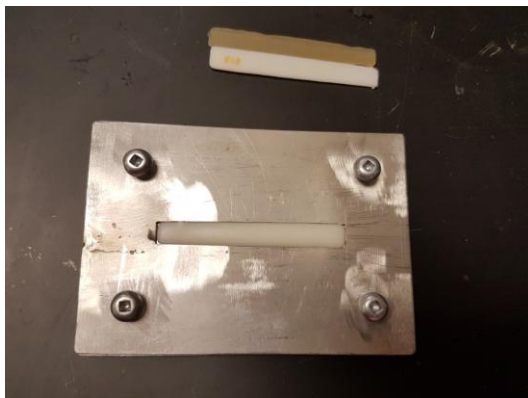
Fig. 3.3 Handmade stainless steel mold used for preparing tensile samples of dimensions [1mm (t) \times 1cm (w) \times 10cm]; yellowish sample is TBPU-3 while the white samples are TBPU-3 reinforced BCNW composites.
