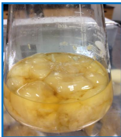
Fig. 3.1 Lab photo showing BC pellicles during their production from shake culture.
