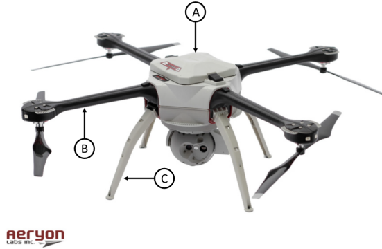
Figure 3.3: Aeryon Skyranger with labeled components: A) centre body B) rotor arms C) landing gear[1].
