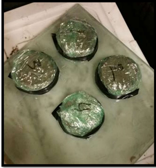
Figure 3-17: Sealed cement-treated samples before placing in the curing chamber
