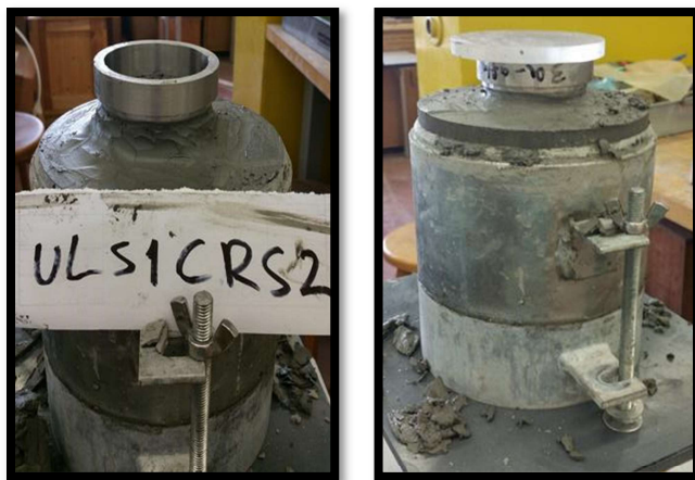
Figure 3-16: Inserting leached samples into CRS rings
