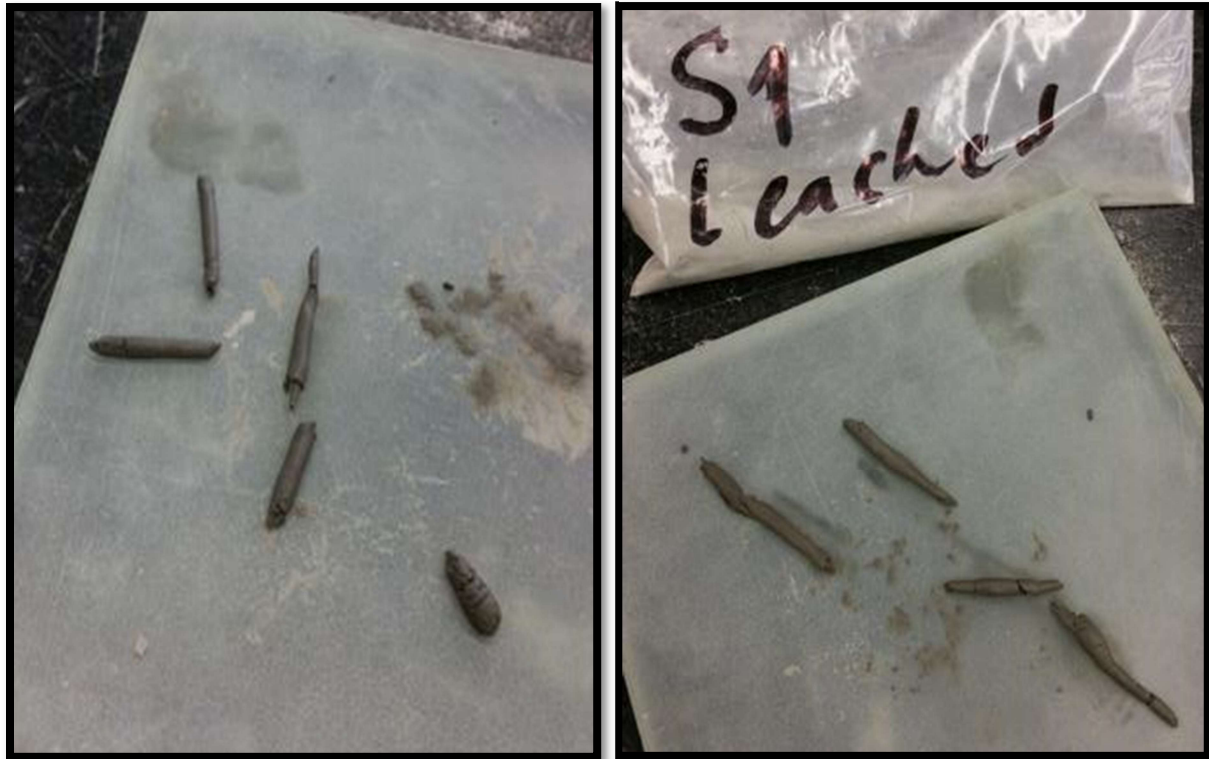
Figure 3-1: Sample of clay at plastic limit
