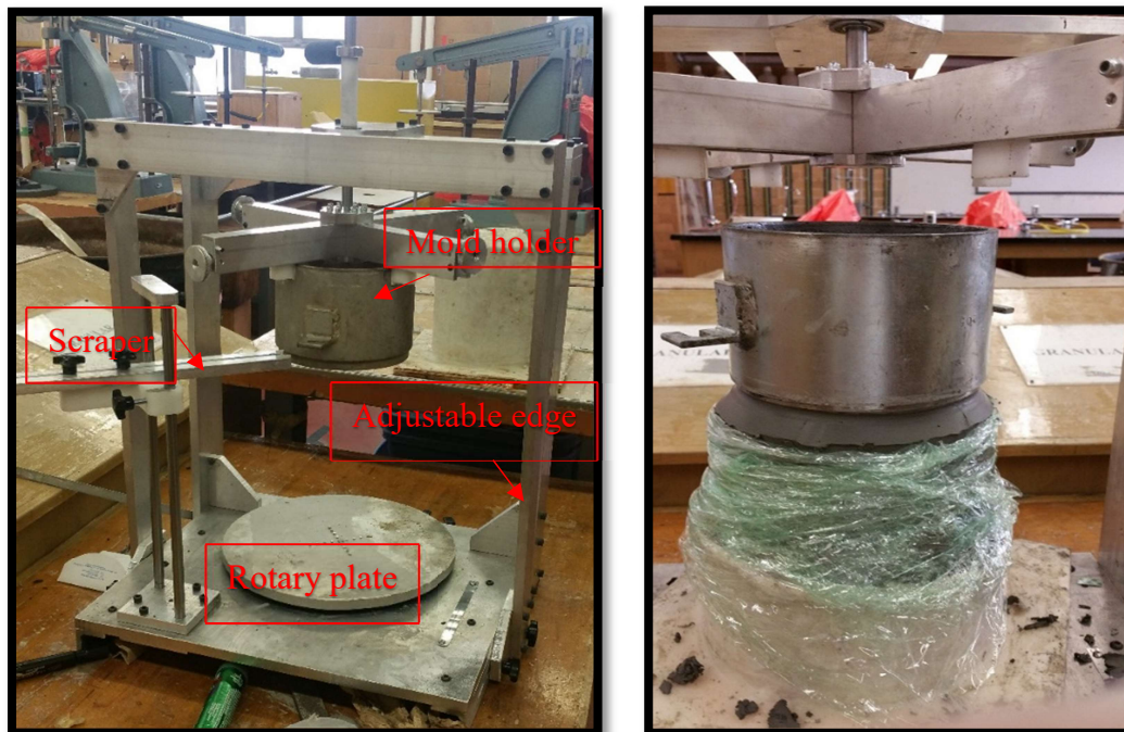
Figure 3-8: View of the cutting machine (right), & a clay sample halfway inserted into the leaching mould (left)
