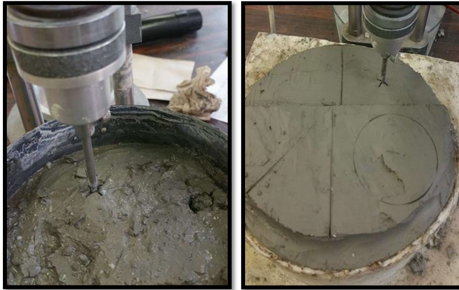
Figure 3-5: Mini vane shear tests on leached (left) and natural (right) Champlain Sea clay
