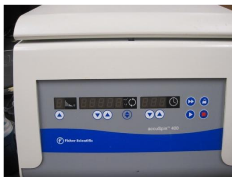
Figure 15 Centrifuge applied to separate wheat straw solids from liquid: model # accuSpin 400; manufactured by Fisher Scientific
