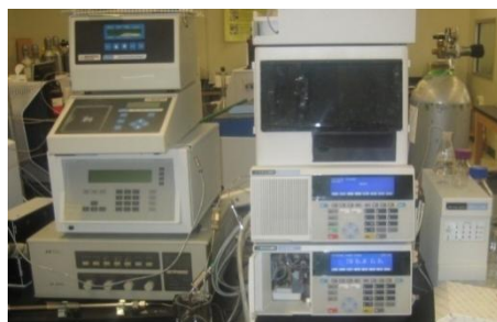
Figure 16 HPLC used to measure sugars, butyric acid, and butanol Refractive index: model # HP 1047A; manufactured by Hewlett Packard HPLC: model # 600; manufactured by Perkin Elmer
