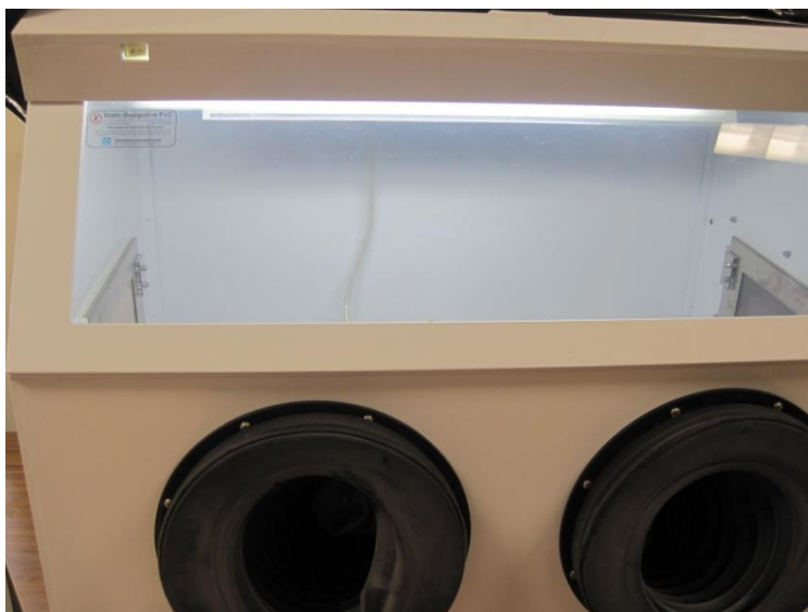
Figure 14 Glove box used to create an anaerobic environment: model # 1681-29C-EX-001; series # 100; manufactured by Terra Universal
