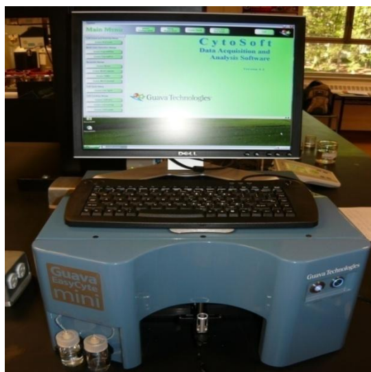
Figure 17 Flow cytometer applied to measure cell concentration: model # GTI_2800080228; manufactured by Guava Technologies
