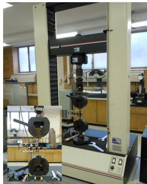
Figure 3.3- Test setup for tensile testing of steel sheeting coupon samples
