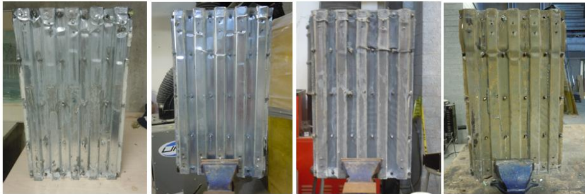
Figure 5.14- UHPC double skin composite wall failure (back view) for control, 400°C, 600°C, and 800°C
