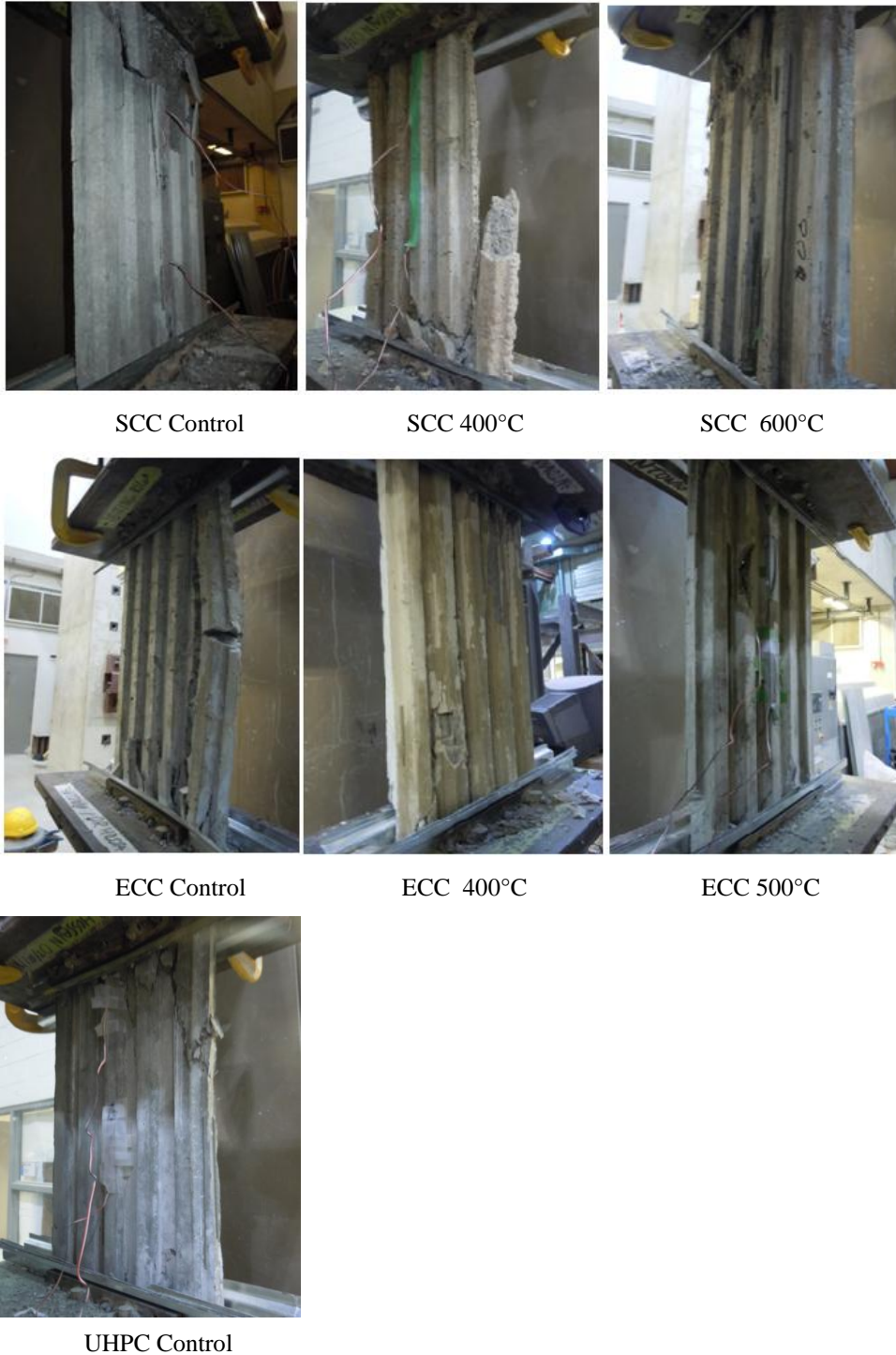
Figure 4.22- Failure modes of profiled concrete walls
