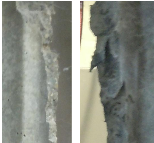
Figure 4.20- Failure in SCC (left) and ECC (right) walls ambient temperature
