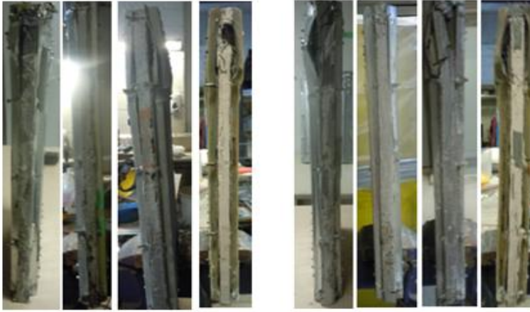
Figure 5.17- UHPC double skin composite wall failure (left and right view) for control, 400°C, 600°C, and 800°C
