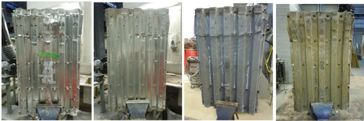
Figure 5.12- SCC double skin composite wall failure (back view) for control, 400°C, 600°C, and 800°C
