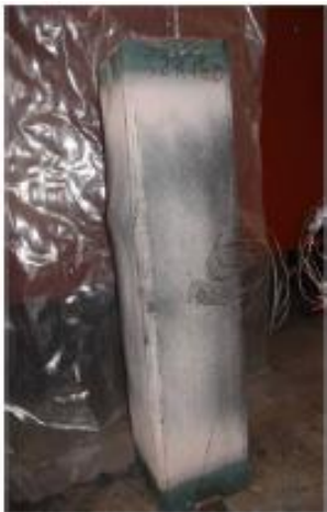
Figure 2.8- Failure mode of short CFST columns (Lu et al. 2009)
