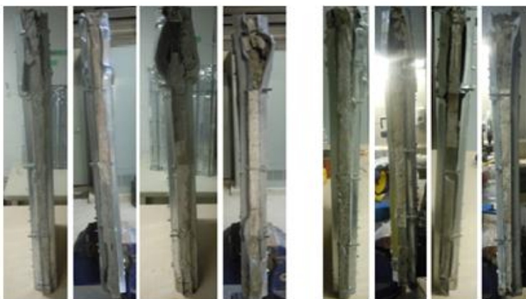
Figure 5.16- ECC double skin composite wall failure (left and right view) for control, 300°C, 400°C, and 500°C
