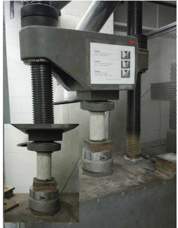
Figure 3.13- Test setup for compressive strength of concrete cylinders
