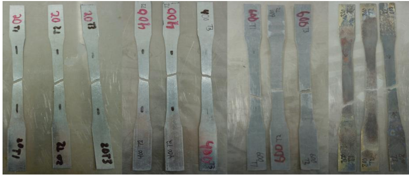
Figure 3.7- Failure Mode in Steel Sheeting Coupon Samples (20°C to 800°C)
