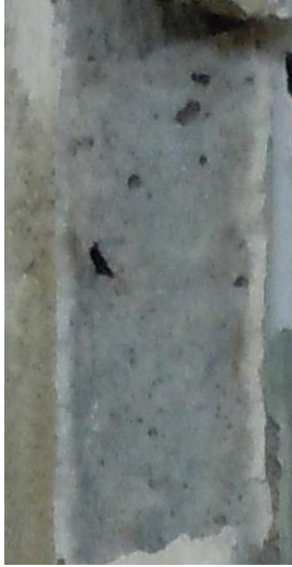
Figure 3.22- Voids present in ECC after melting of PVA fibers
