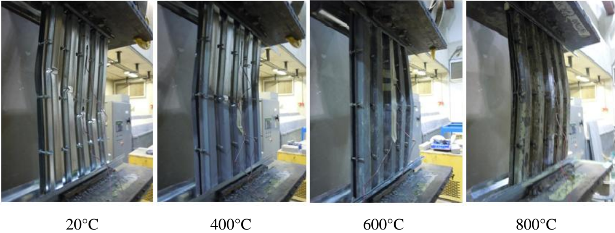
Figure 4.6- SSWs after failure (left view) for control, 400°C, 600°C and 800°C
