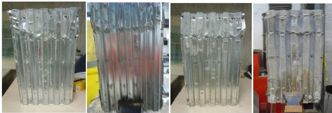
Figure 5.13- ECC double skin composite wall failure (back view) for control, 300°C, 400°C, and 500°C
