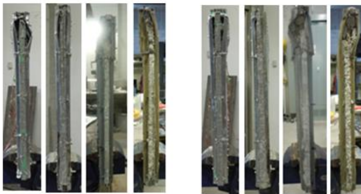
Figure 5.15- SCC double skin composite wall failure (left and right view) for control, 400°C, 600°C, and 800°C
