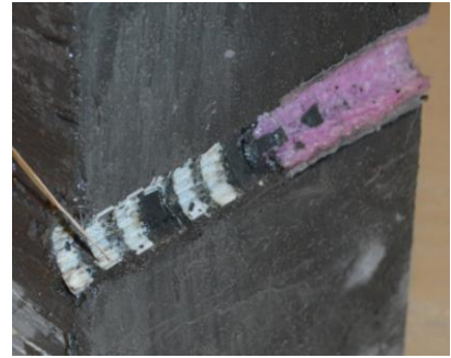
f) Close-up view of sheared ribs
