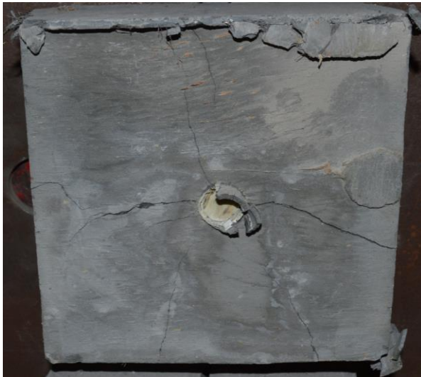
c) Splitting Cracks at free end of the UHPC block after bar pullout
