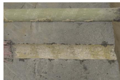
h. Interlaminar shear failure of the coating and shear-off of sand coating from bar surface
