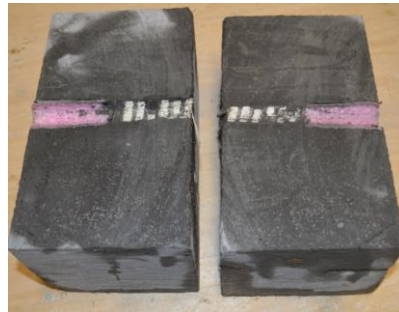
e) Section cut in the UHPC cube at bar location
