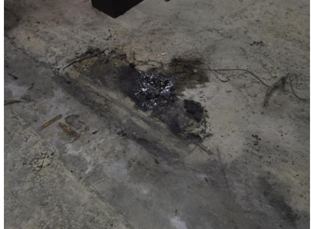
b) Close-up view for the punching shear failure at the wheel footprint
