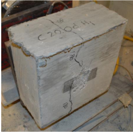
a. Block with centric headed-end bar showing splitting cracks
