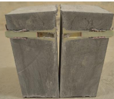
d. Bar pull-through failure and slippage from anchorage head
