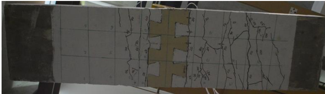
c) Crack pattern at the bottom of the slab
