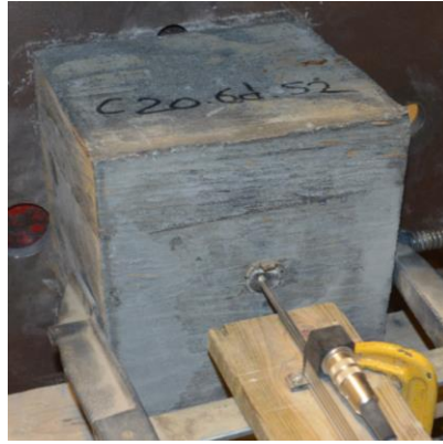
b. Decrease of projecting bar length during test
