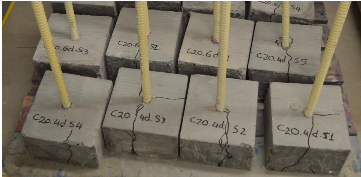
Figure 2.7. Views of splitting cracks after pullout test for the 20M ribbed-surface GFRP bars with embedment length of 4 and 6 times the bar diameters
