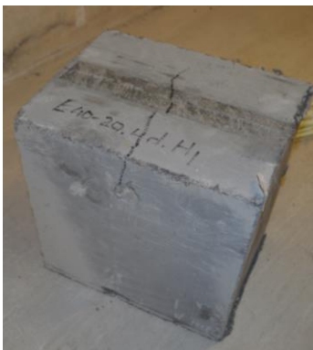
f. Block with headed-end bar at 40 mm concrete cover showing side crack
