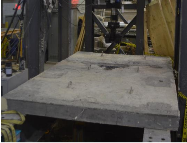
a) Top view showing punching shear failure at wheel footprint
