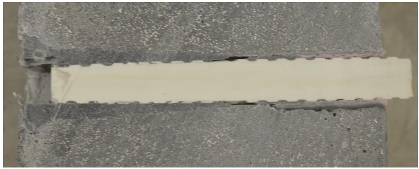
e) Close-up view for the bar slippage from its black head
