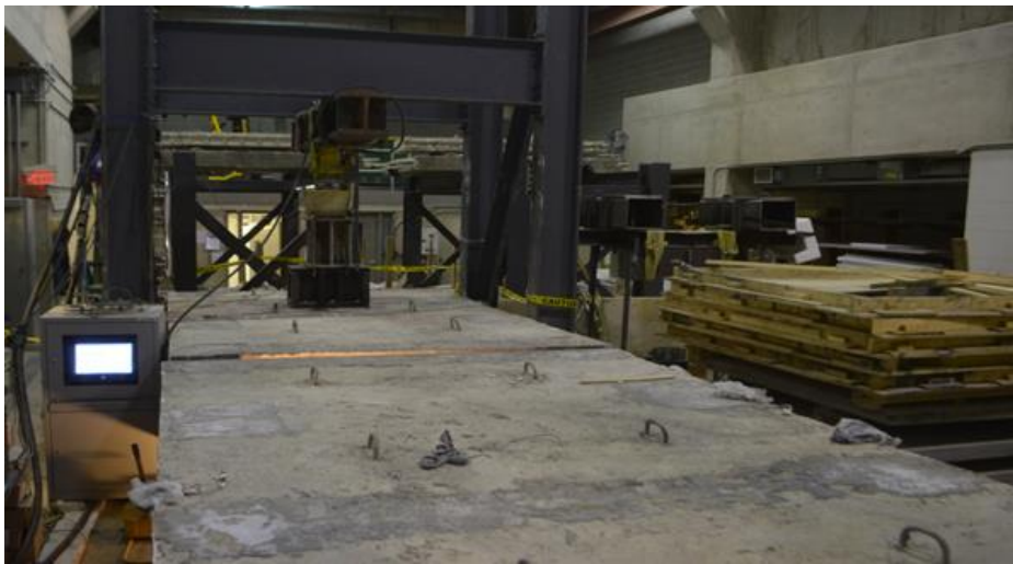
a) Slab-girder bridge system during static load test
