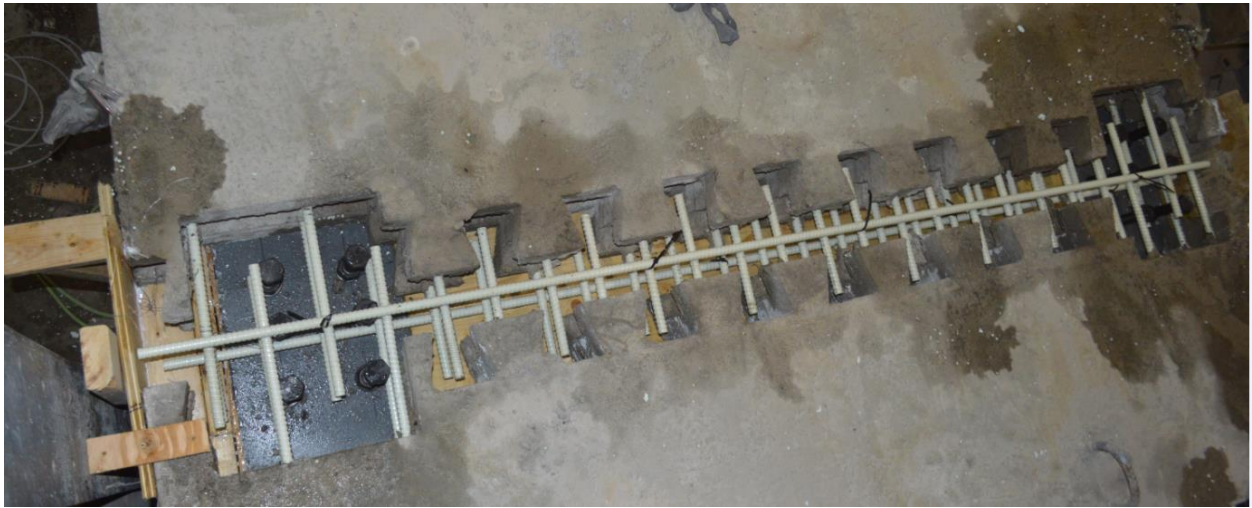
Figure 5.43 Close-up view for the zigzag joint before casting
