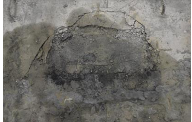
b) Close-up view for the punching shear failure at the wheel footprint
