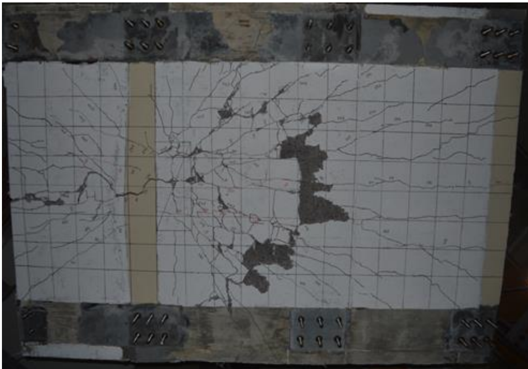
c) Bottom view showing crack pattern
