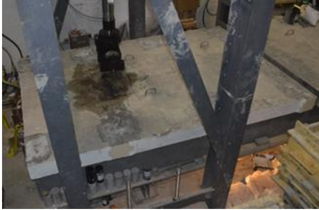
a) Top view showing punching shear failure at wheel footprint
