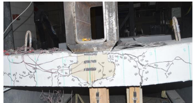
b) Crack pattern at the joint region
