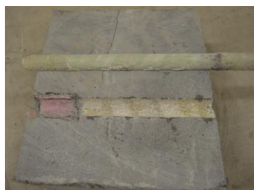
h. Interlaminar shear failure of the coating and shear-off of sand coating from bar surface
