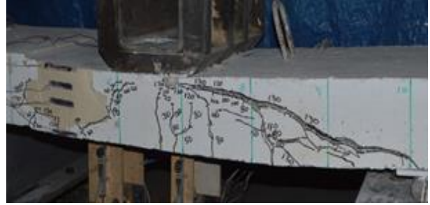
b) Crack pattern at the joint region showing major flexural-shear crack
