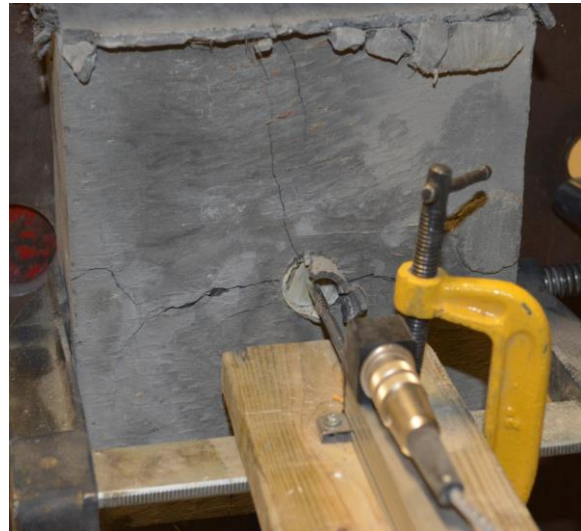
d) Close-up view of the bar pullout and splitting cracks
