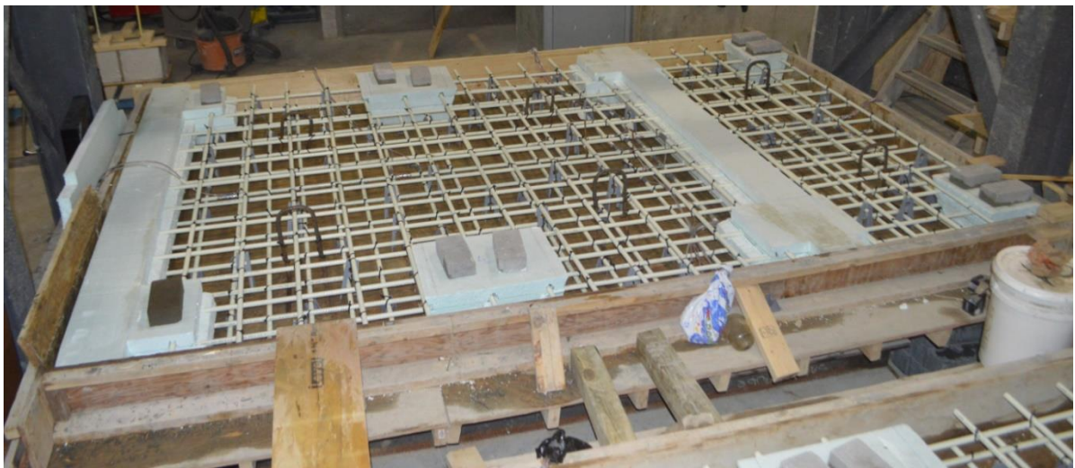
c) View of GFRP bars and styrofoam to form the joints
