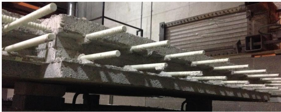
c) Photo of C-joint with projecting GFRP bars
