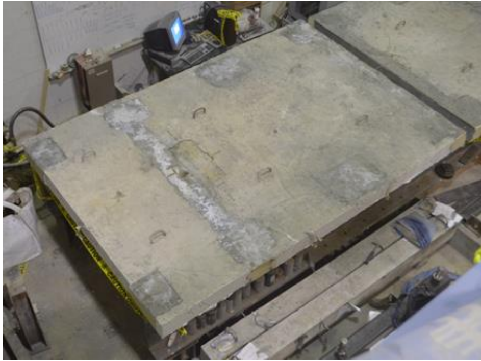
a) Top view of the slab showing punching shear failure at the footprint of the wheel load
