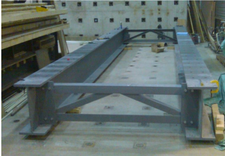
Figure 5.11 View of the steel twin-girder system supporting the precast FDDPs
