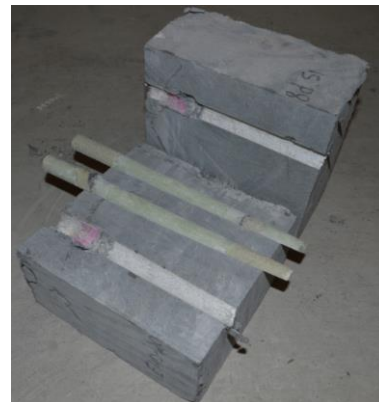
e. View of interlaminar shear failure of the sand coating along with shearing-off of the coating from bar surface
