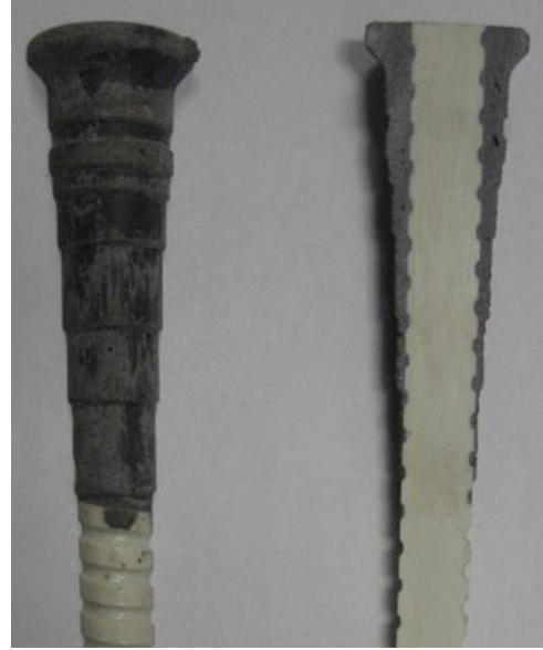
c) Sliced head-end bar showing ribs interacting with bar head material
