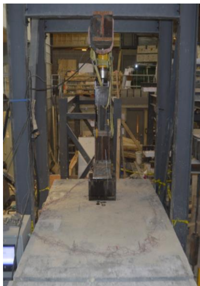
a) Slab-girder bridge system during monotonic loading
