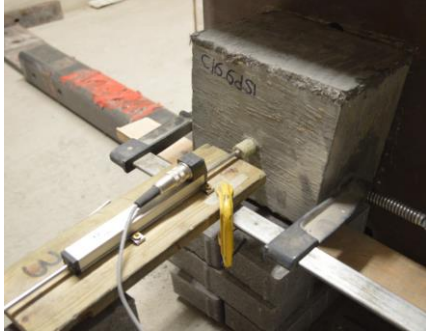
a. Bar projecting length at the free end before test
