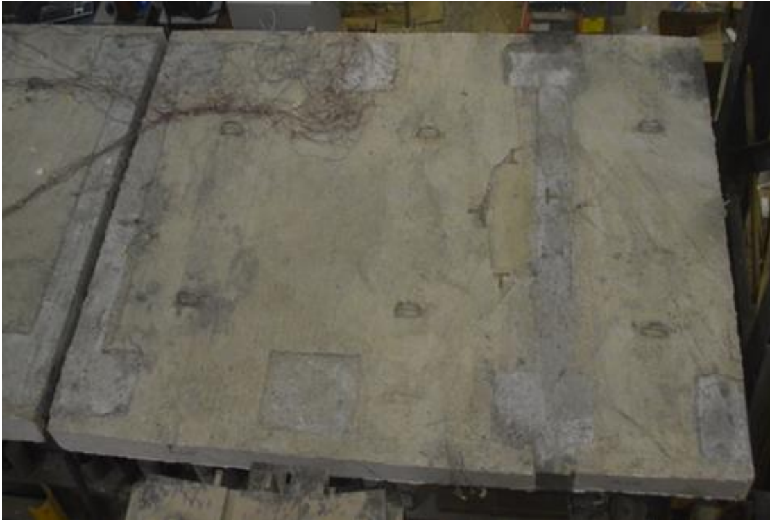
a) Top view of the slab showing punching shear failure
