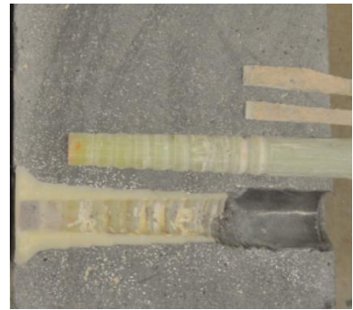
e. Close-up of shearing the grooves along the bar embedded length in the head
