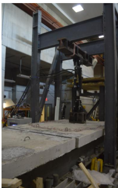
a) Slab-girder bridge system during CAF and VAF loading
