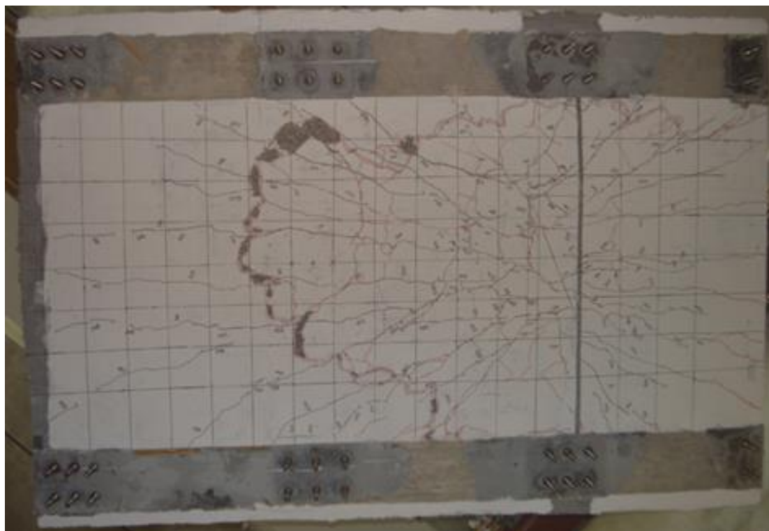
b) Bottom view of the slab showing crack pattern after failure
