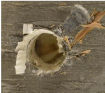
d) Close-up view of bar slip at free end
