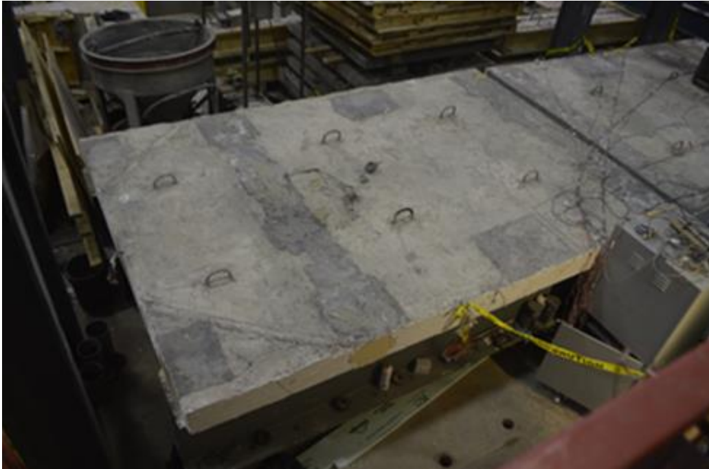
a) Top view of the slab showing punching shear failure at the footprint of the wheel load
