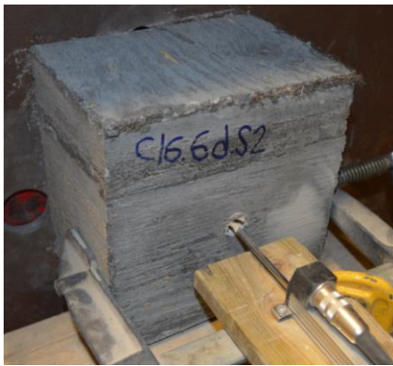
d. Block view at failure shown projecting bar end slipped inside the block at failure
