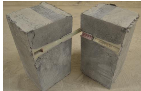
f. Section cut for headed bar with 60 mm concrete cover showing bar slippage from head and pull-through failure
