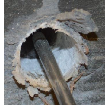
c. Close-up view of the concrete hole at block free end sand-coating left behind along the perimeter of the hole
