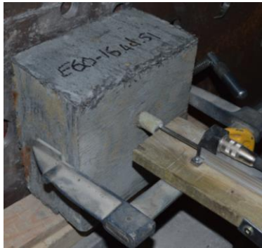
d. Bar projecting length, with 60 mm concrete cover, at the free end before test
