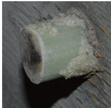
e. Peeling-off failure of the sand coating at failure
