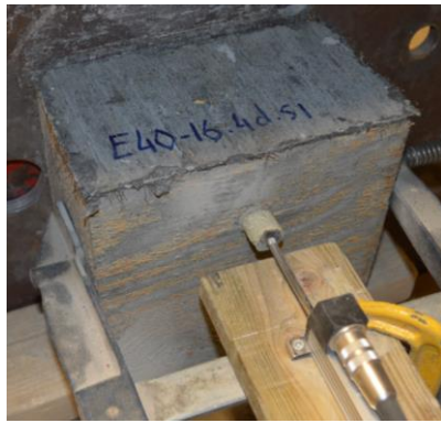
a. Bar projecting length, with 40 mm concrete cover, at the free end before test
