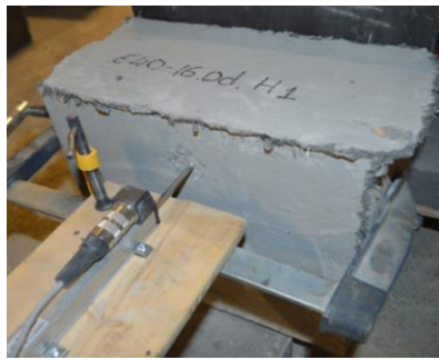
c. View of front and back face of block for GFRP headed bar with 40 mm concrete cover
