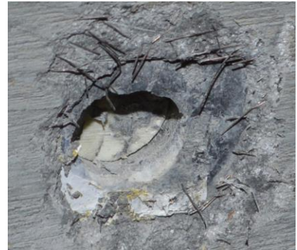
c) Close-up view of bar slip at its end
