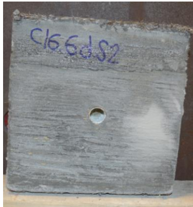
e. View of the block free face showing the bar end went deeply in the hole
