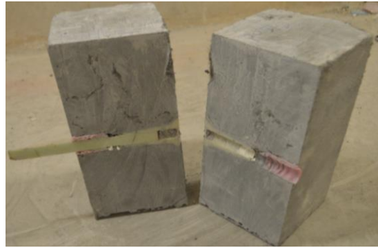
b. Centric bar slippage from the anchorage head
