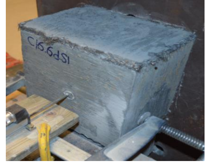
c. Projecting bar end became flush with the block free-end face during test
