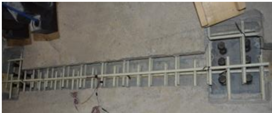
e) Photo of the closure strip for the A-joint before casting
