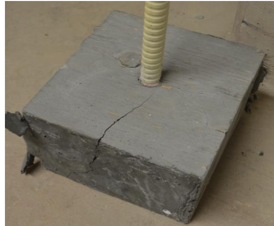
b) Concrete crack at top and side of the UHPC block after bar pullout
