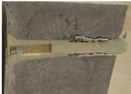
e. View of the GFRP bar with 60 mm concrete cover showing bar slippage from anchorage head
