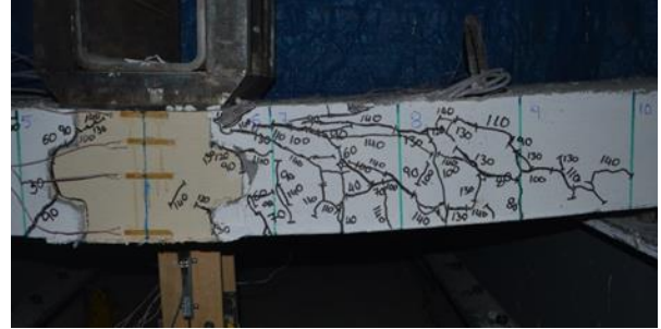
b) Crack pattern at joint region
