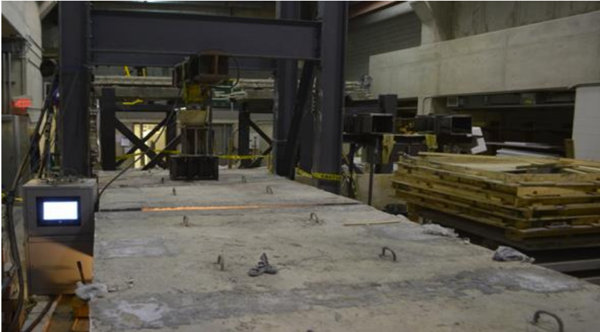
a) Slab-girder bridge system during monotonic loading
