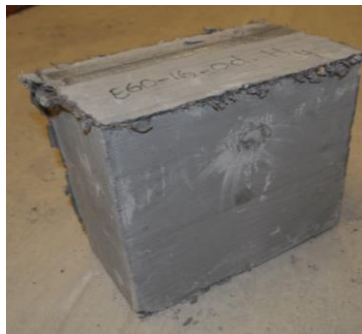
c. View of front and back face of block for GFRP headed bar with 40 mm concrete cover
