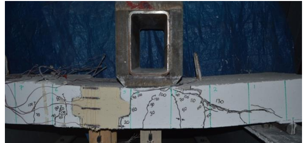
b) Close-up view of flexural-shear crack in precast slab
