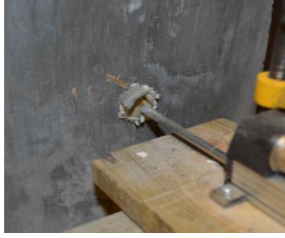
b) Block view at bar end slip
