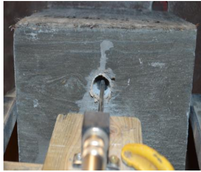
b. Bar projecting length disappeared inside the hole after test
