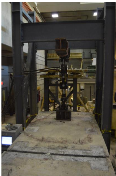
a) Slab-girder bridge system during CAF and VAF loading
