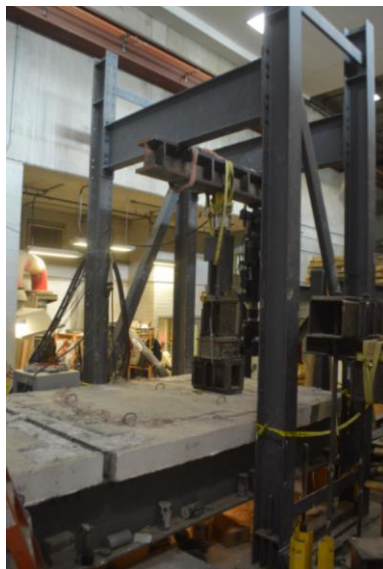
a) Slab-girder bridge system during monotonic loading
