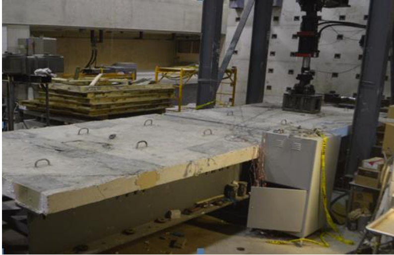
a) Slab-girder bridge system during CAF and VAF loading
