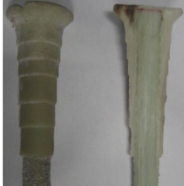
c) Sliced head-end, sand-coated, bar showing the grooves on bar surface filled with head material
