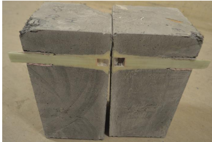
b. Section cut in the block with GFRP headed-end bar at 40 mm concrete cover showing bar slippage from head
