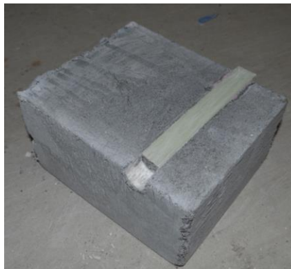
d. Close up view of section cut showing bar slip length at the free end
